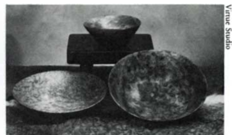
Some of Lory's bowls turned from locally available buris and stumps. Epoxy finish, which completely penetrates the ⅛-in. thick walls, makes the bowls flexible and durable.
