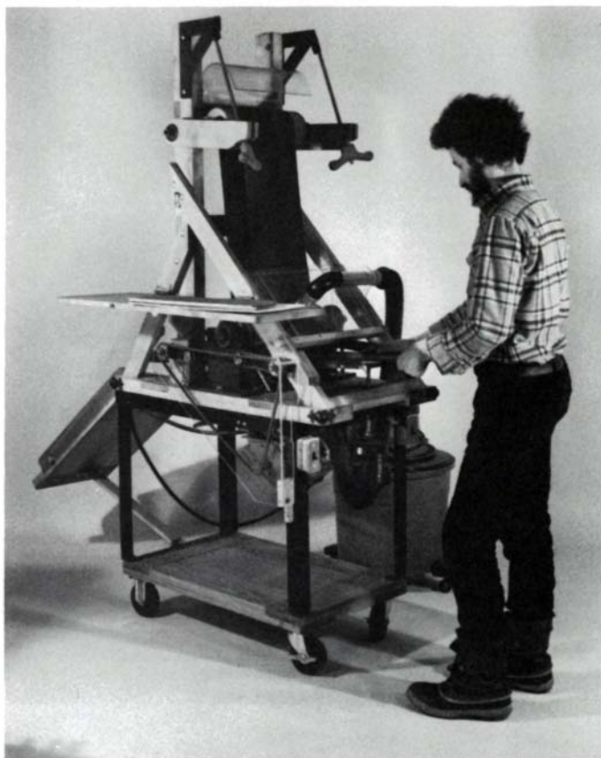
Left, stock thickened on abrasive planer, the thinnest pieces to 0.005 in. Below, Michael Horwitz at the 12-in. model.
