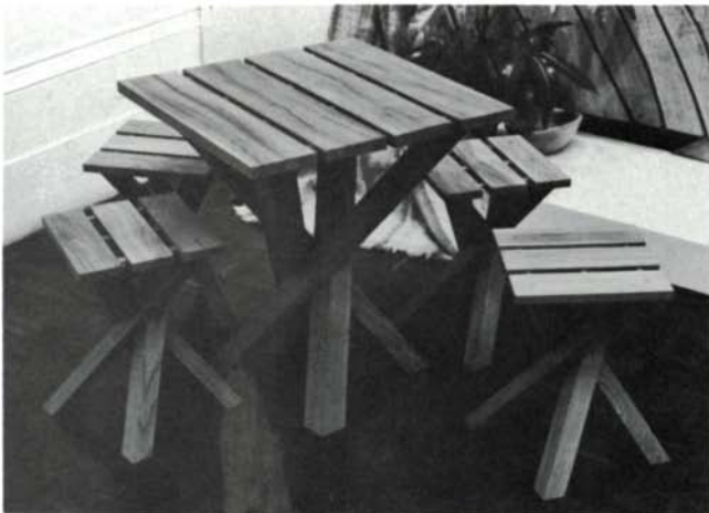
Ashley Cartwright's elm garden table and chairs welcomed visitors and set the tone for the first of the exhibition's three spacious rooms. The table, 25½ in. square and 28½ in. high, and the chairs, 13 in. square and 18 in. high, have four-board tops that are joined together by square-section pegs.
