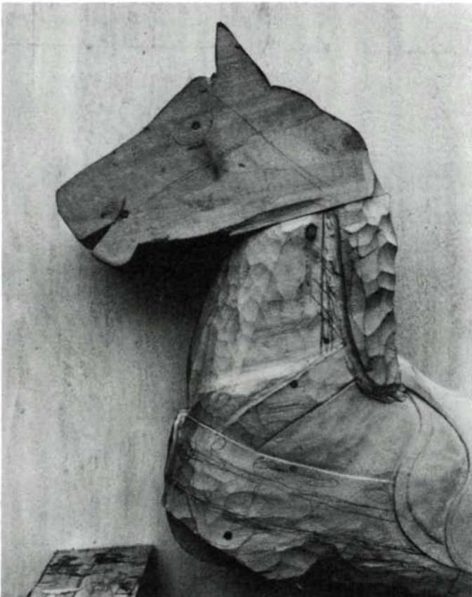
Head blank is tenoned and pegged into partially carved neck. Mortises for forelegs have already been cut in lower chest.
