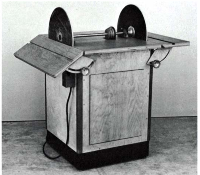
Bjorkman's 16-in. disc sander incorporates tilting tables and uses all four surfaces of the discs. Pulley guard removed for photo.
