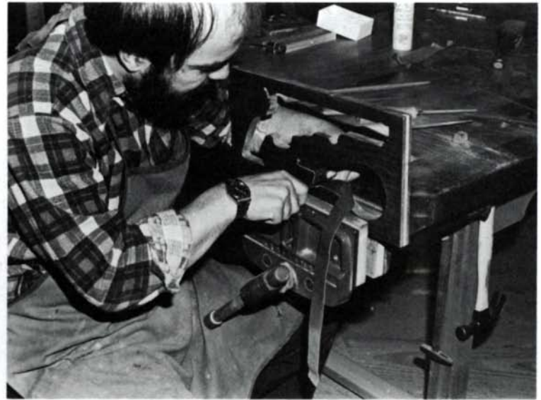
Leather is cemented into place. Note reinforcing spline in panel's edge.
