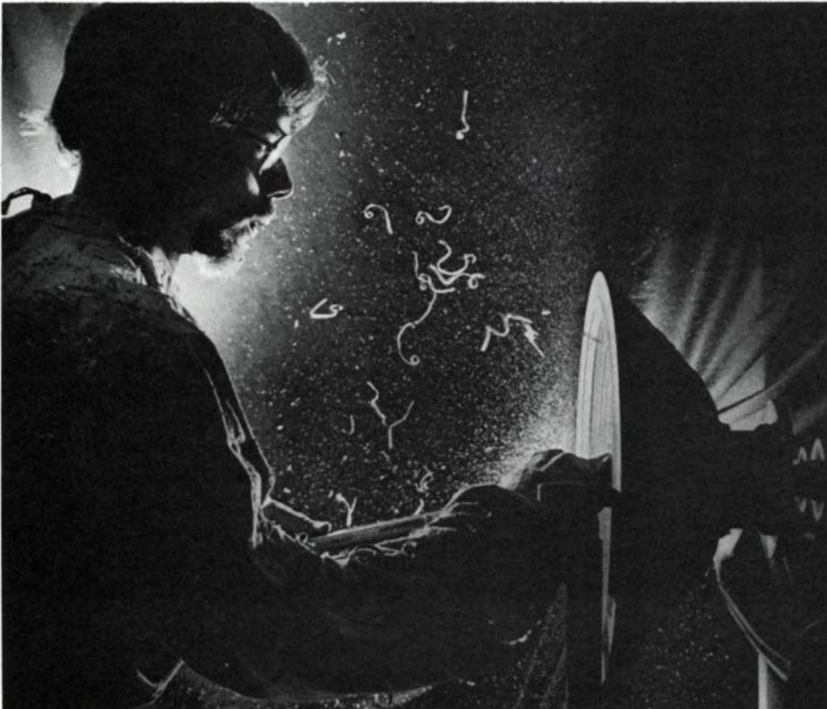
Using a steel-hafted chisel, Lory takes a cut off a rotating bowl blank. Tooling the alternating long and short-grain surfaces produces both shavings and dust.
