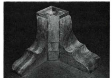
From the back, base frame (left) shows bare-faced mortise and tenon, and half-blind dovetails between back feet and braces. Segmenting the bracket-foot glue blocks (right) minimizes the chance that the bracket pieces, which run crossgrain, will crack.
