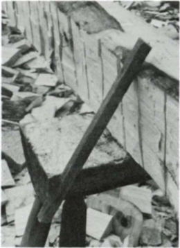
With both sides roughed out and rescored with a thin-bladed ax, log is steadied on trestles with 1x1 staples. Finish hewing can then begin.
