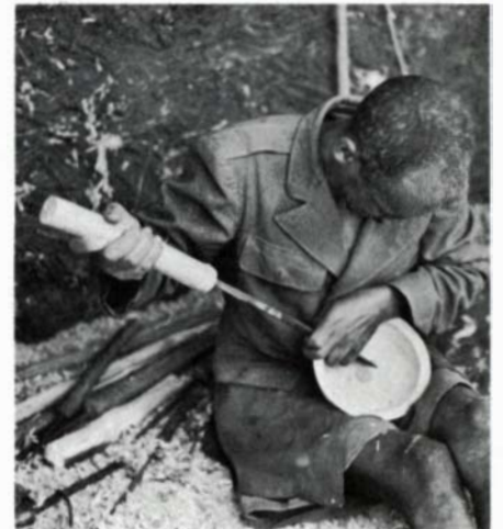
Rough areas are smoothed with a few strokes of the turning tool, and the bowl is done.
