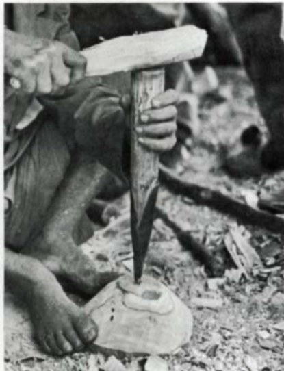
The headstock, a stick with a cone-shaped end wrapped in metal and square at the tip, is banged securely into the center hole with a mallet. Then he marks the tailstock center with a smaller drill.
