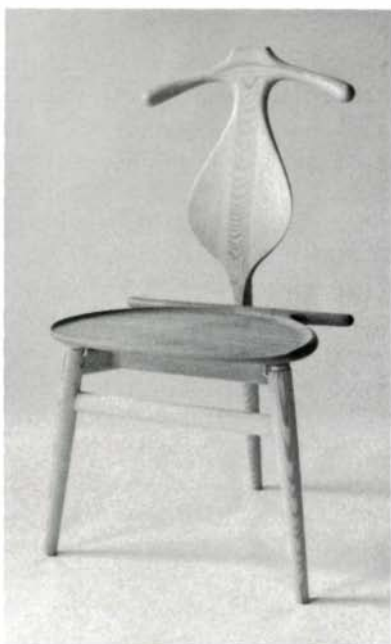
The valet chair demonstrates Wegner's inventive handling of a functional idea, in sculptural terms. The back member and legs are Oregon pine, with joinery and bold figure oriented to accentuate the hanger and backrest. A seat of teak lifts up to hold a folded pair of pants on its shaped edge, revealing a triangular tray for keys, watch and change. The late King Frederik IX of Denmark was the first purchaser of the valet chair, and was fond of presenting it as a gift. Right, a Wegner folding chair, a design often copied cheaply and common in import shops.
