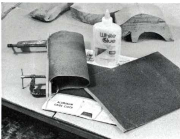
Sheets of cloth-backed sandpaper with a strip of sand removed and glued over on the back form sleeves for the sander.
