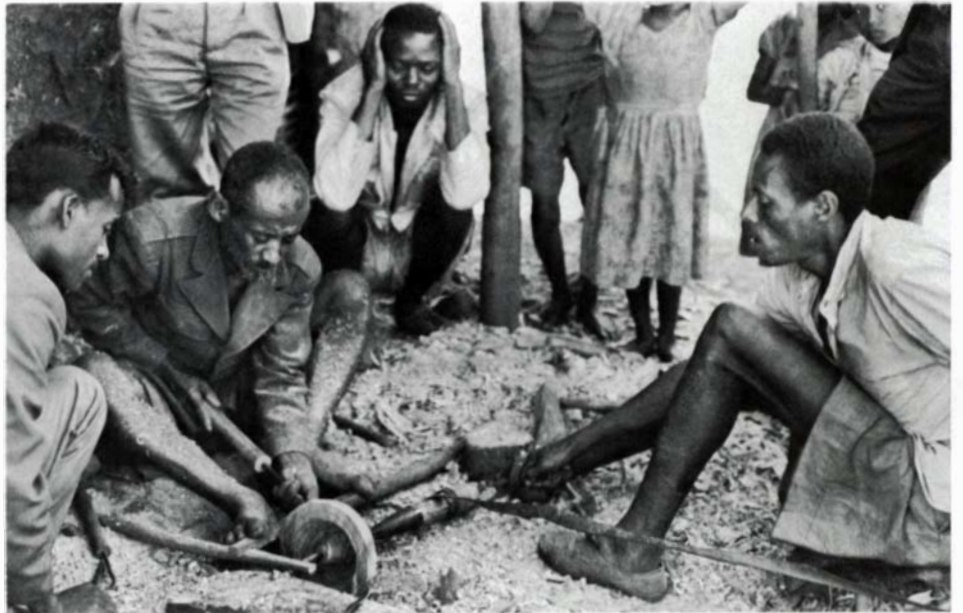
The lathe is powered by a strong assistant pulling forward and back on a long leather strap wrapped around the headstock. For symmetrical cutting, the strap must be pulled rhythmically.
