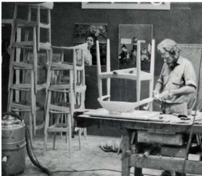
The Classic chair (also shown on the cover) is the epitome of Wegner's style. In some models the tapered finger joints between back and arms (cut on a shaper) are left exposed; in others they are wrapped with cane. The arm, left, is the original model that Wegner sawed a displeasing piece off, replaced and reshaped. The difference in grain between the two pieces indicates the graft. Below, a worker at Hansen's prepares to finish-sand a Classic Chair.
