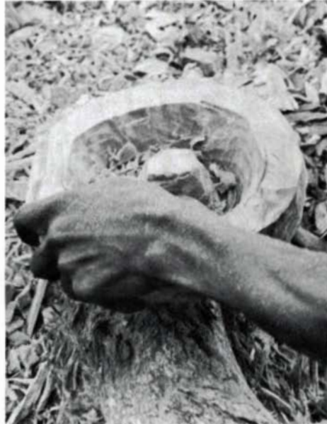
The next step is rough-shaping the inside of the bowl with a concave-bladed ax/adze. The knob in the center is left intact for attaching to the headstock of the lathe.
