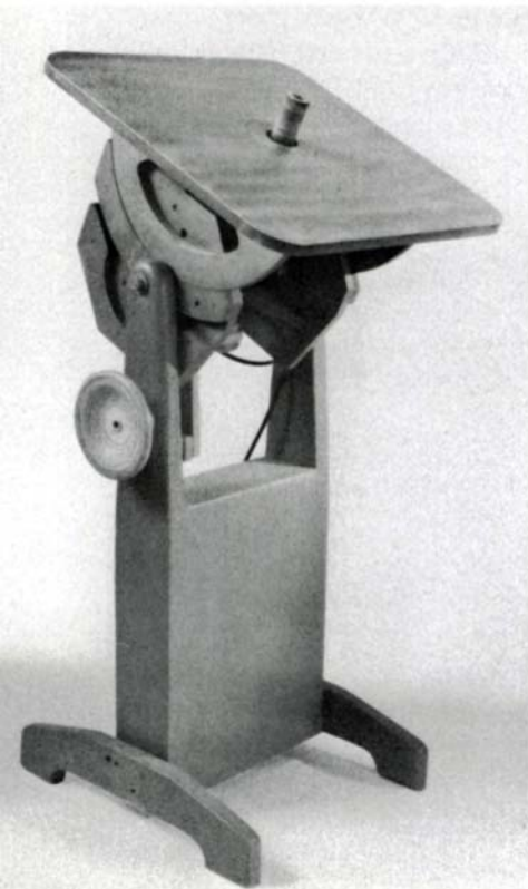
The drawing-board sander in spindle mode, left. The table, of aluminum-laminated MD-44, measures 24 in. by 24 in., and is 48 in. high when not tilted. The base consists of 2x6s covered with plywood, and the trunnions, fixed in position by tightening the four-pronged handwheel, are birch ply. Center, the table is removed, the large birch-ply handwheel loosened and the spindle positioned horizontally to receive foam-backed discs or drums. Self-aligning pillow blocks bear the shaft. Right, the 1/3-HP motor fitted with pulleys yields 2000 RPM and 550 RPM at the spindle.
