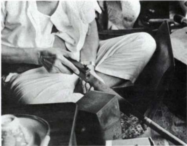
A special tool, left, joints the teeth. The saw vise alongside the sharpener's knee is used with a diamond-profile feather file, as at right, to sharpen the lead side of a rip tooth.
