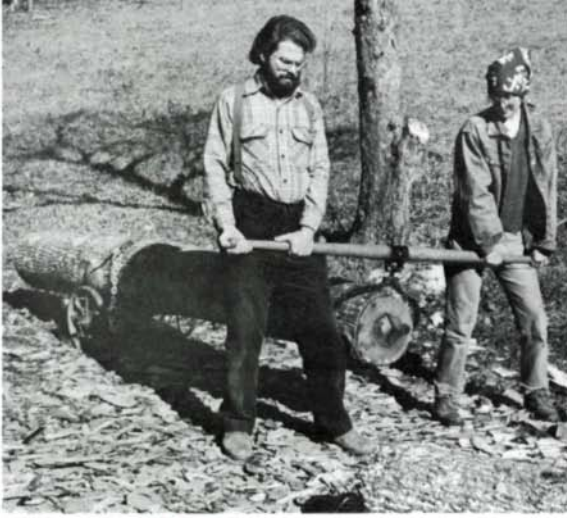
Two-person timber carrier and trolley, left, bring log to where it can be scored with a symmetrically beveled ax, hand saw or chain saw, center. Then log is rotated 30° and waste wood chopped with a symmetrically beveled ax to within 3/8 in. of the chalkline, right.
