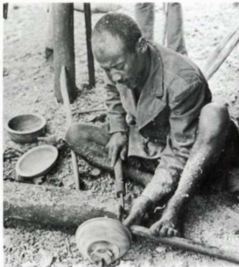
The headstock, a stick with a cone-shaped end wrapped in metal and square at the tip, is banged securely into the center hole with a mallet. Then he marks the tailstock center with a smaller drill.
