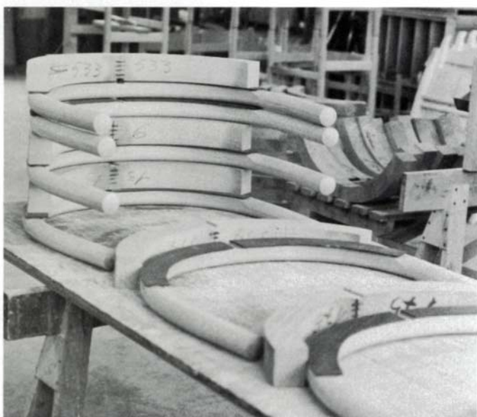
Bowed back of captain's chair consists of 15 pieces of ash, sliced, not sawn, from a single board and then glued back together on an electric form in their original order. In contrast to this technique, which conceals the laminations, Wegner uses wenge strips and splines to accentuate the joints between the other parts of the back.
