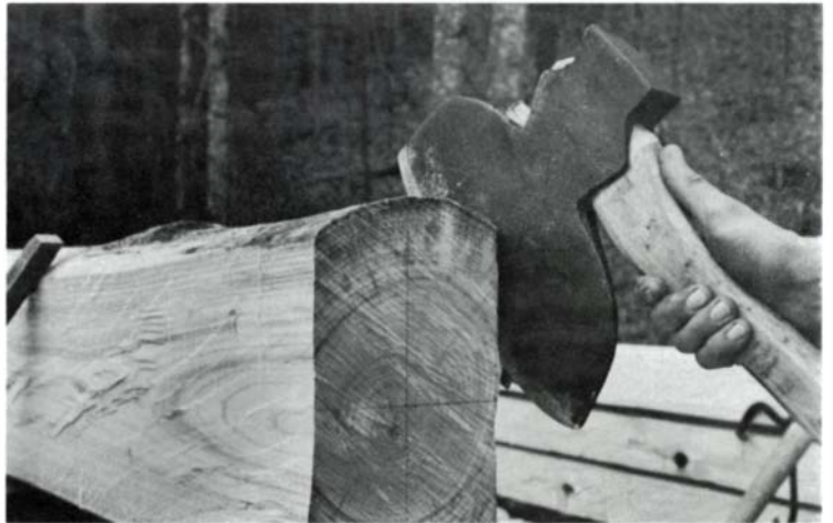
Broad ax, left and below, leaves a smooth surface in plane.
