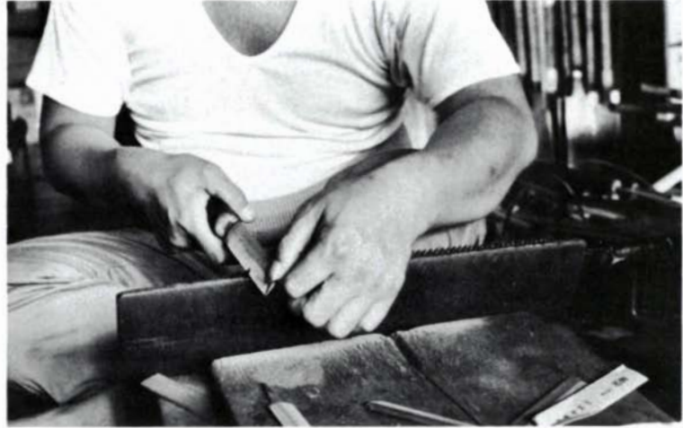
A special tool, left, joints the teeth. The saw vise alongside the sharpener's knee is used with a diamond-profile feather file, as at right, to sharpen the lead side of a rip tooth.
