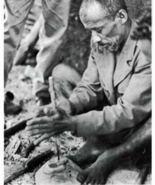
Next he drills a center hole in the bottom of the bowl—the drill is turned by rolling between the hands, while the Bowlmaker steadies the bowl with his feet.
