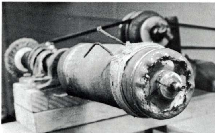
The drum, showing tire valve stem (sealed with silicone), wire wrap, canvas sleeve with drawstring, and pillow blocks bearing the belted shaft.
