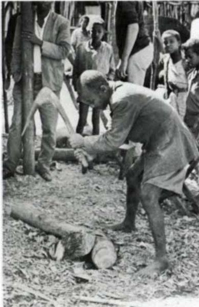
The Bowlmaker splits a large green log in half lengthwise with an ax/adze, then cuts it to length. Rounding the ends completes external shaping.
