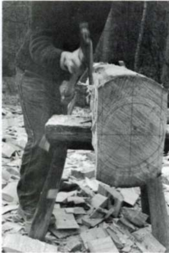
Two-person timber carrier and trolley, left, bring log to where it can be scored with a symmetrically beveled ax, hand saw or chain saw, center. Then log is rotated 30° and waste wood chopped with a symmetrically beveled ax to within 3/8 in. of the chalkline, right.
