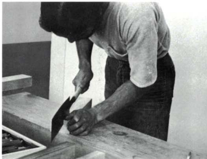
Imai lays out a lapped mortise and tenon scarf joint with a bamboo striking stick, which he dips at intervals into a chalk pot. At right, he cuts the mortise sides with a double-edged ryoba saw.
