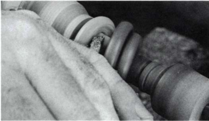
5. Use the same procedure to cut and free the rest of the rings; be sure to sand the surfaces before freeing each ring.
