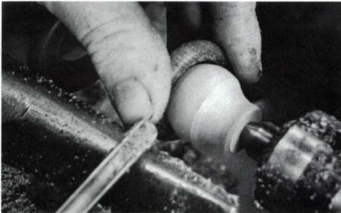
6. Shape the ball on the end of the rattle, leaving it just a little larger than the inside diameter of the first ring.
