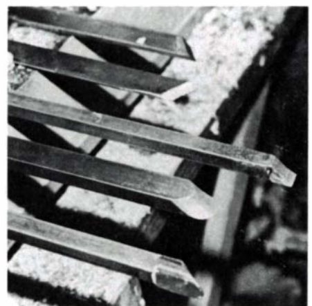
Grind step in cold-rolled steel bar and hack-saw notch.
