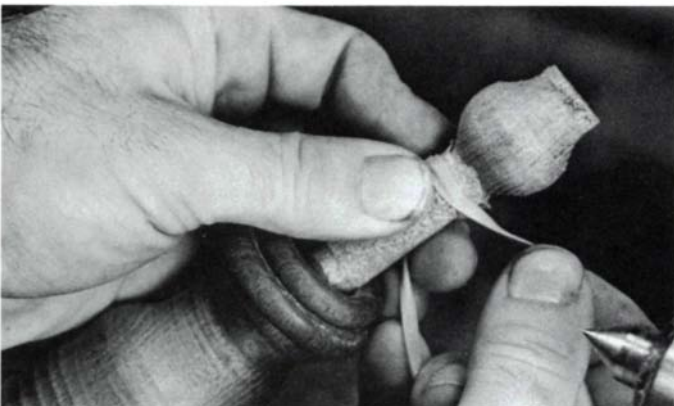
8. Wrap a strip of sandpaper around the shaft clockwise (so it doesn't unwind in use) and hold it in place with a rubber band. If the inner surfaces of the ring are ragged, start with 100-grit paper.
