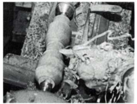
Top, tools made by Del Stubbs: two at top, ground from whole planer blades; second from bottom, ground from tool-steel bar; and the other two made more cheaply by epoxying planer steel bits to a length of ½ x ½ cold-rolled steel. Each of these tools has a deep hollow-ground bevel and is finely honed, as shown in the drawing. Above, the ½-in. roundnose at work.
