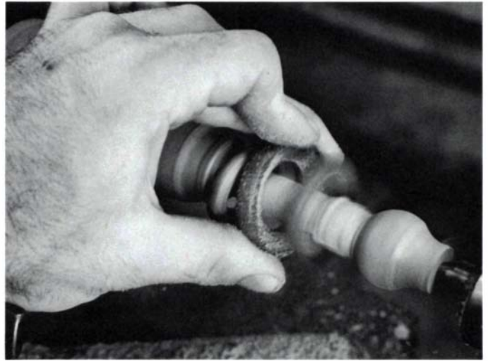
9. With the lathe running, hold each ring against the sandpaper. Move the ring to sand every section of the inside surface evenly, and tilt it to round the edges. I work up to 400-grit wet/dry paper wetted with mineral oil.
