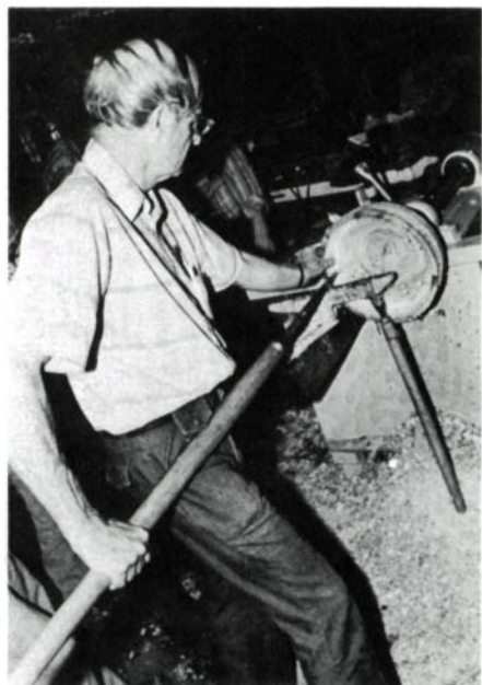
Top, Ed Moulthrop chats with Rude Osolnik. Moulthrop's work here is of tulipwood, the largest piece 36 in. in diameter. Above, Moulthrop checks thickness of turning bowl. His tool rest, attached to a 6x6 cherry beam and propped to the floor, steadies the 6-ft. long hook-bladed cutter he uses for inboard work. A 2½-HP motor turns the 3½-in. diameter spindle.
