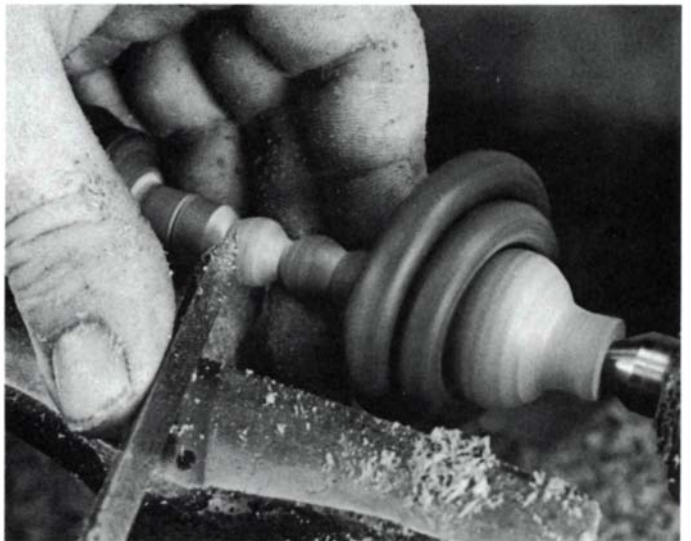
11. Use the toe of the skew or a beading tool to cut the beads. Shape the handle, then sand everything with wet/dry paper and mineral oil. Saw the waste off the ends, whittle them smooth, sand and oil. Warning: This rattle may be habit-forming. Don't leave it around unsupervised adults. □
