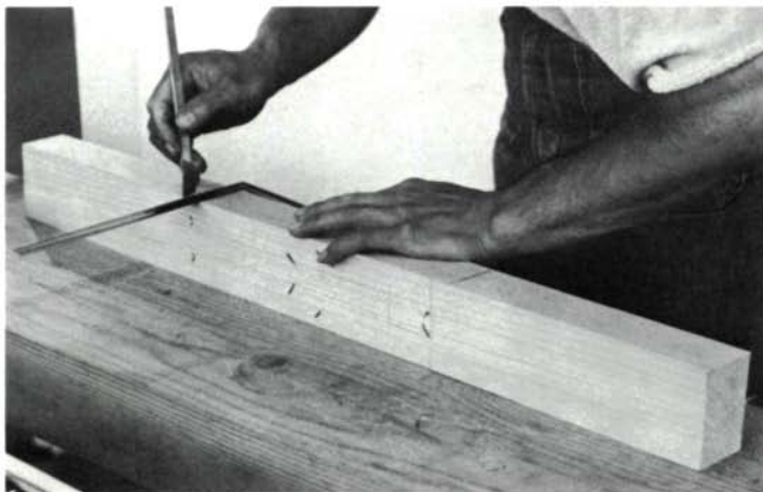
Imai lays out a lapped mortise and tenon scarf joint with a bamboo striking stick, which he dips at intervals into a chalk pot. At right, he cuts the mortise sides with a double-edged ryoba saw.
