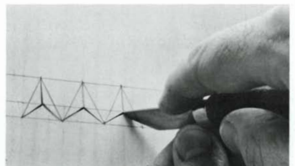
Make the three-cut chip by stabbing out the sides of the triangle with a skew-bladed knife, top left. Then carefully slice out the remaining wood with a straight-edged knife, left. Above, some traditional dreischnitt border designs.
