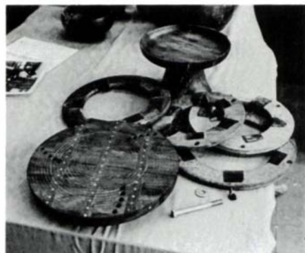
Jack Straka's faceplate assembly with various plywood rings and a finished bowl, whose 6-in. high pedestal is hollow.
