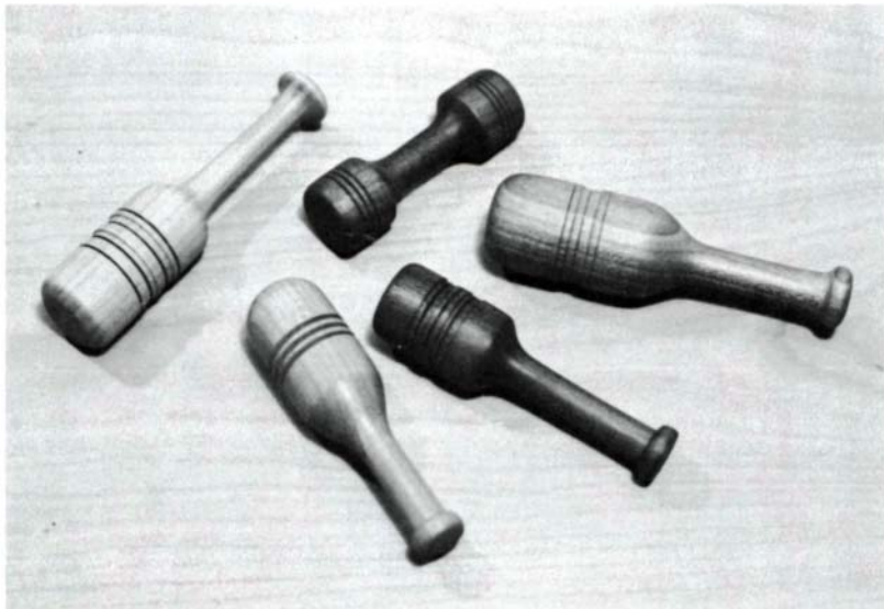
Rattles are assembled from a crosscut block and a wooden sleeve made by drilling a dowel. Kernels of corn rattle inside the cavity, and the dowel walls provide long-grain surface for gluing. Marks on reglued block, right, show where to avoid turning into the dowel.
