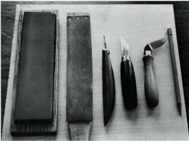
Left, chip-carving tools include a sharpening stone and leather strop for bringing knives to a razor edge, a straight-edged knife for making slice cuts, a skew-bladed knife for stab cuts, and an offset blade. The wood blank is pine, though any soft, even-grained wood will do. Top, a burr is left by sharpening on the stone; subsequent stropping leaves the edge razor-sharp, above.
