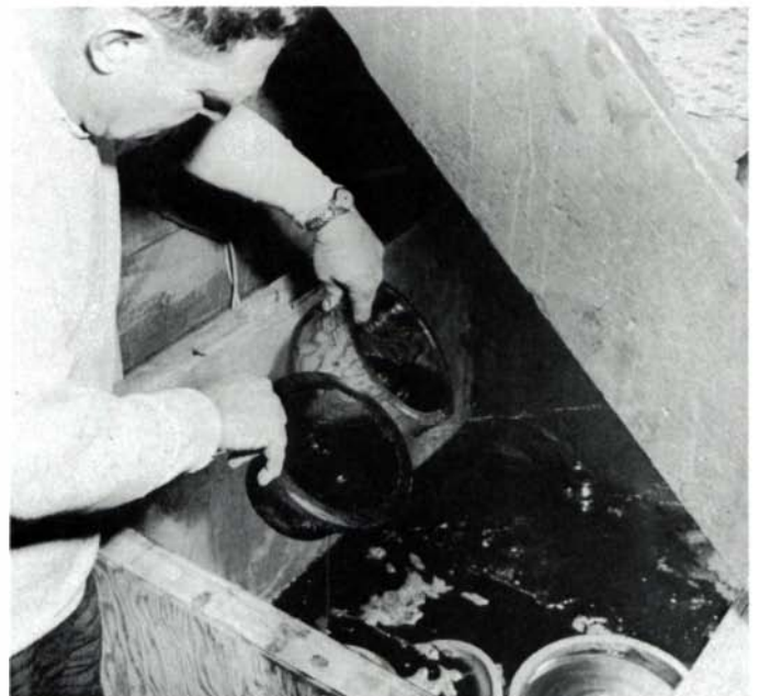
Bowls are removed from a PEG soaking vat—a plywood box lined with fiberglass.
