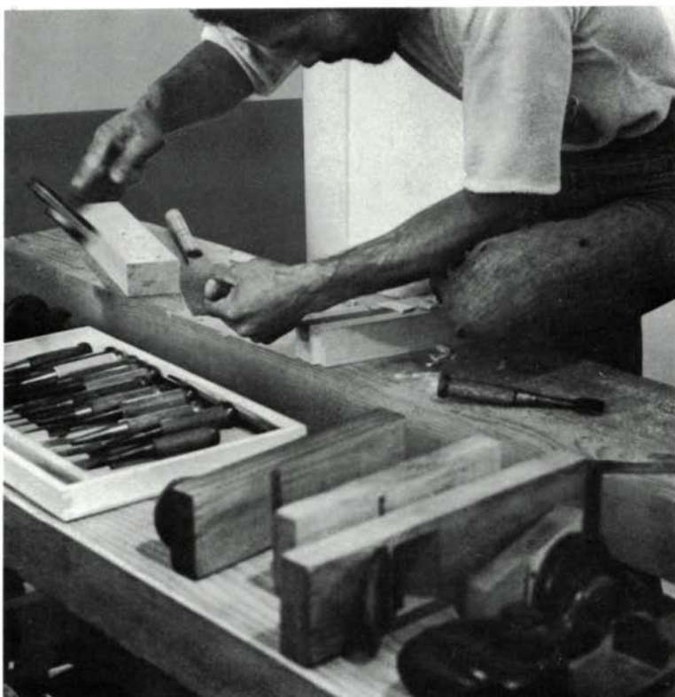
Using only his leg as a clamp, Imai chisels the mortise waste, above. His bench consists of two fir planks on trestle horses: one plank for work, the other for tools. At right, the lock-key half-cuts are chiseled in the sides of the tenon.
