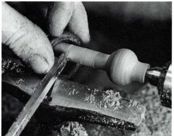
10. This is a good time to rough out the shape of the handle. Then trim the shaft to its finished diameter and lay out the beads with deep marks cut with the point of the 1/4-in. skew.
