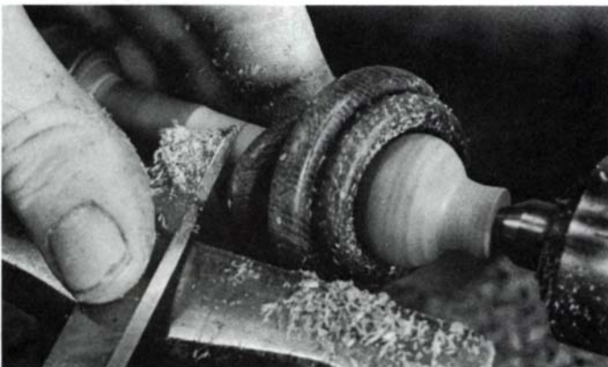
7. Use a 1/2-in. skew to trim the shaft to a smooth cylinder, but leave the diameter of the shaft as large as possible at this stage. Hold the rings away from the tool with your finger.
