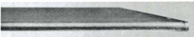
Traditional parting tool leaves rough surface and splintered corners because the side of the tool scrapes rather than cuts the wood.
