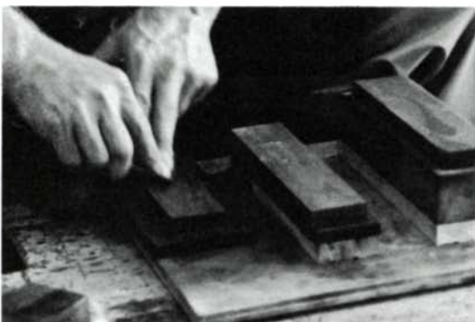
Klausz's three stones are mounted on one board, stepped from coarse to fine to provide clearance for the handle of the chisel or the held end of the plane iron.
