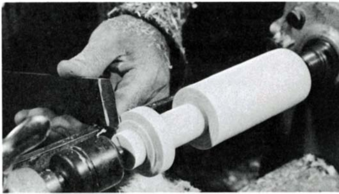
Cleaning up a rough parting cut with a skew chisel. Begin with handle down and over to the right so the left-hand bevel will be in contact with the cut surface. Slowly raise the handle, arcing the point into the work, to slice a thin section. Do not move the bevel away from the cut surface or end the cut with the handle higher than parallel to the floor; the tool is liable to kick.
