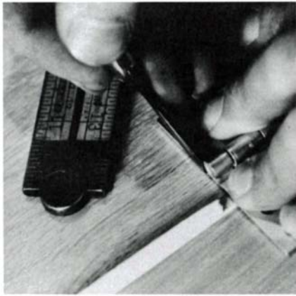
Fitting the hinges is an exacting task. Scribe and chisel the hinge recess, then the hollow for the hinge knuckle.
