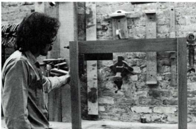
Lay out and cut leg-apron mortises while the stock is still square.
