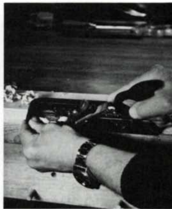
A series of passes with the rabbet plane wastes the bulk of the curve. The open side of this plane allows the iron to cut right to the shoulder of the fillet. At right is an end view of the roughed curve.
