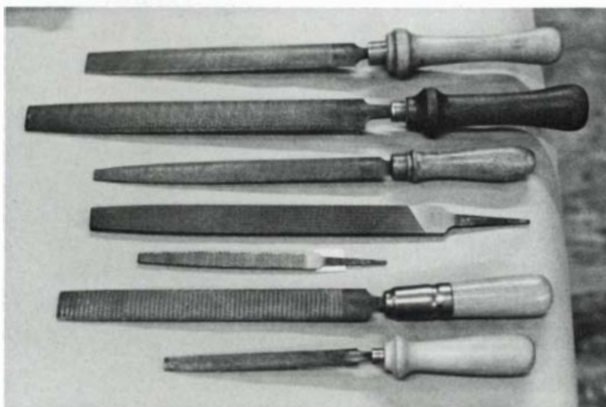
Rasps and files are better than edge tools for shaping complex curves, where the wood grain runs in several directions.
