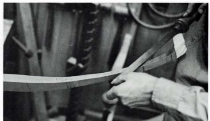
Rasps and files are better than edge tools for shaping complex curves, where the wood grain runs in several directions.
