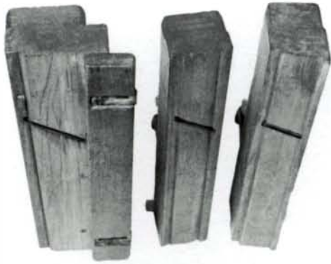
Three panel-raising planes, circa 1800. Left, raising jack made by J. Butler of Philadelphia, has adjustable fence and depth stops, and nicker cutter ahead of skewed iron. This prevents tear-out when working across the grain. Plane at center was made by A. Smith of Rehoboth, Mass.; right was made by S. Kimball. All three planes are 14 in. long, and range from 2 1/8 in. wide to 3 1/4 in. wide.
