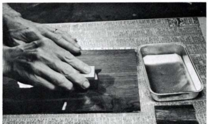
To rub out specks and imperfections, lightly stroke abrasive paper that has been wetted with mineral spirits across the surface in the direction of the grain.
