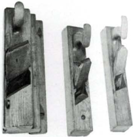
Three panel-raising planes, circa 1800. Left, raising jack made by J. Butler of Philadelphia, has adjustable fence and depth stops, and nicker cutter ahead of skewed iron. This prevents tear-out when working across the grain. Plane at center was made by A. Smith of Rehoboth, Mass.; right was made by S. Kimball. All three planes are 14 in. long, and range from 2 1/8 in. wide to 3 1/4 in. wide.
