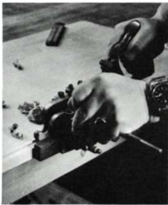
Wallace uses his grandfather's Stanley 45 to remove the fillet from the tabletop, left. A rabbet plane works just as well. At right, the fillet is cut to just shy of the scribed line.
