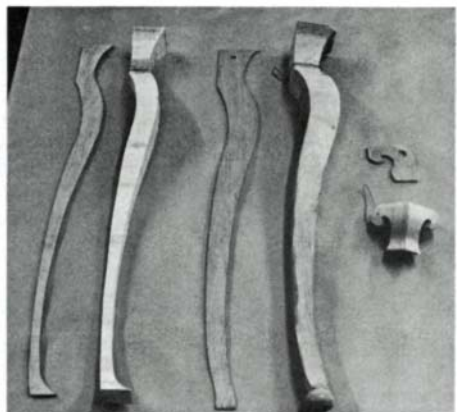
Trace the leg template on two adjacent sides of the blank, flipping it over so the knees meet at a corner. Bandsaw from one tracing, then tape the scrap back to the block to bandsaw side two. Three pattern legs, all in scrap stock, and the templates from which they were cut are shown below.
