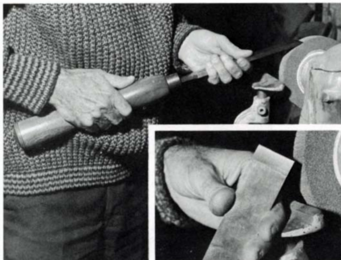
Child sharpens his chisels on top of the grindstone without using the tool rest. He determines the proper angle by eye and maintains it with a light grip, elbows held close to the body. With the ‘woodturner’s sway,’ he moves the chisel back and forth across the stone.
