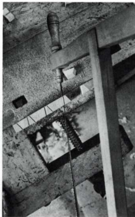
Left, Klausz saws the pin sides. He does not lay these out beforehand, but judges angle and spacing by eye, using the steps detailed at top left. Above, Klausz saws pin-board waste with the dovetail cutout saw. Its bent blade turns horizontally in the vertical kerf, then splits the gauged line that marks the bottom of the tail sockets.
