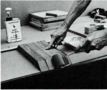
1. Buttering mitered ends with epoxy glue.
