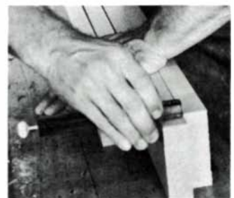
Lay all four aprons on bench, square across for shoulder lines, then gauge mortise width on each apron.
