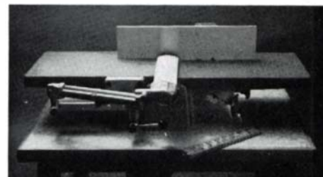
8 5/8" Jointer with thickness planing ability
