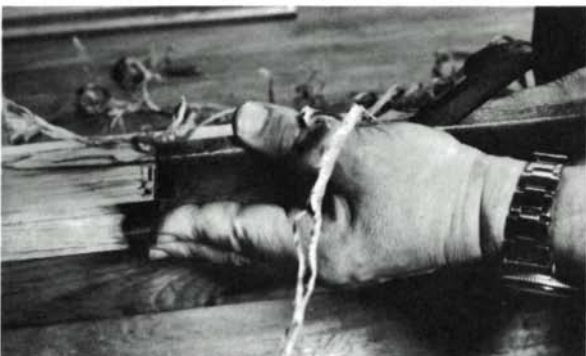
When cleaning up to the line, work the first groove into the chamfer by using your fingers as a fence.
