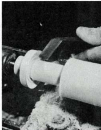
Variations on the right-angle cut: curved taper (planing with square-nose chisel), left, and saucer cut (arcing in with skew chisel), right. In each case the bevel follows in contact with the cut surface.
