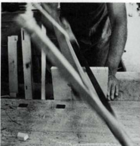
Left, Klausz saws the pin sides. He does not lay these out beforehand, but judges angle and spacing by eye, using the steps detailed at top left. Above, Klausz saws pin-board waste with the dovetail cutout saw. Its bent blade turns horizontally in the vertical kerf, then splits the gauged line that marks the bottom of the tail sockets.
