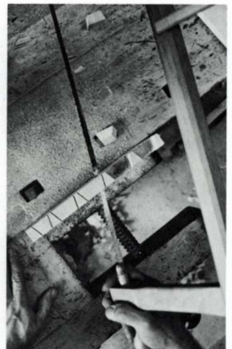
Left, Klausz saws the pin sides. He does not lay these out beforehand, but judges angle and spacing by eye, using the steps detailed at top left. Above, Klausz saws pin-board waste with the dovetail cutout saw. Its bent blade turns horizontally in the vertical kerf, then splits the gauged line that marks the bottom of the tail sockets.
