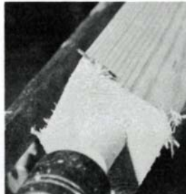
Traditional parting tool leaves rough surface and splintered corners because the side of the tool scrapes rather than cuts the wood.
