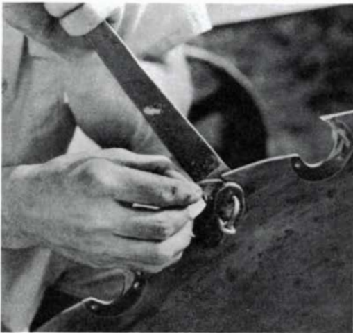
Tooth wrench (left) removes and installs teeth and holders. Swage (above) has two slots: convex-faced for forming points and flat-faced for shaping cutting edge. It is struck (right) with short, sharp blows.
