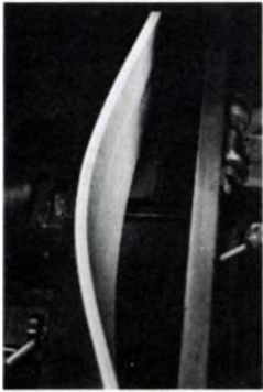
Use the bending form base as a jig to trim drawer fronts to width. The curve can often be freehanded over the jointer.
