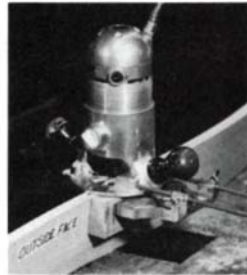
Use the bending form base as a jig to trim drawer fronts to width. The curve can often be freehanded over the jointer.
