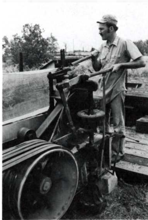
The plate-feedworks, above, is the ideal transmission. Right-hand lever moves feed plate in and out to start and stop carriage; left-hand lever moves friction wheel up and down to control carriage speed and direction.
