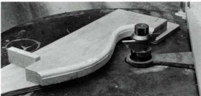
First and final cuts, as cutter is lowered into work over several passes. Notice that the jig contour is set back from stock contour because
