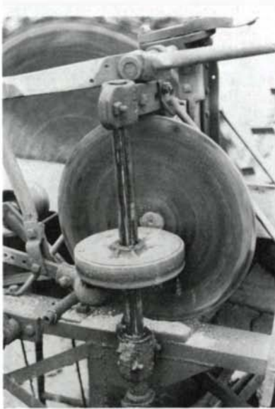
The plate-feedworks, above, is the ideal transmission. Right-hand lever moves feed plate in and out to start and stop carriage; left-hand lever moves friction wheel up and down to control carriage speed and direction.
