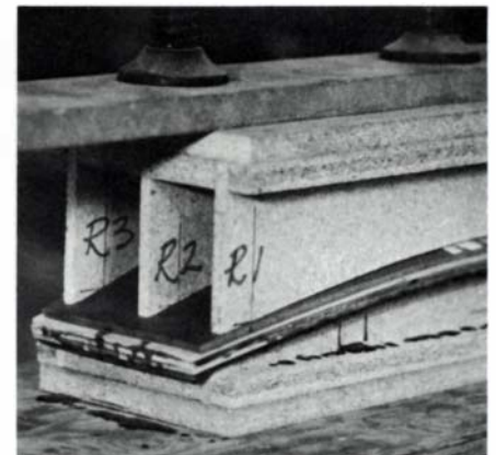
Full-size shop drawing (left) and resulting press-form ribs for drawer-front sections R1, R2 and R3. The press form (center) with ribs in place. These ribs are removable, so the same base pieces can be used with the ribs for the other drawers in the carcass. One section of a veneer press is used to bend the drawer-front laminates (right). The wood and the form are separated by a layer of Masonite to distribute the pressure.
