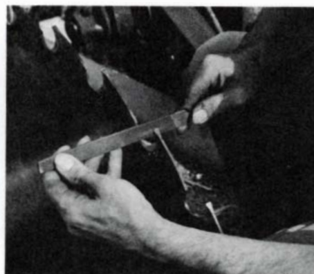
After swaging, sharpen the tooth by first dressing the sides with a bastard file supported by the plate (left). Then file straight across the face of the tooth (above) at the correct angle (right). One light stroke on the back of the tooth removes any burr.
