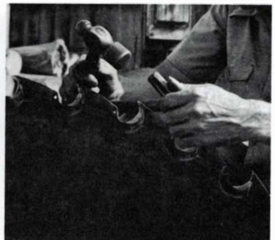
Tooth wrench (left) removes and installs teeth and holders. Swage (above) has two slots: convex-faced for forming points and flat-faced for shaping cutting edge. It is struck (right) with short, sharp blows.
