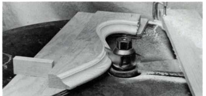
ring collar extends past shallowest part of cut. The guard has been removed for photograph.
