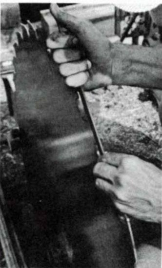
After swaging, sharpen the tooth by first dressing the sides with a bastard file supported by the plate (left). Then file straight across the face of the tooth (above) at the correct angle (right). One light stroke on the back of the tooth removes any burr.
