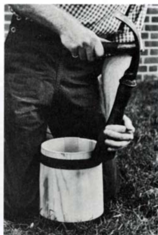
A hoop driver and hand adze are used to tighten the hoops and clamp the staves.
