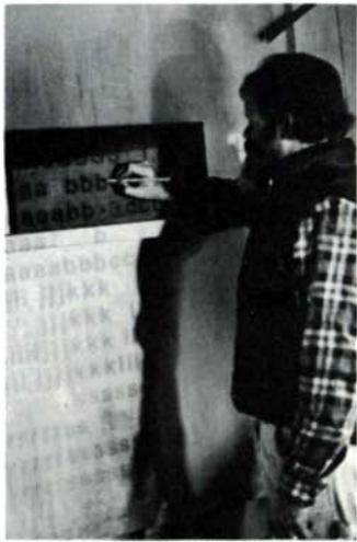
Left, Wilbur traces image cast by overhead projector directly onto the wood, then routs out sample letters, above. The heels of the hands rest firmly on the wood to guide the router through each letter. Some of his finished signs are shown at right.
