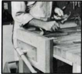
1 "Flip-over" vises provide a solid workstop—yet turn over so top of vise is flush with bench surface for regular vise use.
