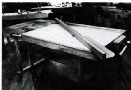
Best of simple router tables, left, is a square of Masonite inlaid into a large, flat work surface, under which a router motor is hung. Fence is clamped to edge of table and supported at the bit by scrap board. Chips escape through opening in fence. Center, router table clamps into the three vise openings of a Scandinavian-style workbench, and was the genesis of Kunkel's convenient, 'sublime' table, which clamps almost anywhere. Right, underside of table. Block in upper right-hand corner strengthens stud bolt on which fence pivots.
