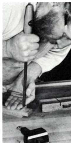
Place the workpiece on a bench hook and cut the shoulders with a tenon saw, leaving about 1/16 in. for paring with a wide chisel or shoulder plane.
