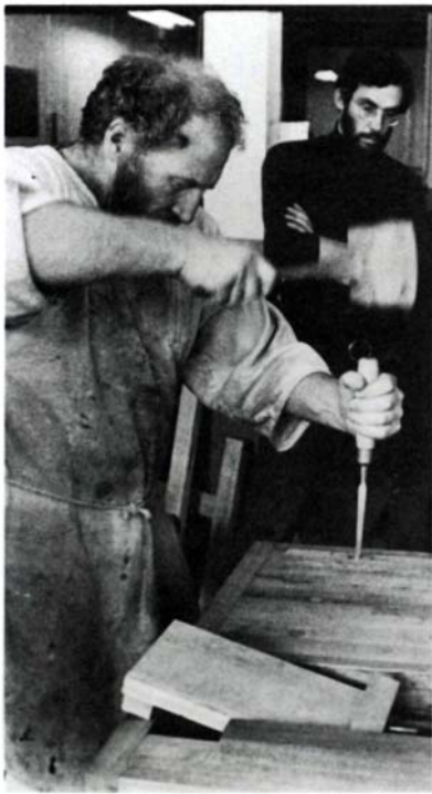
Align the chisel with the center of your body, strike it hard, and then lever out the waste.
