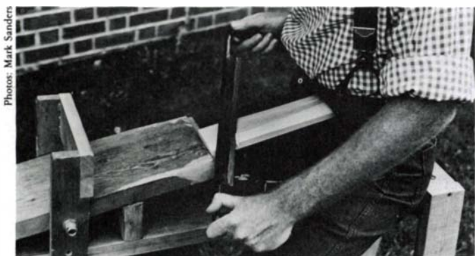
A drawknife rounds the outer surface of the stave. If working the stave in both directions chips the grain, hold the stave between a notch in the shaving horse and your stomach.
