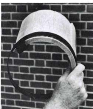
Each added stave is pushed towards the clip. Because the outsides of the staves are wider than the insides, they won't fall in.
