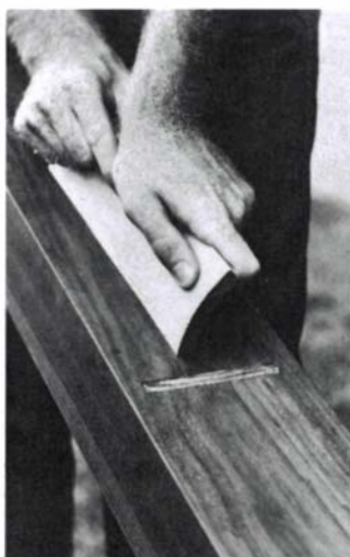
When jointing stave edges, determine the bevel by eye.
