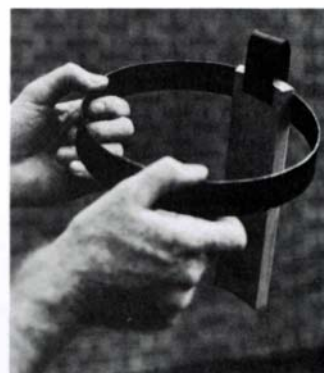
The first stave clipped to the hoop with a scrap of hoop is a template for the other staves.
