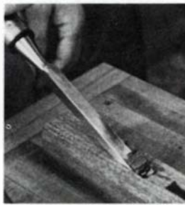
Align the chisel with the center of your body, strike it hard, and then lever out the waste.
