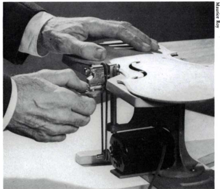
Wake's purfling machine cuts a narrow channel a round edge of violin plate.
