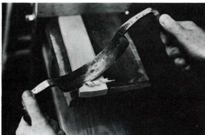
A hollow knife cuts the concave surface on the inside of the stave.
