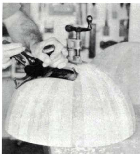
Whittle a plug to fill the hole, then bore a clean 2-in. hole at each pole to receive turned plugs. The hemispheres are shaped with a compass plane and Surform, then a rabbet is routed at the equator.
