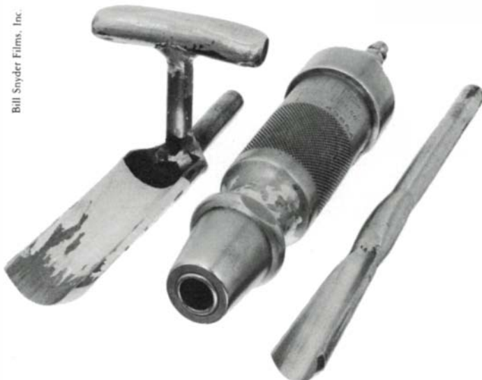
The pneumatic carving gouge is a stonecarver's reciprocating air hammer (center) that accepts a standard 1/2-in. shank. Right, 3/4-in. #11 sweep has been cut down at the handle flange so a length of 1/2-in. steel rod could be welded on. The steep-sided #11 enters and leaves the wood easily, without becoming buried, but carvers' preferences vary. The large gouge at left has an added T-bar for better control. Top photo: the author demonstrates the use of the pneumatic gouge to an audience of sculptors.
