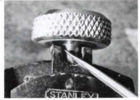
It's usually necessary to modify the adjustment mechanism to eliminate slop. Offsetting the fingers on the horizontal-screw block plane (left), bending the top finger downward to the nut on the vertical-screw block plane (center), and bending a finger rearward on large horizontal-screw planes (right) help eliminate play. The mechanisms of larger planes are similar to the ones shown here.
