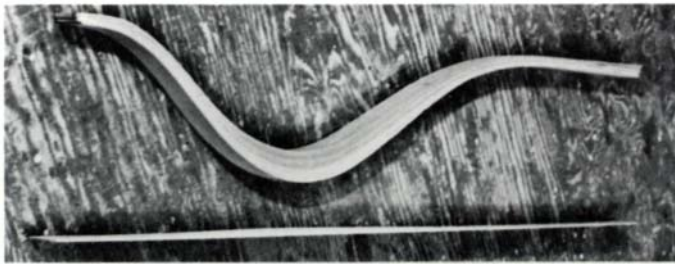
Double-tapered lamination (top) and one of its components.
