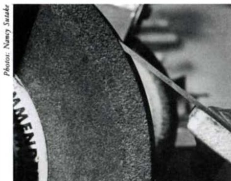
A properly set tool rest supports the blade and fixes its proper angle to the stone.
