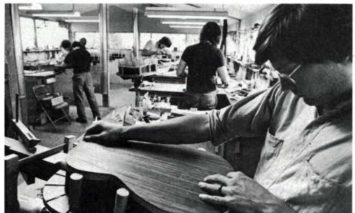
Morris checks alignment and fit on a guitar back, while students work on their projects.
