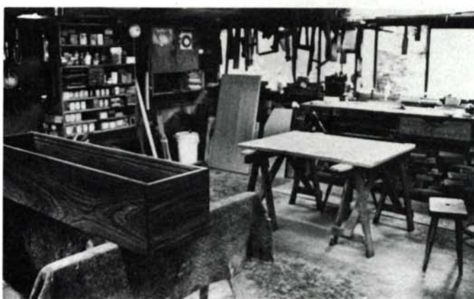
Machine room, top, has three table saws, two thickness planers (one 32 in. wide) and two jointers (one 24 in. wide), two band saws, a lathe, a drum sander and a stroke sander. In the adjoining bench room, above, is a rosewood carcass (foreground) that will become a horizontal wall-mounted cabinet with sliding doors, a special commission. The corner joint is a through dovetail (inset) with mitered ends, an attractive detail that also hides the through-plowed door grooves. The usual shop practice is to cut the tail angles first, using a tilt-arbor saw, rout the waste almost to the line and finish with chisels. Then the pins are scribed and cut with a fine Japanese saw. The miters are left a little fat, the joint is closed as far as it will go, and the saw is run through the miter to create a perfect fit.
