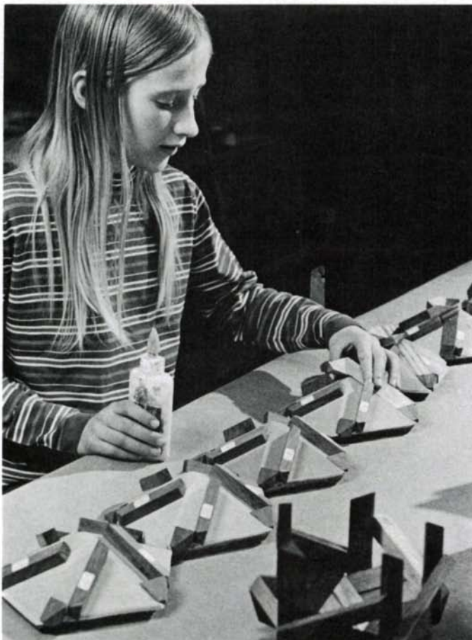
The 60 individual sticks that make up the puzzle shown above are assembled on a set of 12 precise gluing jigs. The original pentahedral base for the jigs was made on a milling machine, then duplicated by
