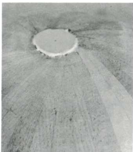
Whittle a plug to fill the hole, then bore a clean 2-in. hole at each pole to receive turned plugs. The hemispheres are shaped with a compass plane and Surform, then a rabbet is routed at the equator.
