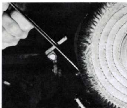
To buff, pass each edge over the wheel several times with moderate pressure.
