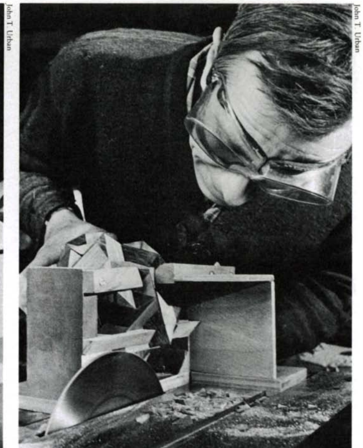
casting in Hydrastone. After the yellow glue has set, the puzzle is assembled, and the ends of the sticks are trimmed flush on the table saw, using a jig that slides in the miter-gauge slot.
