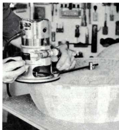
Whittle a plug to fill the hole, then bore a clean 2-in. hole at each pole to receive turned plugs. The hemispheres are shaped with a compass plane and Surform, then a rabbet is routed at the equator.
