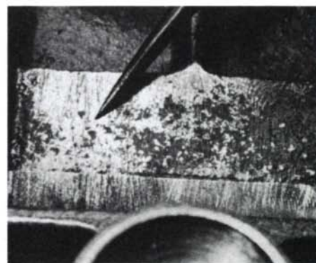
This blade, adjusted parallel to the sole (left), is angled because of an out-of-square support surface. To remedy, remove metal from the high side of the support surface (right).
