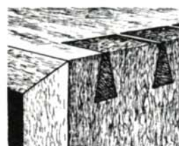
Machine room, top, has three table saws, two thickness planers (one 32 in. wide) and two jointers (one 24 in. wide), two band saws, a lathe, a drum sander and a stroke sander. In the adjoining bench room, above, is a rosewood carcass (foreground) that will become a horizontal wall-mounted cabinet with sliding doors, a special commission. The corner joint is a through dovetail (inset) with mitered ends, an attractive detail that also hides the through-plowed door grooves. The usual shop practice is to cut the tail angles first, using a tilt-arbor saw, rout the waste almost to the line and finish with chisels. Then the pins are scribed and cut with a fine Japanese saw. The miters are left a little fat, the joint is closed as far as it will go, and the saw is run through the miter to create a perfect fit.
