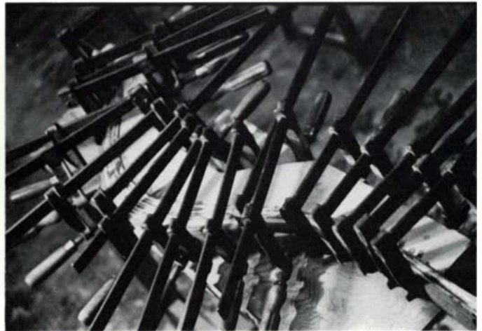
Double-tapered laminates are clamped to a one-piece form.
