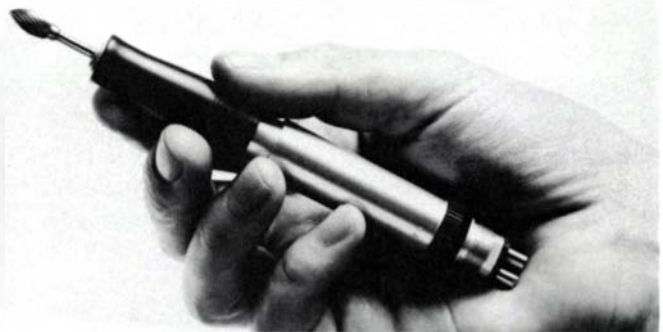
Dental laboratory handpiece, at 25,000 rpm, does the same job as the more common flexible-shaft grinder but is less tiring to control. A slightly larger tool, the industrial pencil grinder, runs at 50,000 rpm. Users of flexible-shaft tools know that small high-speed steel burs aren't very durable. Dental supply firms sell carbide burs, which last much longer, for about $3 each.
