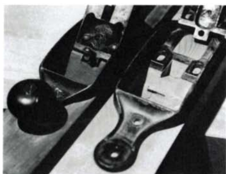
Old plane (left) and old mechanism with a new block. Note the relief for the metal boss at base of frog.
