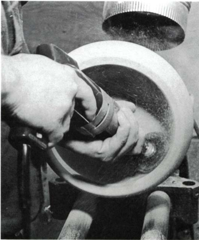
The bowl interior is ground smooth with a disc attached to an electric drill. A suction system located above the bowl removes the clouds of dust that lathe-sanding creates.
