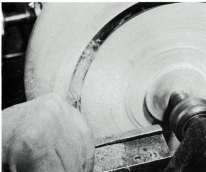
Cone separation: Above, a cut twice the thickness of the file divides the center cone from the bowl. After subsequent cuts have roughed out the interior of the bowl, the cone can be freed with a spoon gouge and mallet, below. A few sharp whacks of the mallet, with the cutting edge of the chisel facing end grain, will do the trick. The cone can later be made into another, smaller bowl.
