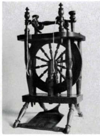
early 19th-century chair wheel has two wheels connected by a drive band, for high speed. Double treadle and pitman permit precise starts and stops without hand propelling.
