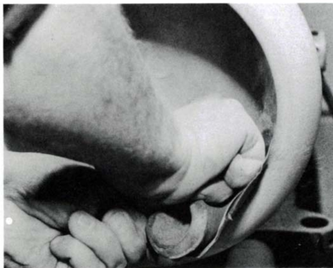
The bowl is finish-sanded in increasingly finer grits, with a \frac{1}{2} -in. foam-rubber pad held behind the sandpaper.
