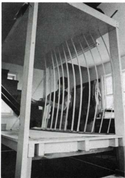
Springy oak 'go-bars' braced against stationary upper deck hold down work placed on movable lower deck. Jig provides uniform pressure for gluing complex shapes.
