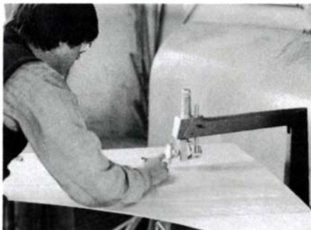
A precisely crafted soundboard is critical to the tone of the instrument. Here, the soundboard is carefully measured with a "poor man's caliper," a dial indicator attached to a jigsaw. Then the soundboard will be planed to the proper thickness.
