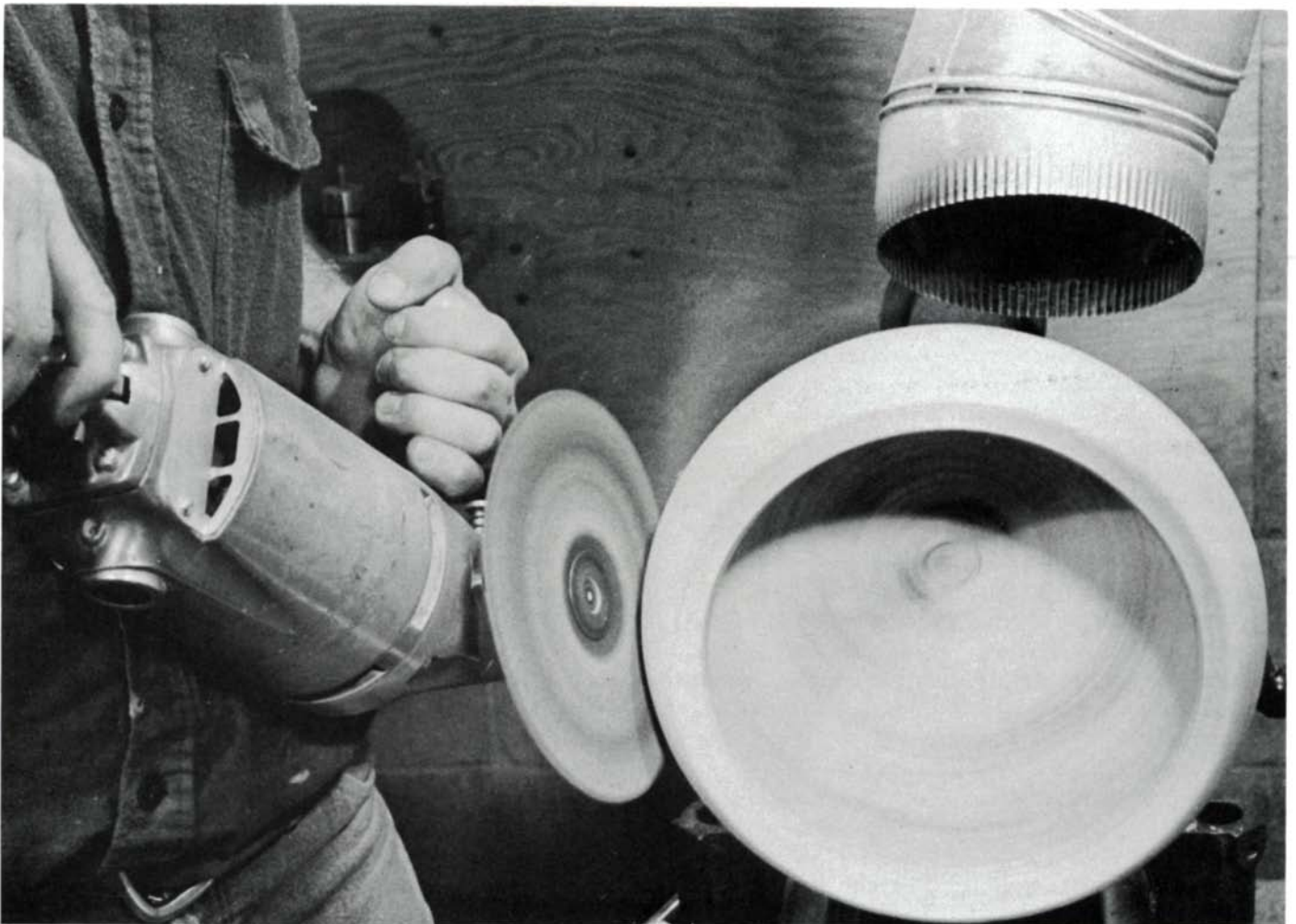
Author rests body grinder on hip and pushes it from headstock to lip to sand bowl exterior.
