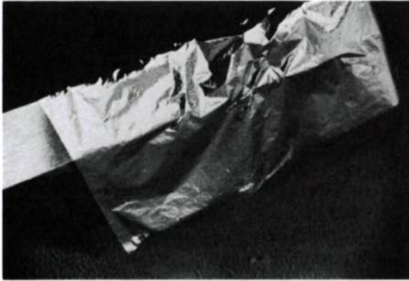
Special gold knife, lightly dusted with fine pumice, lifts sheet of genuine gold leaf. Beware of imitation gold, which tarnishes within months.
