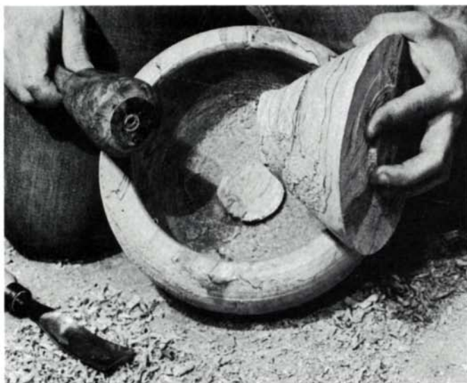
Cone separation: Above, a cut twice the thickness of the file divides the center cone from the bowl. After subsequent cuts have roughed out the interior of the bowl, the cone can be freed with a spoon gouge and mallet, below. A few sharp whacks of the mallet, with the cutting edge of the chisel facing end grain, will do the trick. The cone can later be made into another, smaller bowl.
