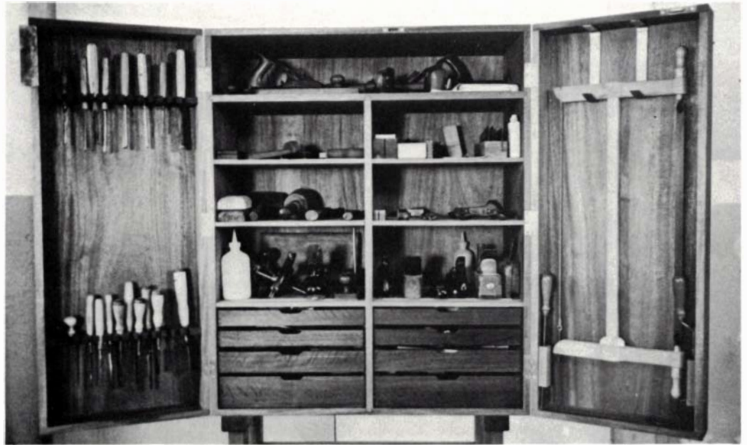
John Dunnigan's tool cabinet (41 in. by 34 in. by 19 in.; base is 24 in. high) is solid mahogany, with plywood door panels veneered in fiddleback mahogany. The inside of the door is 3 1/4 in. deep. One door holds saws; the other has adjustable shelves with holes and slots for screwdrivers and carving tools. The shelves are 14 in. deep and adjustable in height.
