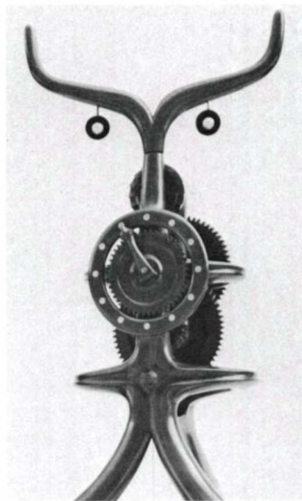
'Clock III' by Lawrence Hunter uses a verge-and-foliot escapement. The horns atop the clock swivel majestically back and forth, taking two seconds each way, releasing a tooth of escape wheel each time. Wheel has 15 contrate teeth—that is, teeth are parallel to arbor rather than perpendicular to it.
