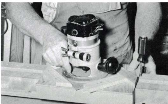
Spangler routs a slot; screwdriver indexes carriage.
