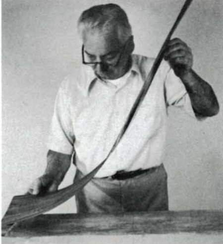
Lay veneer face down in glue. The glue that smears on it will help hammer slide easily.
