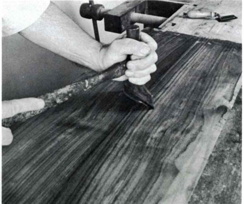
With both sheets stuck and the seam trimmed, reheat with the iron and push hard with the hammer to squeeze the excess glue out through the line of the joint.
