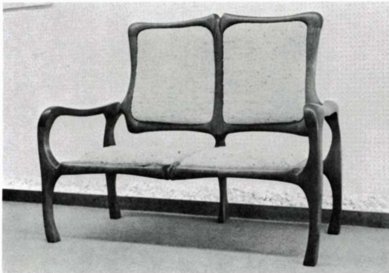
Settee by Kenneth A. Lange of Port Chester, N.Y. (cherry with Indian tweed upholstery, 50 in. long, 43 in. high, 27 in. deep), shown at Westlake Gallery in September. Lange begins with square stock, cuts the blind mortise-and-tenon joints, then bandsaws each piece to its general outline before assembly. Then he rasps, files and carves the final form.
