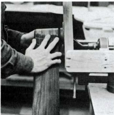
Waist-first bending: Mark at center of blank, where waist will be, ensures sufficient length for upper and lower bouts.
