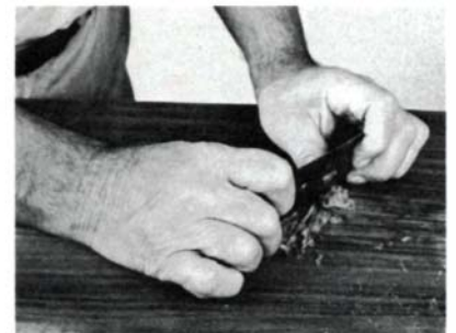
Block and clamp hold curly spot down while glue cools; strip of heavy paper along seam keeps it closed until glue dries. Then a sharp scraper cleans off paper and glue.
