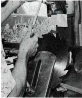
All the spurs in a group on a dado blade, left, are alike. In blade blank above, right gullet is typical, left is correct.
