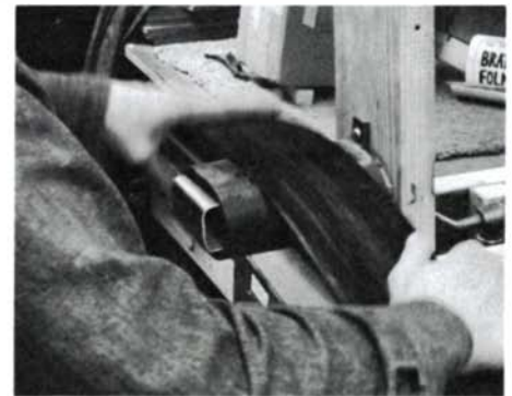
Right hand feeds evenly while the left fans rapidly (note blur) to advance the blank in small hops across the pipe.
