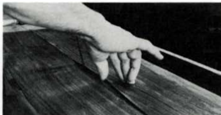
Saw through both veneers at once, carefully lift top sheet and peel away scrap beneath.
