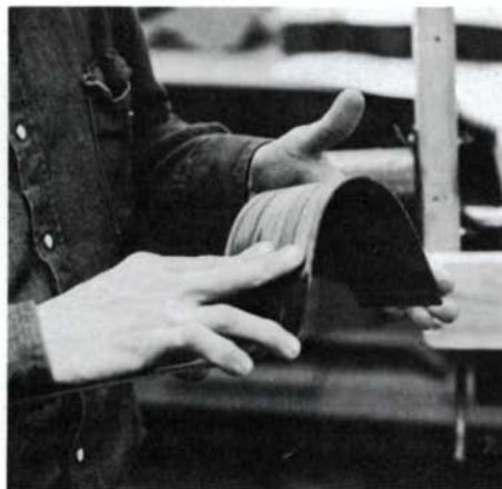
Neck-to-tail bending: Major curve section of upper bout is held in tension momentarily to permit wood to “cure” in new shape.
