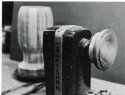
5. Cylinder is removed from lathe and replaced by stock for base. Author usually turns a rabbet so base will plug in snugly.
