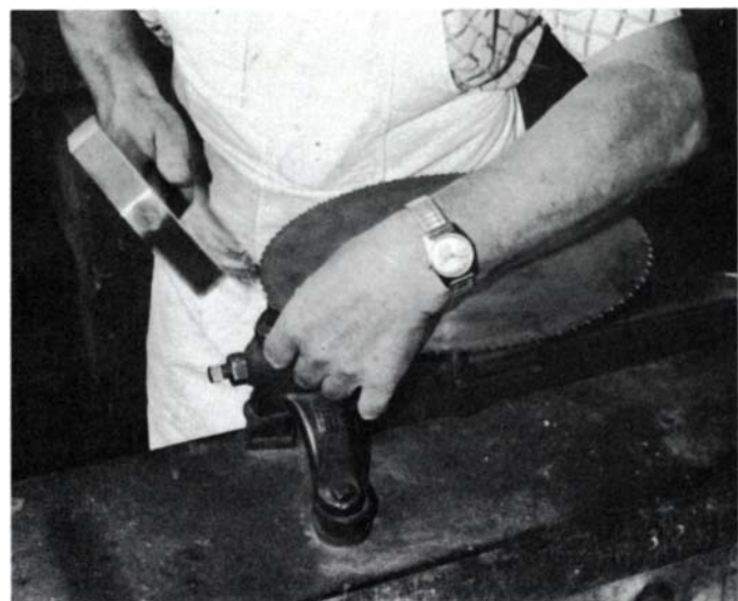
With anvil and stake, one sharp tap per tooth sets the saw.
