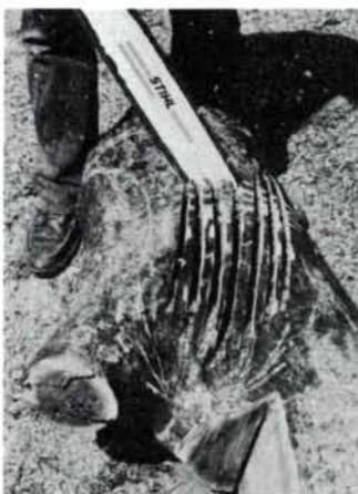
From tree to finished form: Above, Werner begins with a promising walnut trunk that includes the stump of a branch. First he chalks the lines on the log and slices away the waste. Convex forms are refined and smoothed by scraping lightly back and forth with the edge of the saw bar. Deep pockets are formed with the nose of the saw by tracing a cross-hatch pattern and breaking away the waste. Top right shows the sculpture as shaped by the chain saw. Right, 'Two-Hooded Form' has been dried, finish-carved and sanded (66 in. high).
