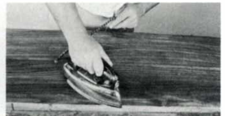
A hot iron remelts the glue in a troublesome spot. Then go over it with the hammer.
