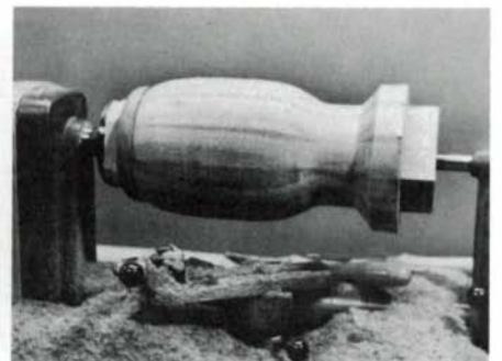
6. Tailstock feed applies pressure for gluing cylinder to its base.
