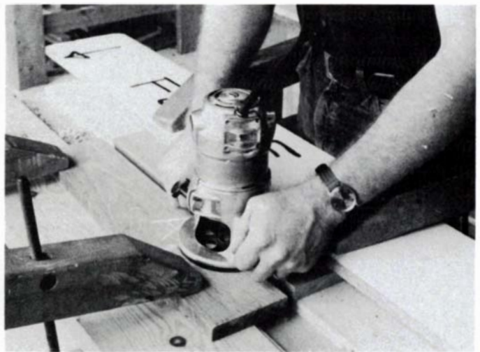
Operator guides router along fence from his left to right to cut 1/16 in. from second piece of wood.
