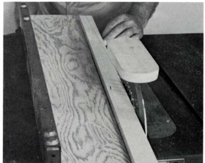
Ripping the taper: Jig guarantees four identical slides.
