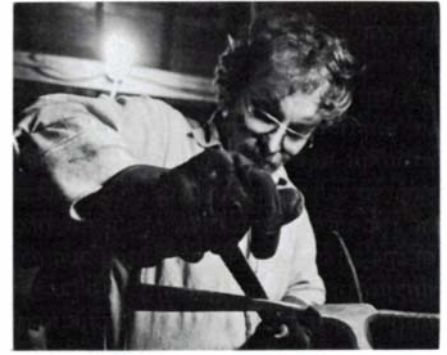
Author files weld on shell auger.
