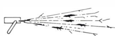
Low-carbon steel: Streamers thrown from wheel are straight, light straw in color. Some small amount of sparking.
