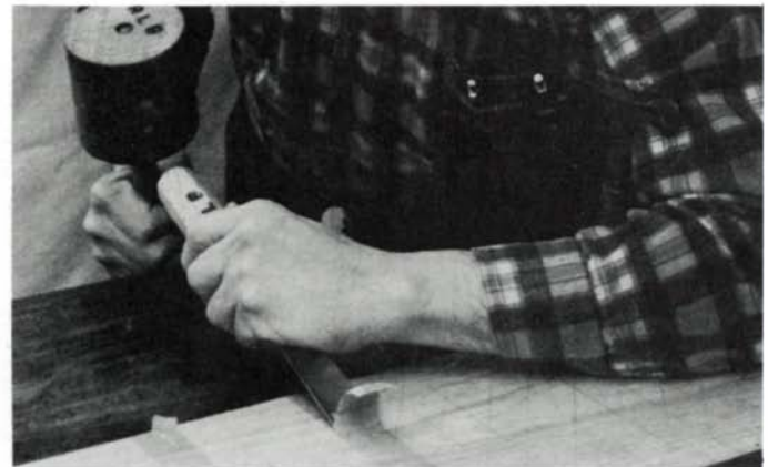
Mallet powers gouge; guiding hand holds center of tool and pivots from elbow.
