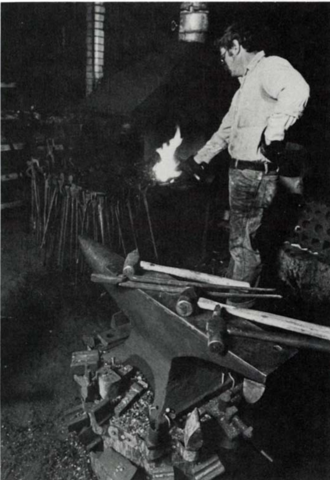
Author at work. Note rack of tongs by the forge and hardies mounted in slips around base of anvil, a 350-lb. Hay Budden.
