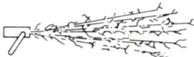
High-speed tool steel: Similar to high-carbon steel but with fine explosions. Reddish streamers. No sparking around wheel.
