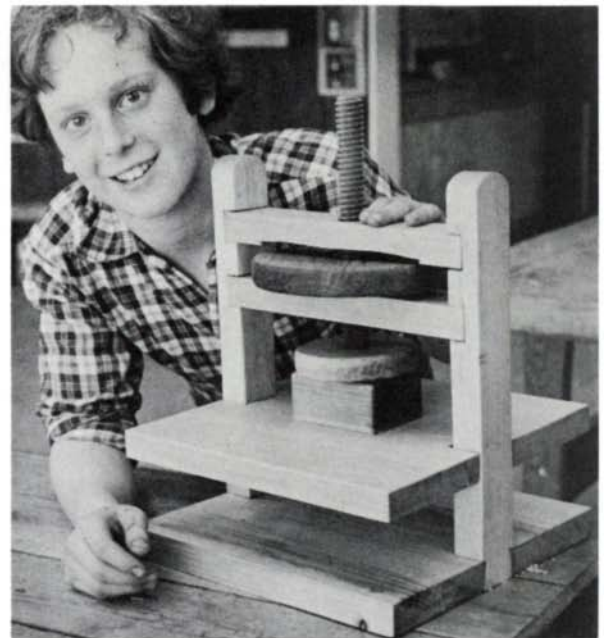
'It's a press. You turn the large round wheel to make the board go up and down.' —Adam Tucker, 7th grade.
