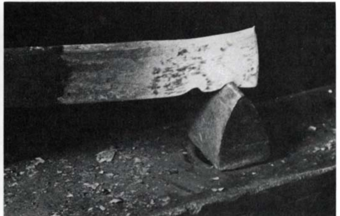
Below, fuller in hardie hole of anvil speeds drawing down steel. Bottom, swage block gives steel round or gouge-like shape.
