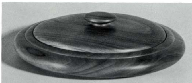
Horizontal-grain box in cherry, 10 in. diameter, 2-1/4 in. high, shows design possibilities permitted by the method diagrammed above. Lid is mostly finished with tailstock for support, then taped in place for final shaping of knob.
