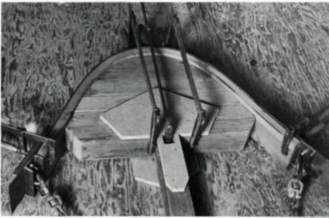
Bend is complete. Enormous compressive forces are apparent in slight curve away from mold's ends, despite heavy reverse levers.
