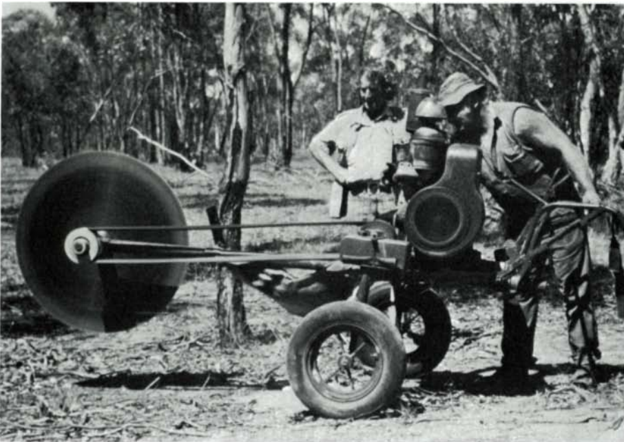
Tools and techniques for milling logs where they fall are ingenious and varied. Above left, Granberg's Mini-Mill chain-saw attachment for vertical cutting (about $50); right, Granberg's two-man Alaskan mill ($350 to $450, depending on size; chain saws not included). Left, Australian machine for cutting eucalyptus logs into railroad ties. The operator straddles the log and steers the whirling blade through the wood, with one wheel on either side of the log. Very few of these tie-cutters still exist; their use is now prohibited for obvious safety reasons. Below left, wedge-splitting slabs off a large chunk. Below right, pit sawing in Honduran forest: two-man teams rip logs into boards to transport to market. Top man raises saw and follows cutting line; bottom man powers downward cut and gets face full of sawdust.
