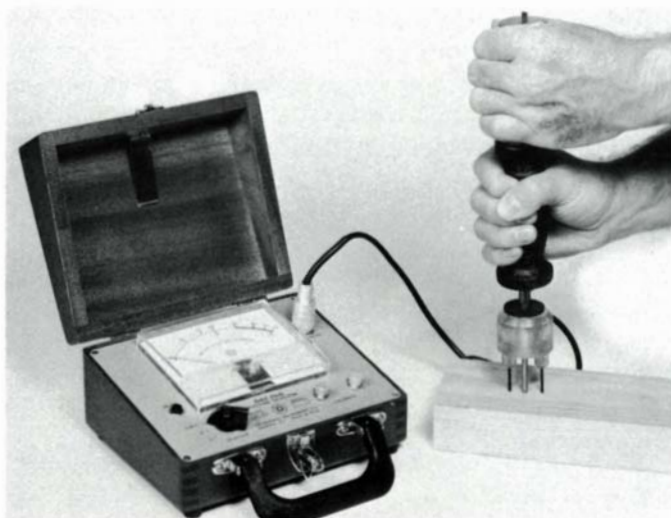
Pin electrodes of resistance meter are pushed into board, parallel to grain. Center pin gauges penetration.
