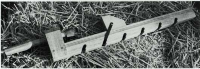
Screws of C-clamp, top, and bar clamp are slanted to allow for flex.
