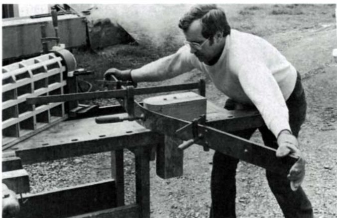
Wood fits tightly against strap between solid steel end blocks, which extend outward from small clamps to provide leverage. Then assembly is clamped to center of mold to prevent initial buckling and quickly pulled around. After setting for 15 minutes, wood is clamped overnight to drying jig, left.
