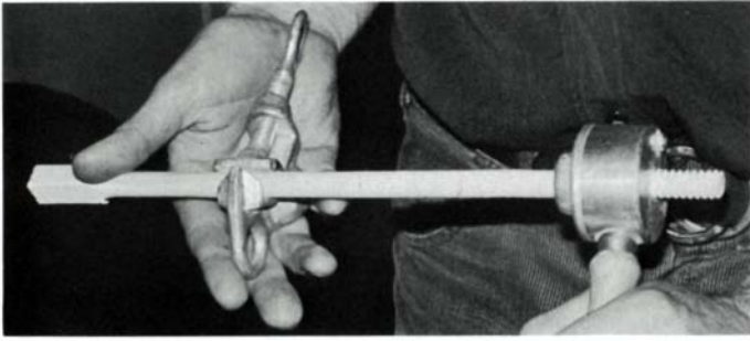
Modified tubing cutter propels dowel through German screwbox.
