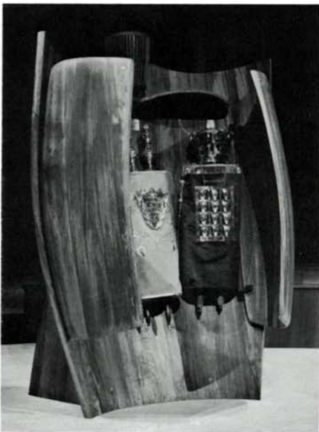
Ark at Interfaith Chapel, University of Rochester, is 8 ft. high and made of steam-bent teak angled and then joined edge-to-edge to create the shell's compound curve. Pieces bent off-the-corner become legs of small table in chapel at Geneseo, N. Y.; plain bends joined edge-to-edge support altar and lectern.
