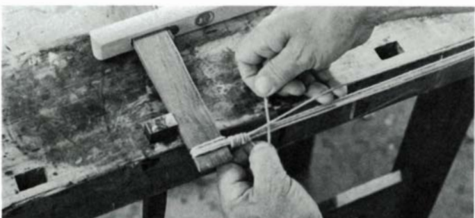
Tensioning string is wrapped four times lengthwise, woven to finish.
