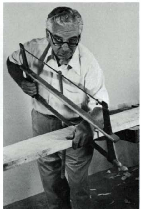
down stroke, away from sawyer. As saw nears end of crosscut (right), sawyer reaches between blade and bridge to catch wood.
