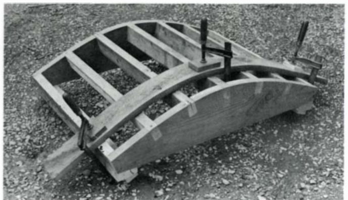
For shallow bends, or when stock is very thin, bending can be done without a strap. The steamed wood is clamped directly to a combination mold and drying jig such as the one shown above.
