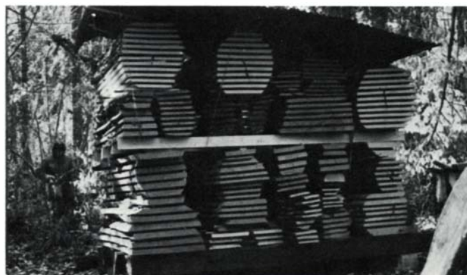
Chain-sawn lumber is stickered and sheltered to dry in air.
