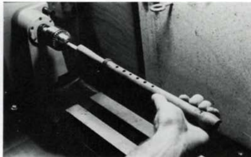
Flageolet is held in V-block, left, to file channel behind mouth that forms upper surface of windway. To sand inside of bore, right, garnet paper is wrapped and glued around dowel and chucked in lathe.
