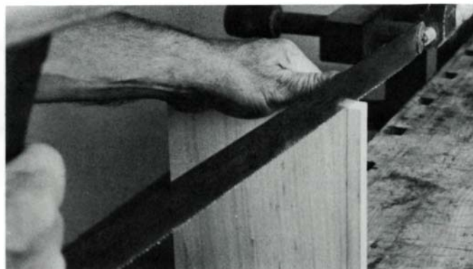
Starting the cut: Frid holds saw loosely, left thumb guiding blade, with eye, blade and cutting line all aligned vertically. Blade is angled so frame will clear wood as cut proceeds.
