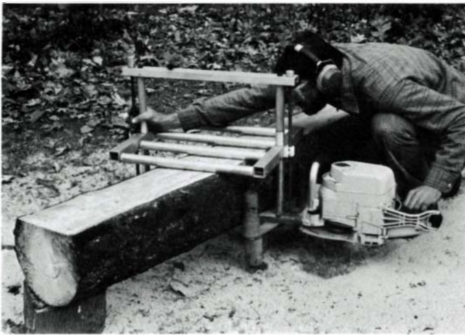
With ends of log resting on vee-cut blocks, Sperber makes bottom cut using one-engine chain-saw mill. Side force generated by engine pulls front and rear vertical rollers against the log. Mill advances at slight angle, at which it cuts best. At end of cut, mill pivots on rear roller as cutting bar swings free.
