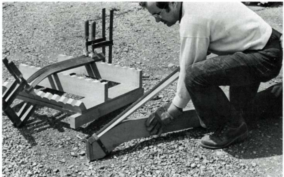
Off-the-corner strap, left, is welded from two sizes of angle iron. Steamed wood fits tightly between end blocks, is tucked under shackle on mold, and forced into place, above. After 15 minutes it is removed, placed in drying jig, and clamped with the aid of blocks notched at 45°.
