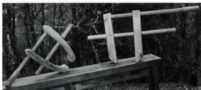
Wooden hand screws may be made in almost any size, with jaws and handles shaped to fit particular types of work.
