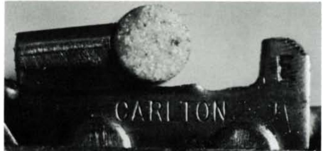
Cutting angle of 45° is obtained by setting grinding stone so that one-quarter of its diameter is above cutter top.
