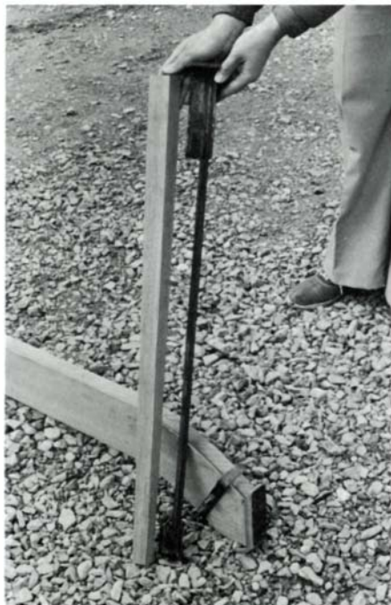
Off-the-corner strap, left, is welded from two sizes of angle iron. Steamed wood fits tightly between end blocks, is tucked under shackle on mold, and forced into place, above. After 15 minutes it is removed, placed in drying jig, and clamped with the aid of blocks notched at 45°.
