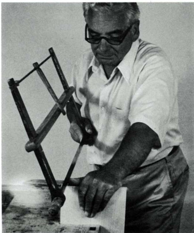
Starting the cut: Frid holds saw loosely, left thumb guiding blade, with eye, blade and cutting line all aligned vertically. Blade is angled so frame will clear wood as cut proceeds.
