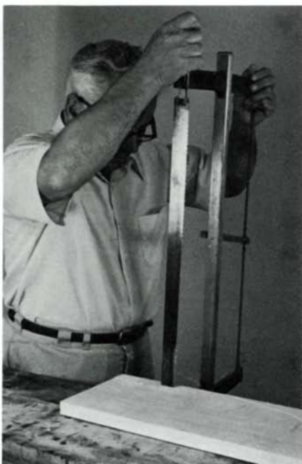
When ripping (left), left hand guides cut and right hand powers whole length of blade downward. Scroll bowsaw (center) also cuts on
