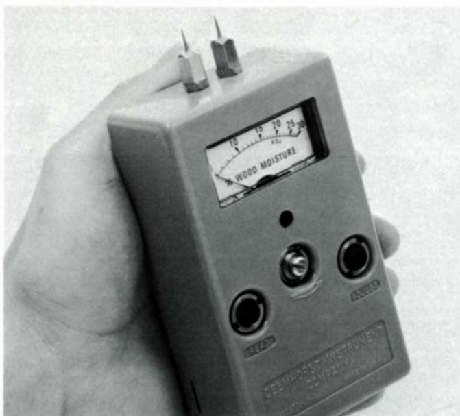
Electrodes are attached to case of pocket-size resistance meter.
