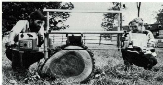
With slabbing rail (end view) in place, first cut is begun.
