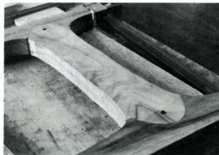
Jim Sweeney makes curved closed bridle joints with precise router jigs.
