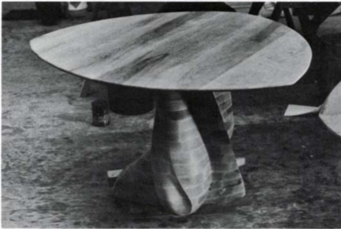
A ball mill helps shape the graceful transition from top to base. After six coats of Watco the table is finished.
