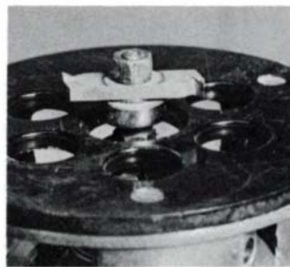
Tongue-and-groove joints can be made with a carbide-tipped slotting cutter in a router, left. At right, shaper cutters shown in the tongue-cutting configuration. Groove cutter is not shown.
