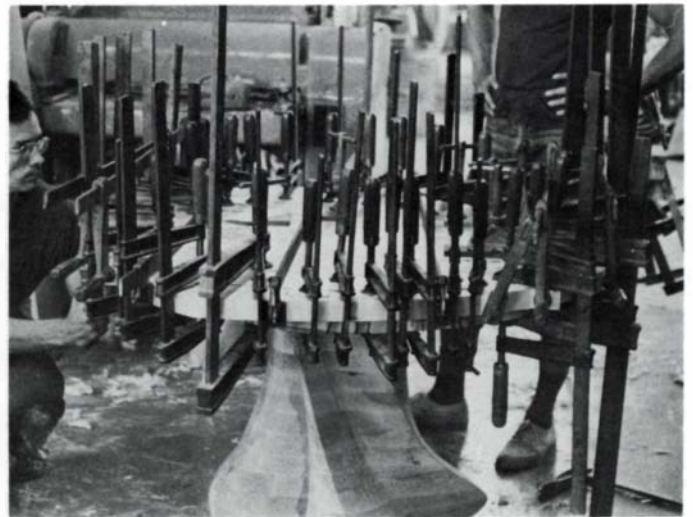
The cavity of the first top layer is carved to remove weight, as it adds no useful glue surface. The top is clamped across to help keep the pieces level, and then laden with clamps until the glue sets.
