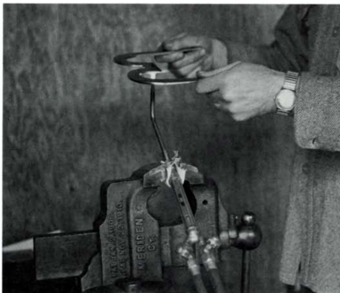
Once forged and ground, the draw knife is heated with an oxyacetylene torch to a bright cherry red, or about 1,450 degrees. As soon as the steel is heated to cherry red, it is hardened by quenching rapidly in a bath of used crankcase oil (5-30 SAE).
