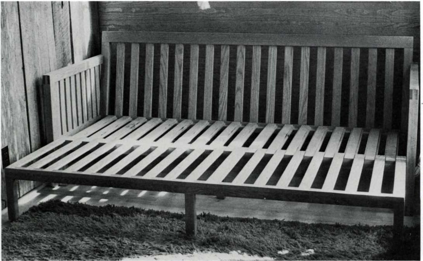
Author used mostly 8/4 stock for the couch because it was readily available. Drawing below gives general dimensions and an idea of how it was put together. Owners use a foam-rubber mattress for sleeping rather than the cushions shown.
