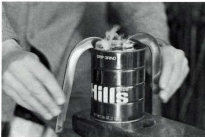
Once forged and ground, the draw knife is heated with an oxyacetylene torch to a bright cherry red, or about 1,450 degrees. As soon as the steel is heated to cherry red, it is hardened by quenching rapidly in a bath of used crankcase oil (5-30 SAE).
