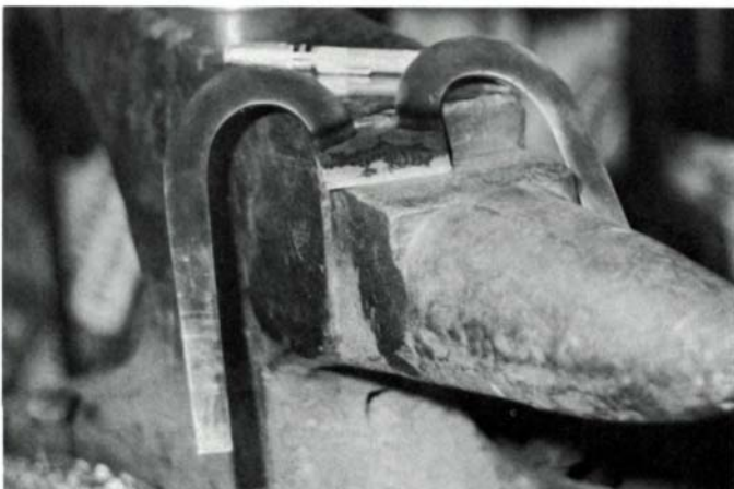
The hardened knife shows oxidation rings, where the curve begins. Temperature-indicating crayon for 500° F is applied to the entire bevel and the blade is ready to temper with a propane torch (right).
