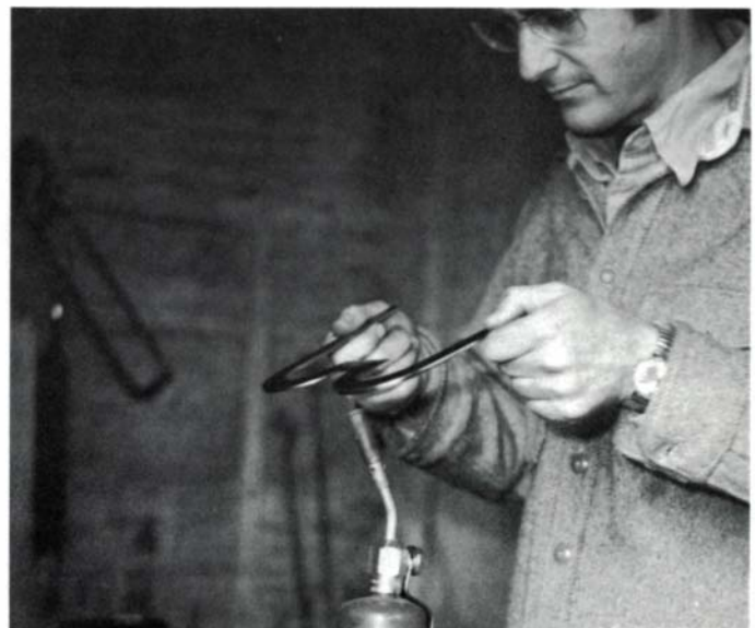
The hardened knife shows oxidation rings, where the curve begins. Temperature-indicating crayon for 500° F is applied to the entire bevel and the blade is ready to temper with a propane torch (right).
