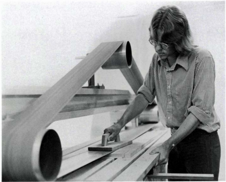
The author's son at work. Third drum gives plenty of working room.
