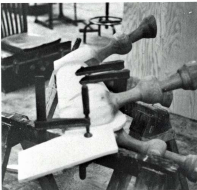
Camel is assembled as split turnings are attached to "back bone" of solid birch plywood using dowels and fox wedges.
