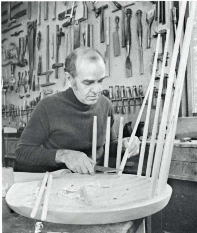
The author making a reproduction (right) of the chair Thomas Jefferson sat in when writing the Declaration of Independence. All woods are the same as the original: maple legs and arm posts, poplar seat and mid-arm back, hickory spindles, white oak arms and crest rail.
