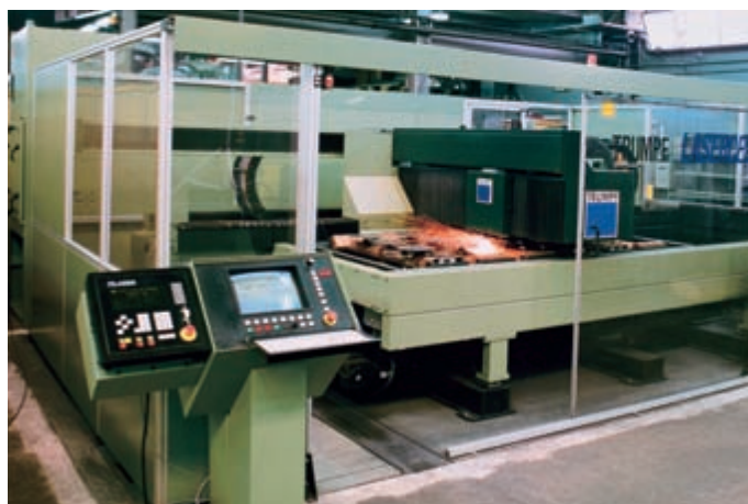
Laser cutting the steel plates.
