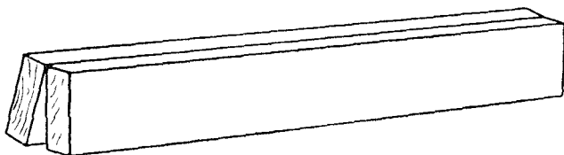
Fig. 2.—How the Wood is held whilst Glueing.
