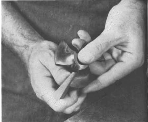
PHOTO BY ROBERT C. SMITHERAM JR. 17-11. Honing the face of a wing cutter with a slip stone.
