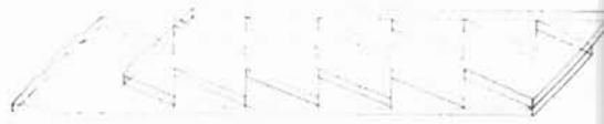
9-59. To grind ends flat and square, place teeth edge of one end toward the back edge of the other end.
