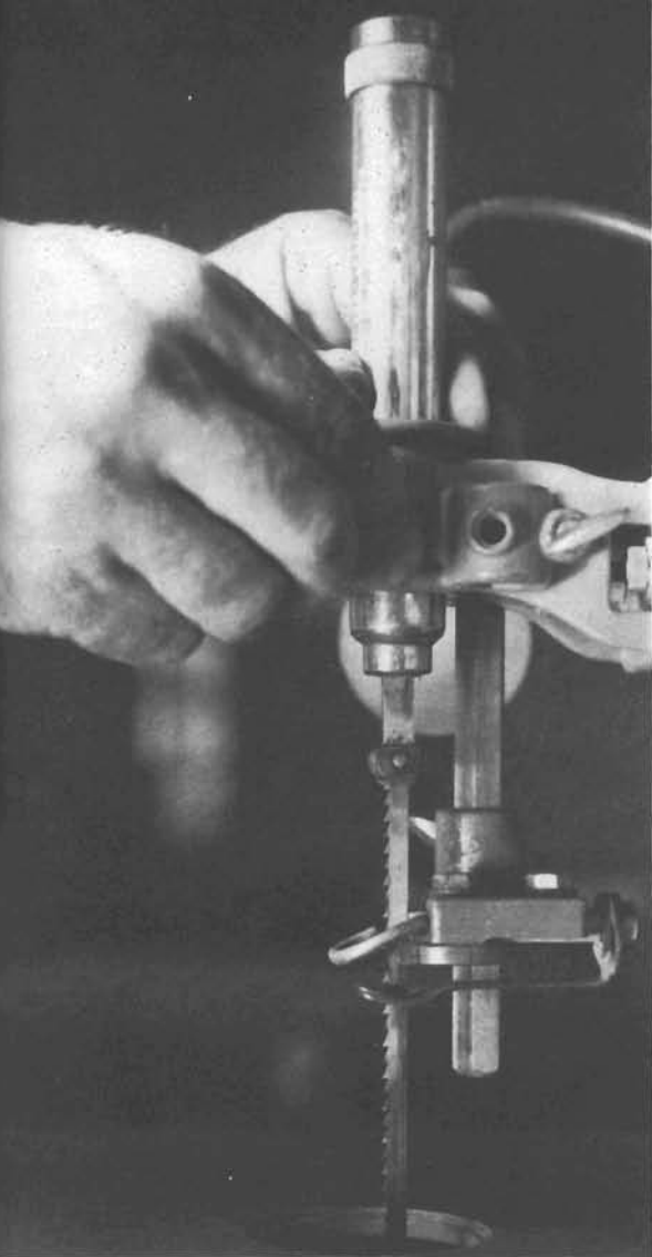
11-5. Top chuck is lowered by loosening tension device.
