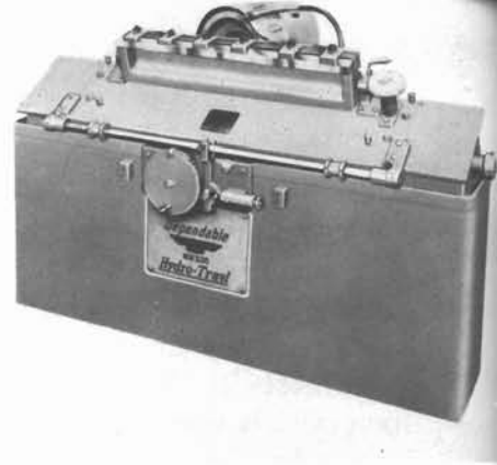
COURTESY DEPENDABLE MACHINE COMPANY 13-3. Knives must be ground on a special grinder to obtain a straight cutting edge.
