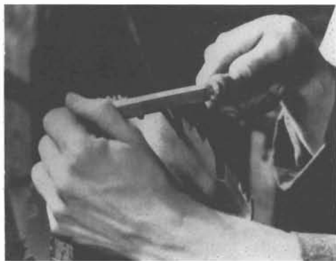
COURTESY SIMONDS SAW AND STEEL COMPANY 10-42. Position of file when filing a combination saw. Use a cant file when the gullet angle is less than 60^\circ .
