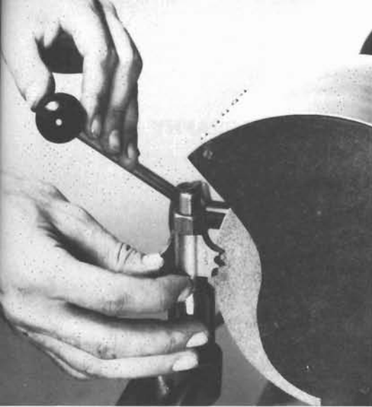
COURTESY MC GRAW-HILL BOOK COMPANY 17-13. Sharpening a three-wing shaper cutter on the side of a grinding wheel with the aid of a special holder. Sharpening is usually done by offhand grinding.
