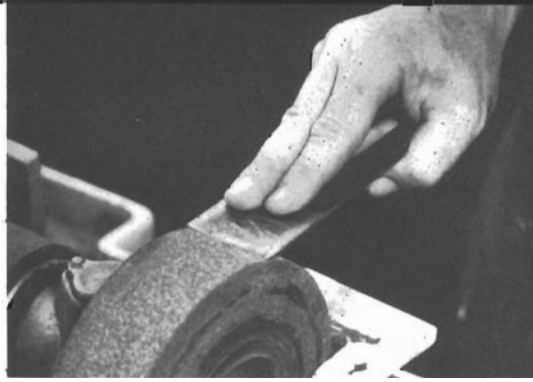
3-9. Position of the right hand on the plane iron in offhand grinding method.
