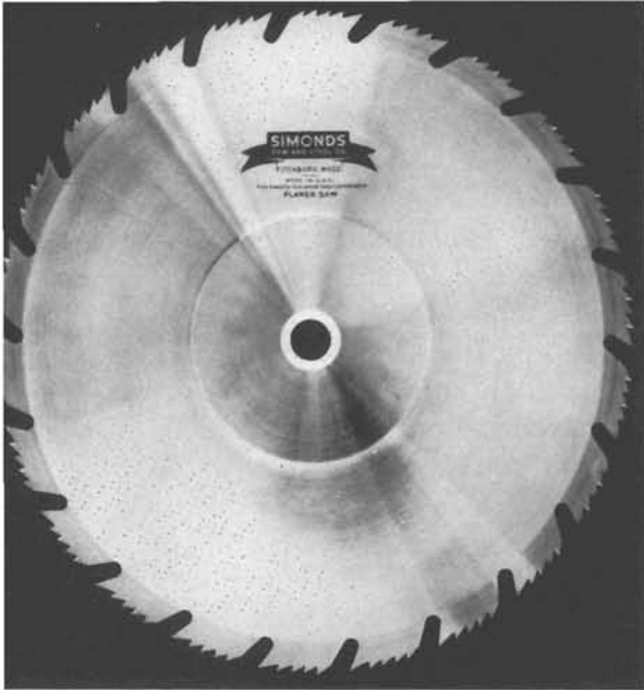
COURTESY SIMONDS SAW AND STEEL COMPANY 10-19. Hollow ground saw. Clearance is provided by grinding a gradual taper from the rim to the collar area.
