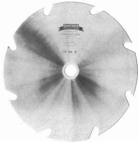
COURTESY SIMMONDS SAW AND STEEL COMPANY 10-61. Cut control saw. Notice the small number of teeth as compared with conventional circular saws.
