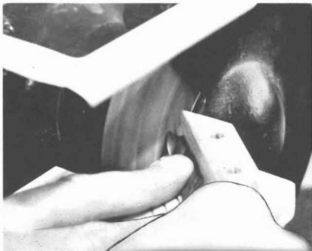
7-22. Grinding a twist drill on a home-made grinding attachment.
