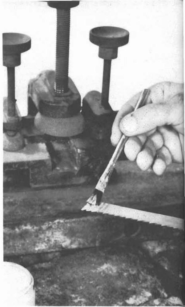
PHOTO BY CHARLES J. PEREZ 9-55. The flux is applied to the joint.
