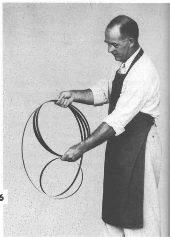
9-37. Hold the one loop and three lower loops with left hand and release loops in right hand.
