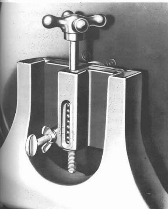
9-14. Compressing coil spring places tension on blade.
