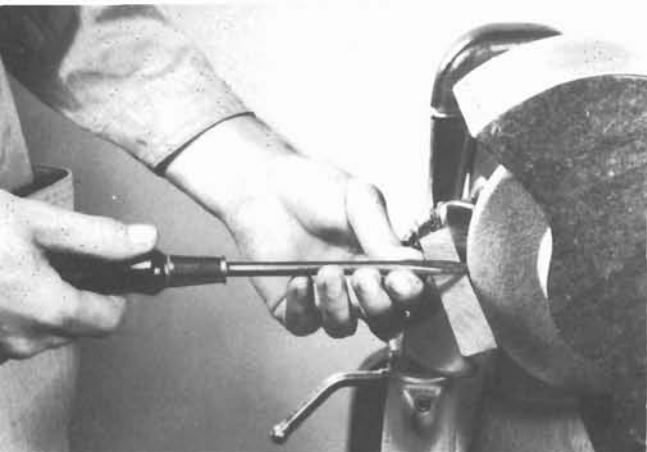
8-6. Grind the tip square on the face of the grinding wheel.
