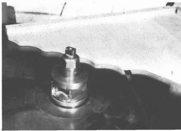
PHOTO BY CHARLES J. PEREZ 17-4. Flat shaper knives are clamped between two slotted knife collars.
