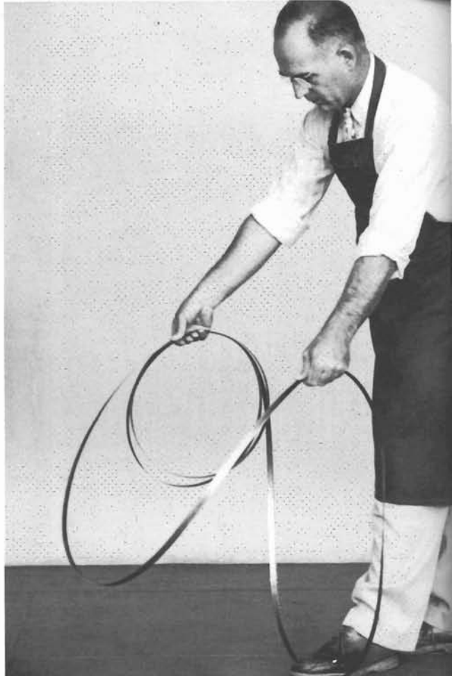
9-31. Holding two loops in left hand and middle and top of large loop in right hand permits top of large loop to fall away from you.
