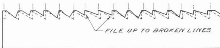
6-15. Shape of teeth after jointing.
