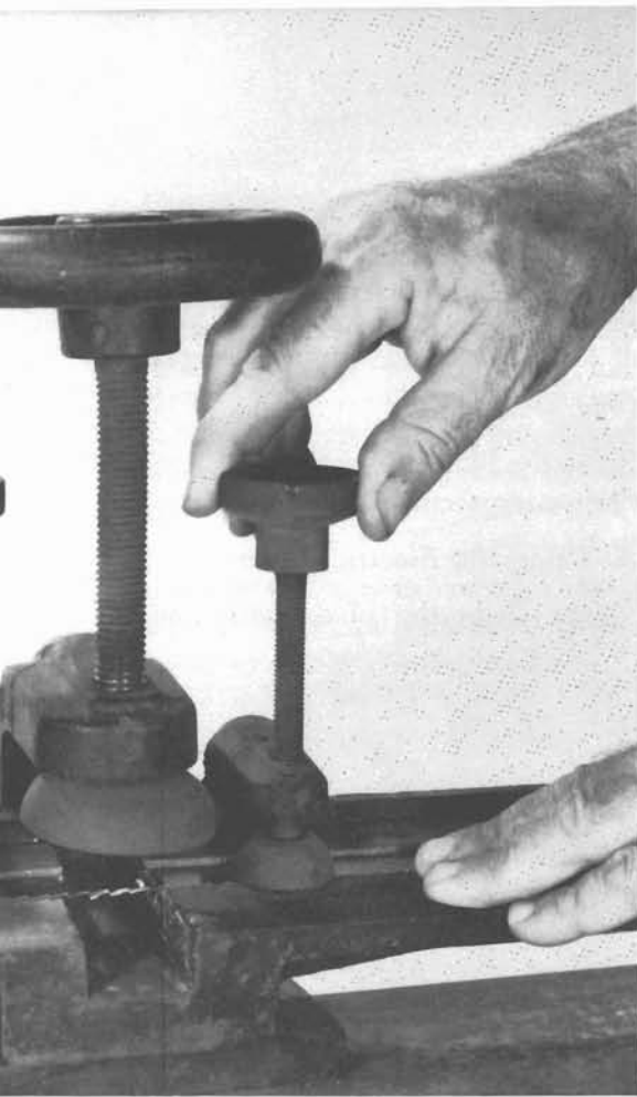
PHOTO BY CHARLES J. PEREZ 9-54. The band saw blade is clamped with the joint in the middle of the clamp throat.
