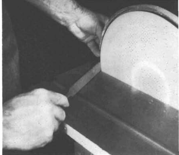
PHOTOS BY CHARLES J. PEREZ 16-10. An old mill file is used to trim the projecting edges of the abrasive disk.
