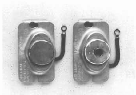
COURTESY GENERAL ELECTRIC COMPANY 18-6. Automatic and manually operated thermal protectors. When the motor has cooled to a safe operating temperature the circuit is automatically closed. The circuit is closed by pushing the reset button on manual protectors.
