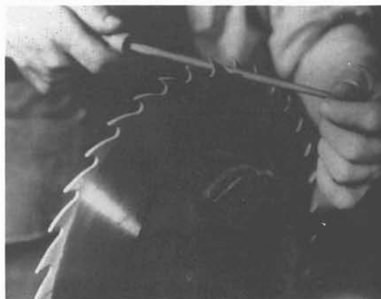
10-47. Deepening the gullets of a rip saw with a round file.
