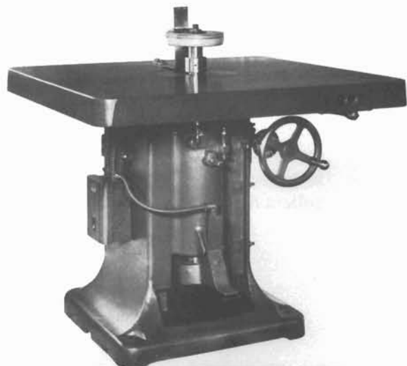
17-1. Heavy shaper. COURTESY OLIVER MACHINERY COMPANY
