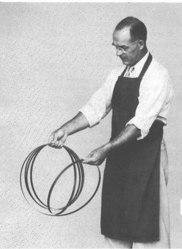
9-36. Notice three loops above two crossed loops below. The continuation of the loop in the left hand forms the two loops held in the right hand.
