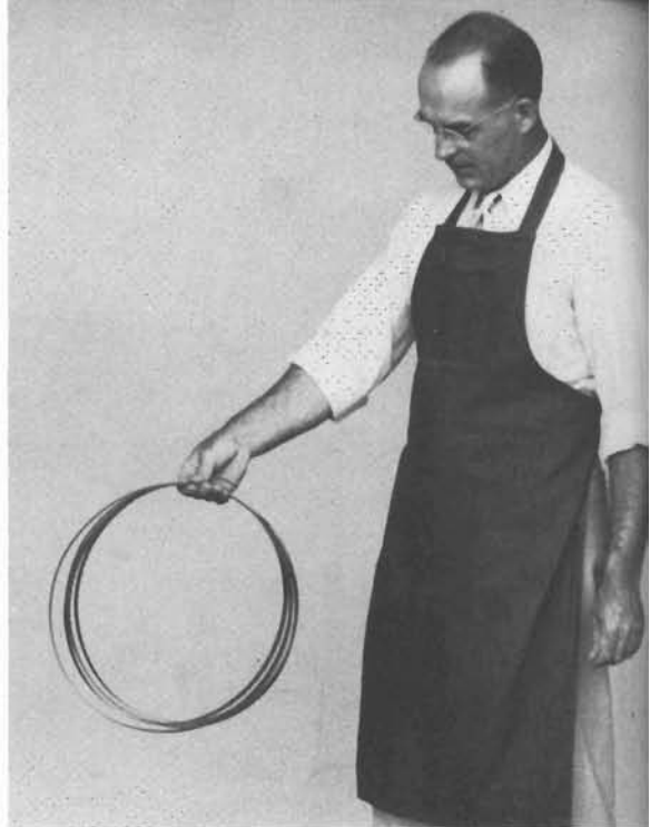
9-35. Blade held in right hand with teeth toward the left.
