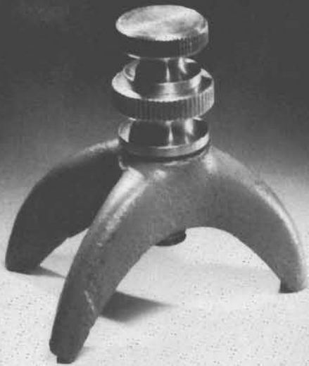
COURTESY BELSAW MACHINERY COMPANY 15-8. Knife setting gauge for planer knives.
