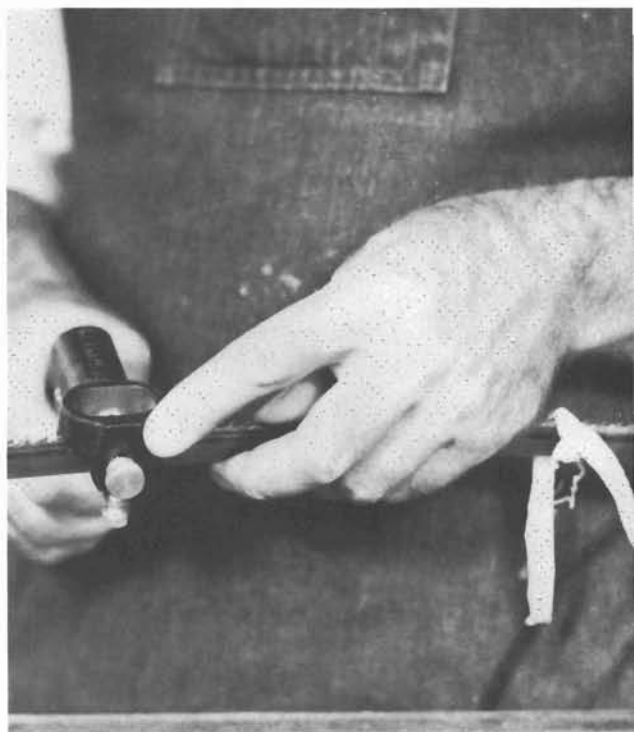
PHOTOS BY CHARLES J. PEREZ 9-43. Mark starting place on blade and set every other tooth toward one side.
