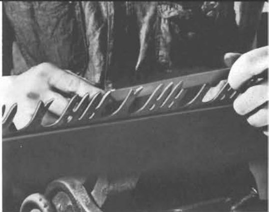
6-31. Filing the crosscut teeth of a crosscut saw, as seen from the rear.
