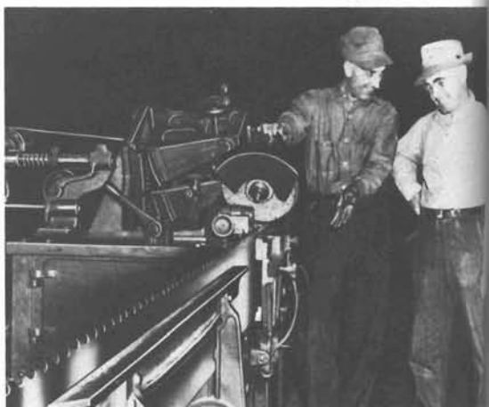
9-49. Close-up view of the process of sharpening a large band saw blade.
