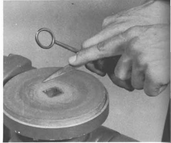
COURTESY ATLAS PRESS COMPANY 8-19. Sharpen very dull scissor edges on a fine grinding wheel.
