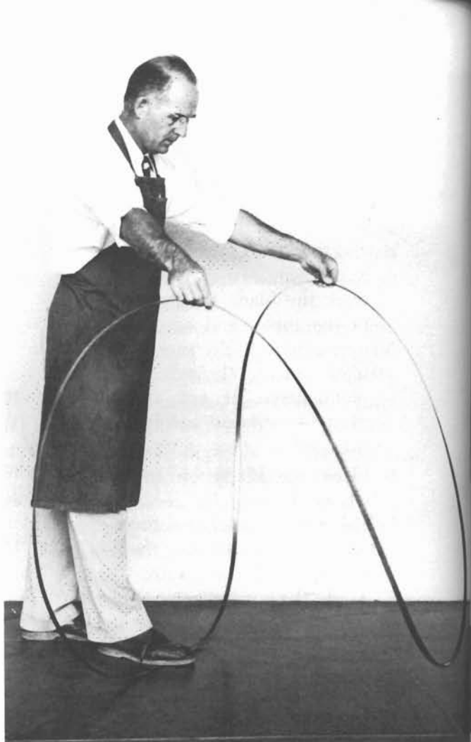
PHOTO BY R. A. MC COY 9-21. Extend your arms, turn the teeth in, permitting top half of the blade to bend away from you.
