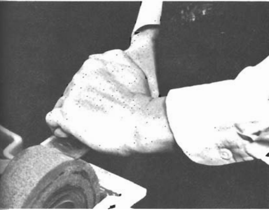
3-8. The plane iron cap can be used as a convenient guide in sharpening a plane iron. Be sure to fasten it at right angles to the plane iron.
