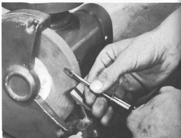
8-9. Faces of a screw driver can also be shaped on the side of a grinding wheel.
