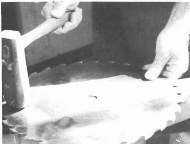
10-10. Blade tension is restored by hammering the body of the saw carefully.
