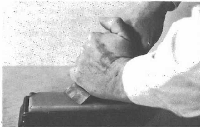
3-9. Position of the right hand on the plane iron in offhand grinding method.
