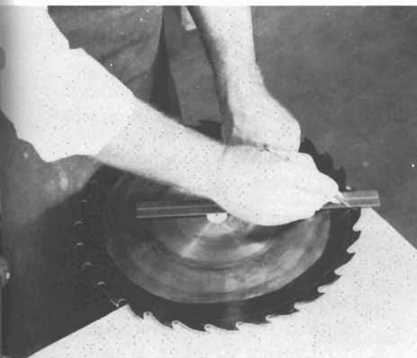
PHOTO BY ROBERT C. SMITHERAM JR. 10-54. Line from point of tooth to center of saw intersects circumference of circle.
