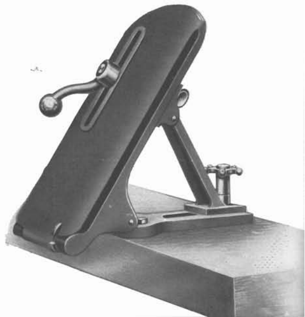
10-27. The same vise in a tilting position. When sharpening dado blades this position is preferred.
