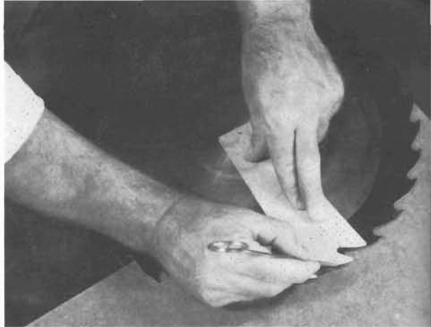
PHOTO BY ROBERT C. SMITHERAM JR. 10-59. Outlines of the new teeth are scribed on the saw. The common point on the template is placed on the lines extending through the circumference of the circle.
