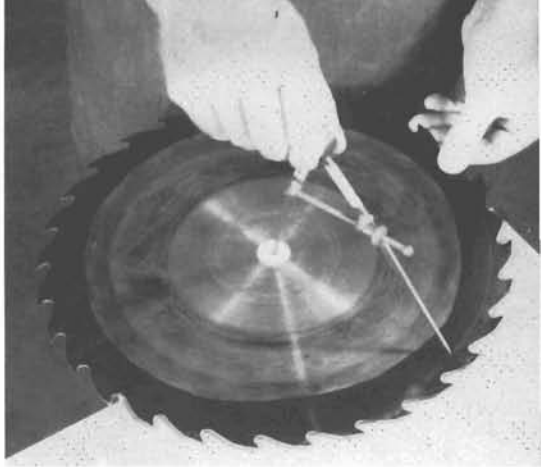
PHOTO BY ROBERT C. SMITHERAM JR. 10-53. Circle is drawn on dyed side of saw, using dead center end in arbor hole piece for the center.
