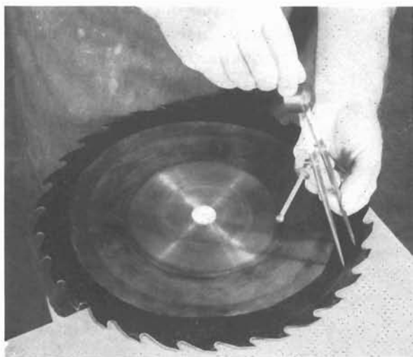
PHOTO BY ROBERT C. SMITHERAM JR. 10-55. Equal spaces are located on circumference of circle.
