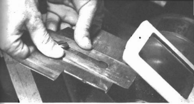
3-8. The plane iron cap can be used as a convenient guide in sharpening a plane iron. Be sure to fasten it at right angles to the plane iron.
