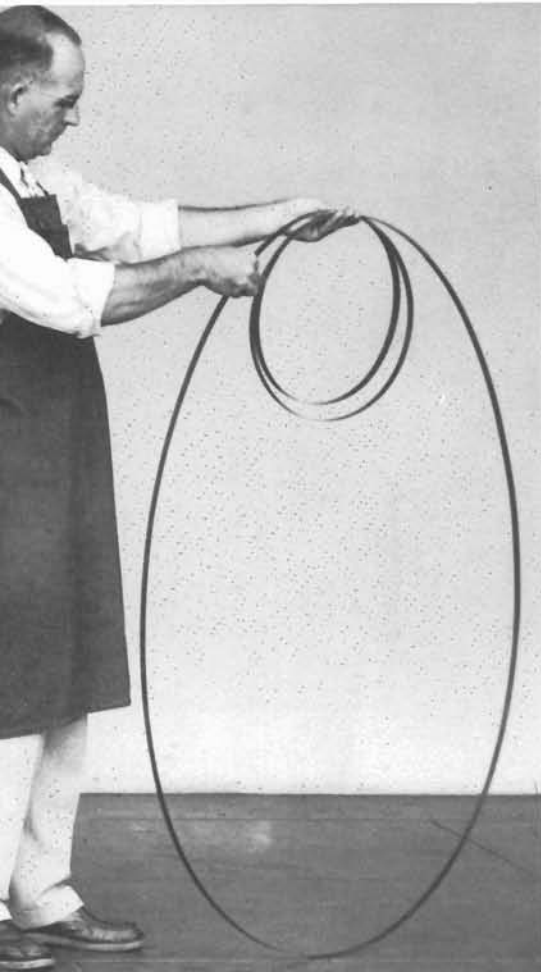
9-30. Blade coiled in three loops showing one large loop.
