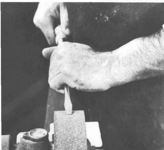
8-7. Grind the tip to the proper shape on the face of the wheel, using offhand method.
