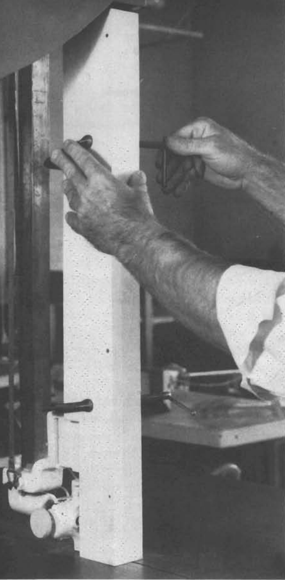
PHOTO BY ROBERT C. SMITHERAM JR. 9-12. Guard placed over blade while tire is being shaped.
