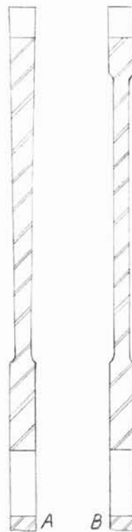
10-18. Two methods of hollow grinding saw blades.
