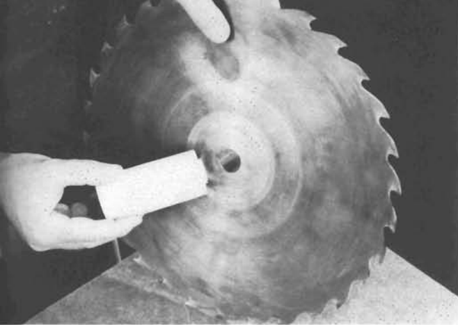
PHOTO BY ROBERT C. SMITHERAM JR. 10-52. The dead center end of a piece of turned stock fits the arbor hole tightly.
