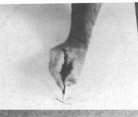
PHOTO BY ROBERT C. SMITHERAM JR. 10-49. Circumference of circle is divided into same number of equally spaced points as there are teeth in saw. Note how tooth shape is carefully designed.
