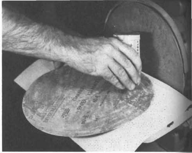
16-7. An even coat of mastic cement is also applied to the abrasive disk.
