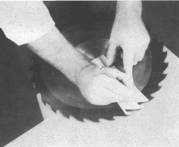
PHOTO BY ROBERT C. SMITHERAM JR. 10-58. Locating a common point on edge of template.
