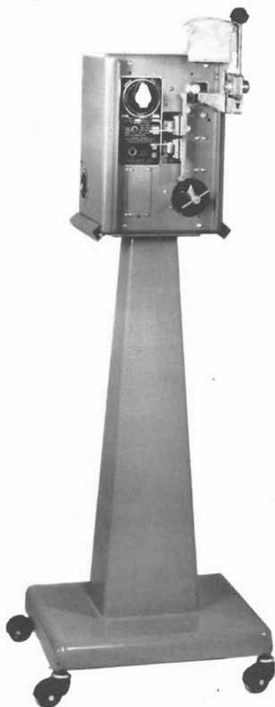
COURTESY GROB BROTHERS, INC. 9-58. Butt welder used for joining narrow band saw blades.
