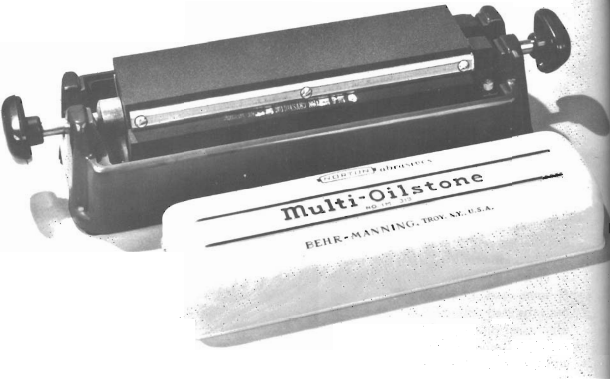
1-20. Multi-oilstone includes three stones: coarse, medium, and fine. They revolve in the container as shown.
