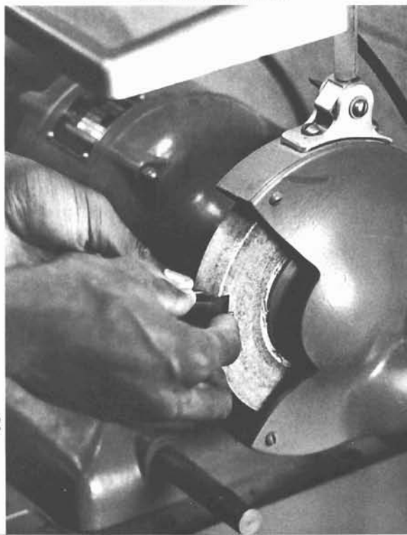
17-12. Sharpening a three-wing shaper cutter by offhand grinding on the side of a grinding wheel.
