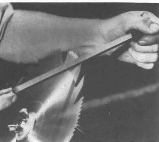
COURTESY SIMONDS SAW AND STEEL COMPANY 10-46. Position of file when sharpening a dado blade. Notice the protective tip on the end of the file as a precaution against possible injury.
