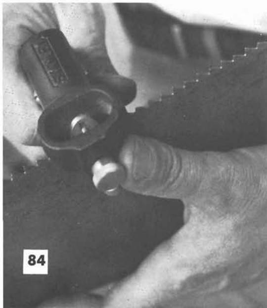
6-16. Setting rip teeth, using a handsaw set.
