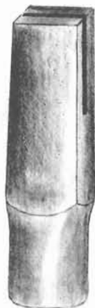
8-3. Hammer handle prepared with saw kerf to hold thin wooden wedge.
