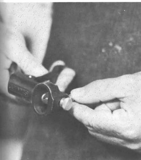
PHOTO BY CHARLES J. PEREZ 9-42. Adjusting hand set to set not more than one-half the depth of the tooth.
