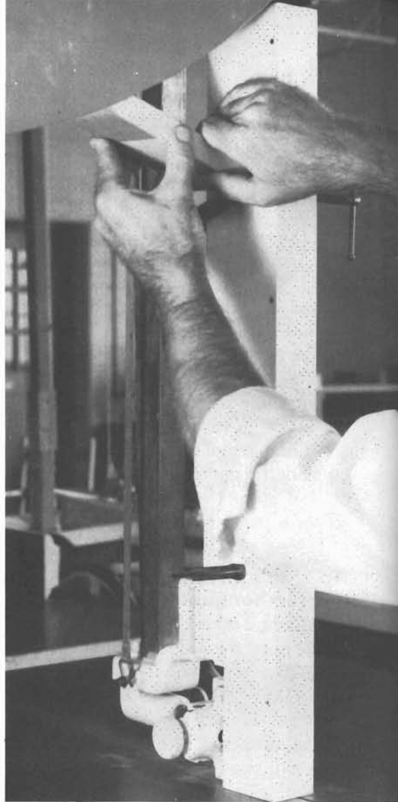
PHOTO BY ROBERT C. SMITHERAM JR. 9-13. Shaping tire on upper wheel with shaping tool.
