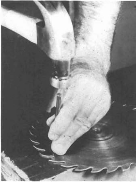
PHOTO BY CHARLES J. PEREZ 10-25. To stop small cracks, center punch both sides of the saw at the end of the crack.
