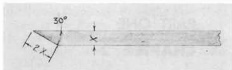
2-4. Bevel length equals twice the thickness of the tool. Depending upon the material, this proportion may vary somewhat.
