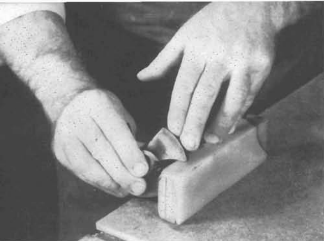
PHOTO BY ROBERT C. SMITHERAM JR. 17-10. Solid wing cutters are sharpened by grinding and honing on the face only.
