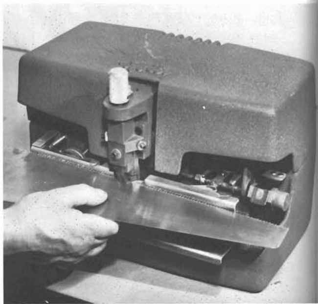
6-17. Setting a handsaw on the Foley automatic power setter.
