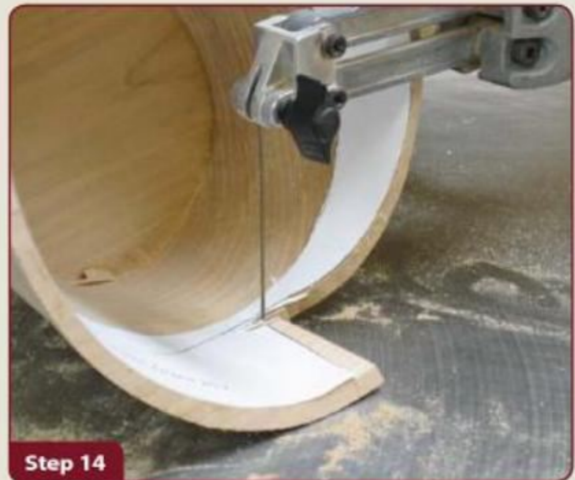
Cut off the waste if needed.
