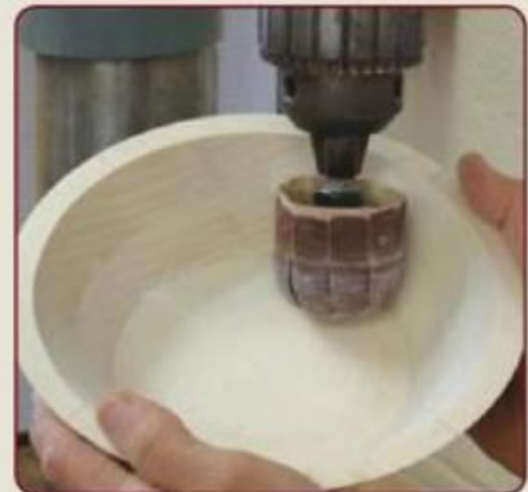
Use inflatable ball sanders to sand interiors.
