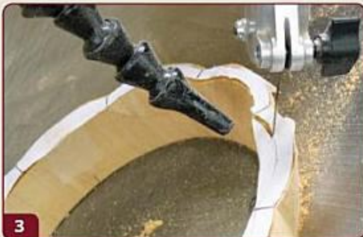
3 Cutting the inner petals. Tilt the saw table 40°, left side down. Cut clockwise along the inner edge of the pattern. Be careful not to cut into the lower edge of the ring.
