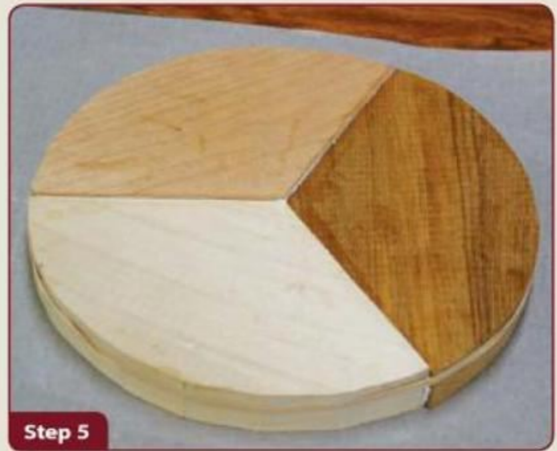
Glue the three segments together.
