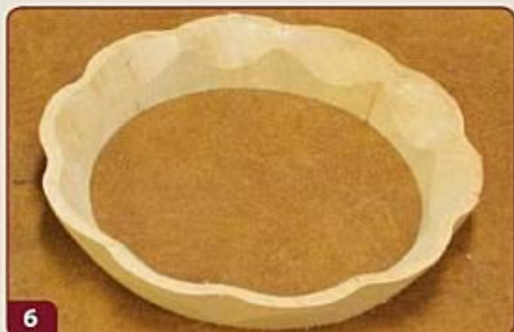
6 Completing the rough-sanding. The ring is left rough at this point to avoid damage during glue-up. Final sanding will be done after the bowl is glued together.
