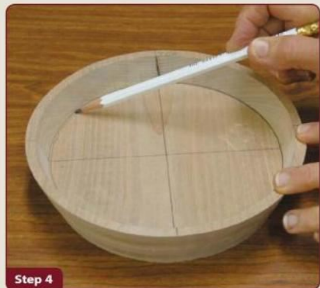
Step 4 Trace the inside of the ring on the blank.
