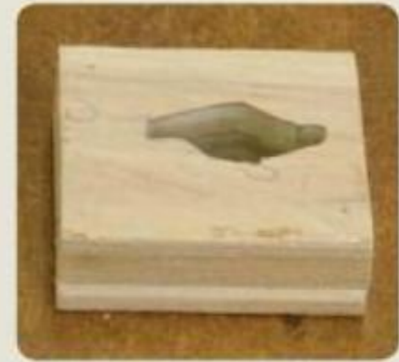
This shop-made device makes it easy to tighten blade holders.
