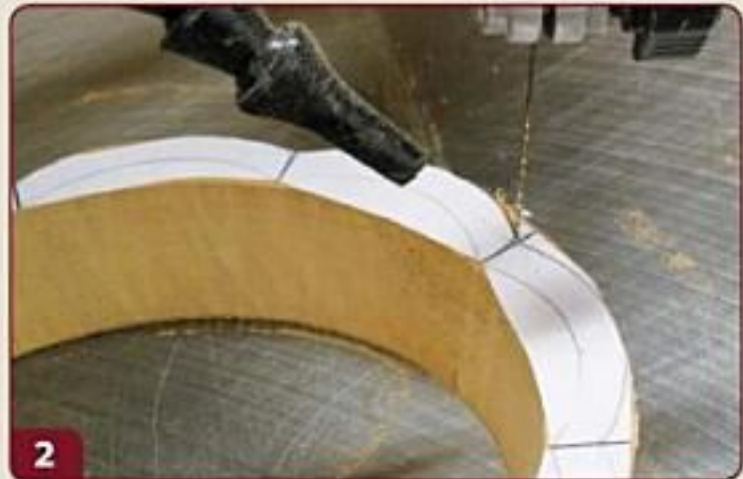
2 Cutting the outer petals. Tilt the scroll saw table 15°, left side down. Cut clockwise along the outer edge of the pattern.
