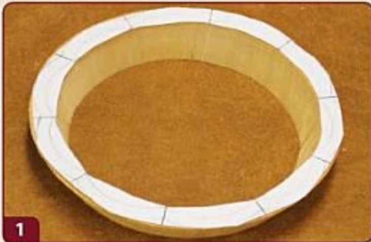
1 Attaching the pattern. Glue the pattern for the petal edge to the top rim with repositionable adhesive.
