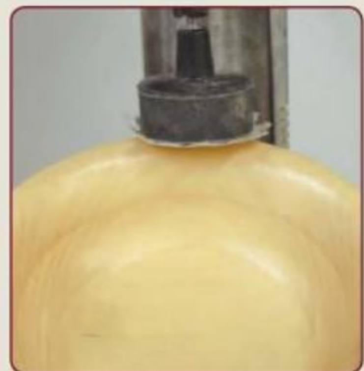
Use inside-to-outside strokes to shape the lip's outward flare.
