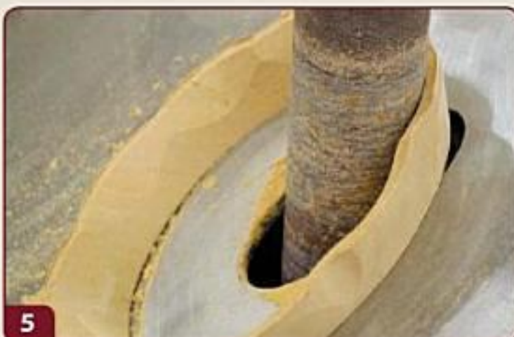
5 Sanding the inside. Smooth the inner edge with a spindle sander, table set to 40°.
