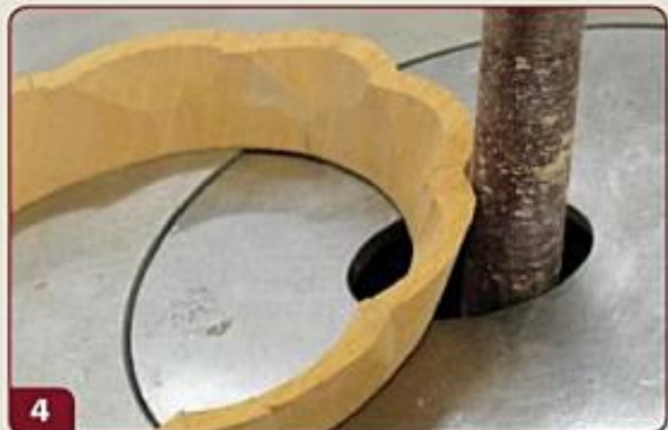
4 Sanding the outside. Smooth the outer edge with a spindle sander, table set to 15°.
