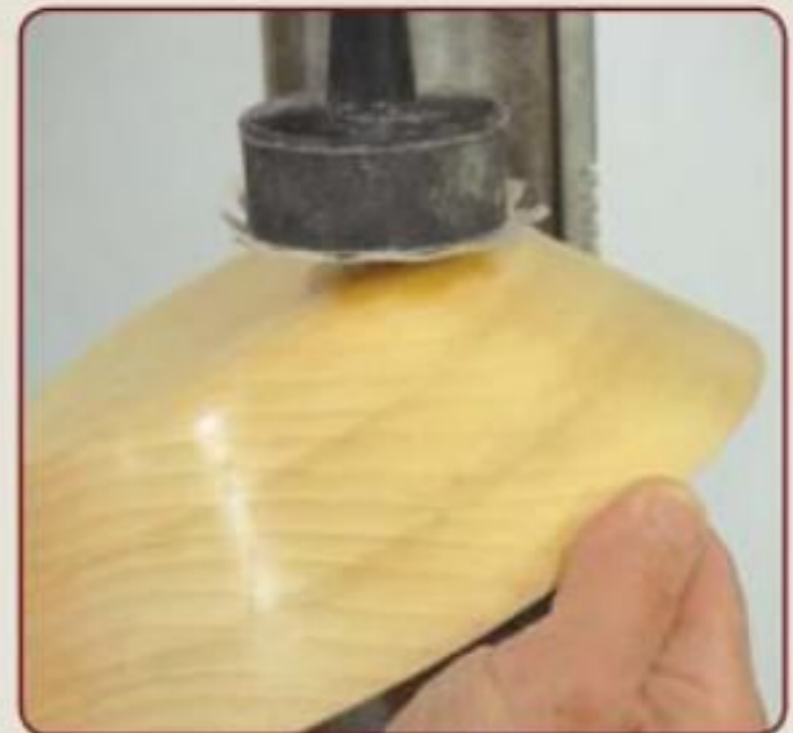
The base can be contoured after being glued to the bowl.
