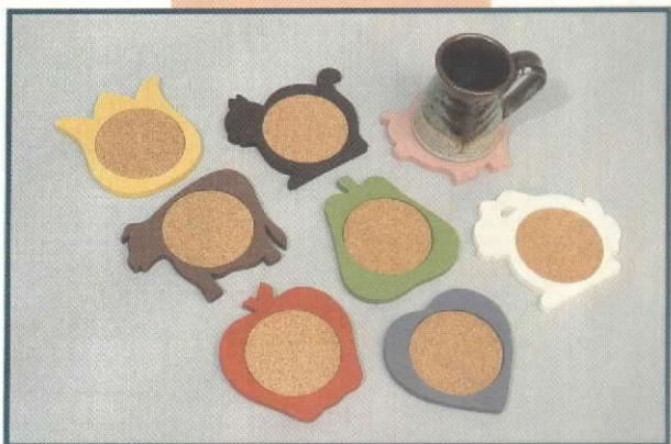
Each of these coasters is made from two layers of 1/4" plywood with a 1/8" thick cork inlay.
