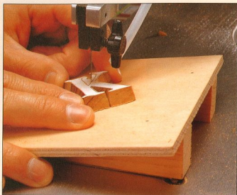
No matter what scrollsaw you use, this simple 10° auxiliary table helps you make beveled cuts in any direction.
