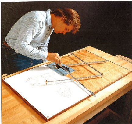
With the eagle pattern centered in the 2:1 ratio rectangle and the blank paper in the copy area, we're doubling the size of the pattern onto the blank paper.
