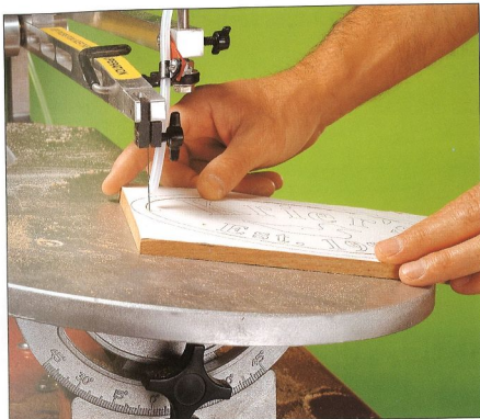
Tilt your scroll saw table 10° to the left or right and keep the waste side of the cut on the downhill side of the blade.
