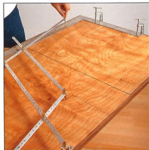
Follow the outline of the copy-area rectangle with the tracing point to mark the 4:1 ratio rectangle on the drawing board. Darken lines with a felt-tip marker.
