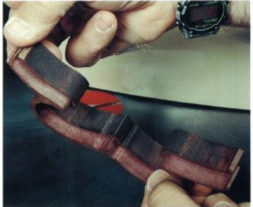
You can see the result of two cuts with the same blade and speed in this piece of purple heart wood. The top one was done without the tape and shows much burning. The bottom one was done with the tape in place.
