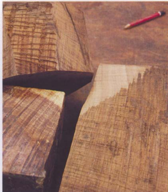
Corrugations on a tree (left) indicate highly figured wood within (right).
