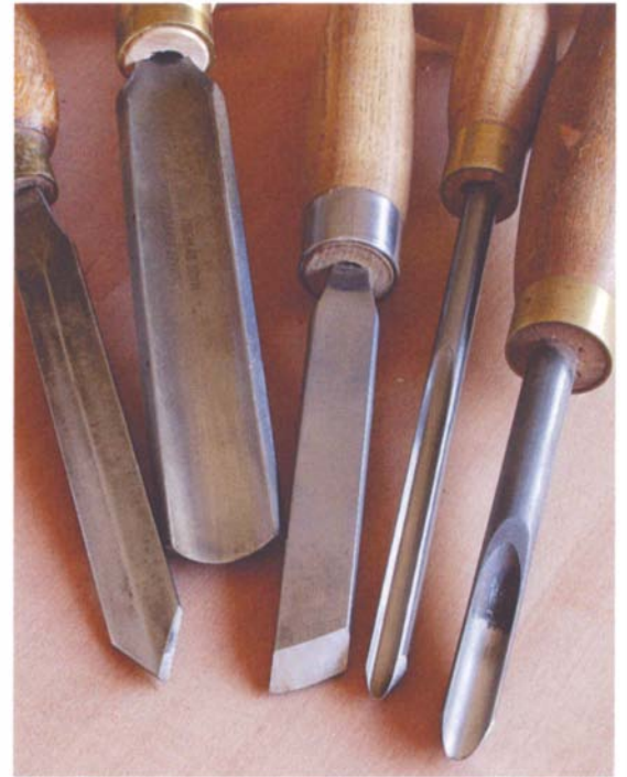
Center-work tools commonly include ( from left ) a parting tool, a roughing gouge, a skew chisel, and various spindle gouges.
