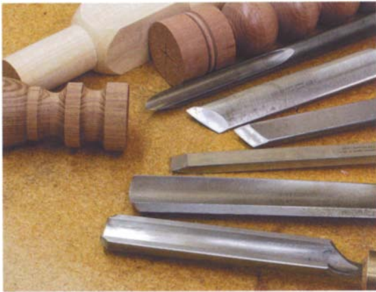
Center-work tools ( from top ): detail gouge, skew chisels, beading and parting tool, shallow and deep roughing gouges.
