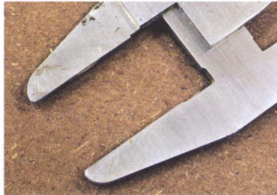
Rounding over the tips of the jaws on vernier calipers prevents them catching on a spinning workpiece.
