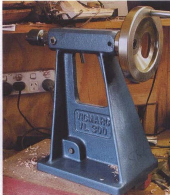
When a heavy tailstock is not in use on the lathe, keep it on its own stand, set at lathe height to prevent back strain from lifting.
