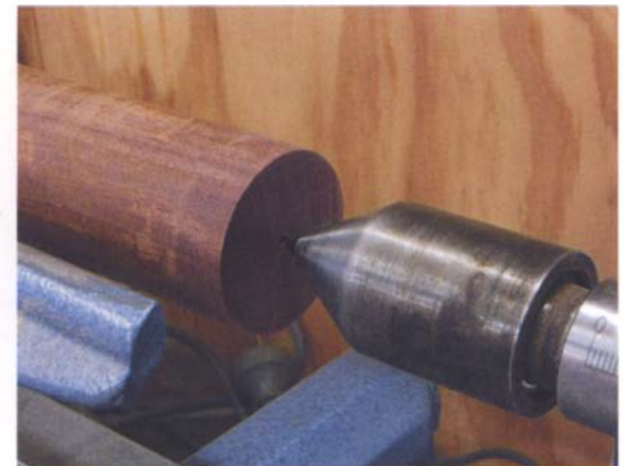
To check the alignment halfway down the bed, inspect the rotation of a chuck-mounted cylinder in relation to the tail-center point.
