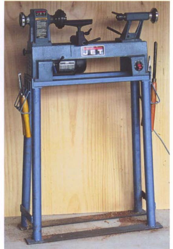
A tailor-made stand can raise a lathe to any appropriate height—like this one made by its tall owner.
