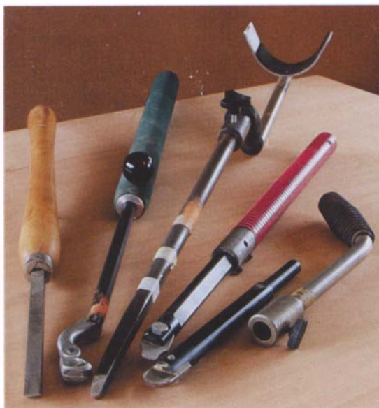
Deep-hollowing tools need to be long and strong or have a Stewart system arm-brace ( center ) or pistol-grip handle ( right ).
