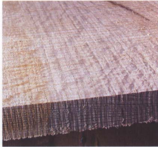
Rays parallel to the cut face yield a ribbon figure.
