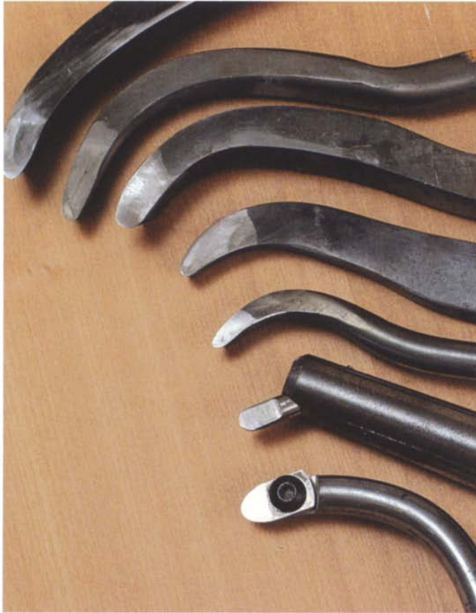
Bent scrapers enable you to hollow out vase forms with small openings.
