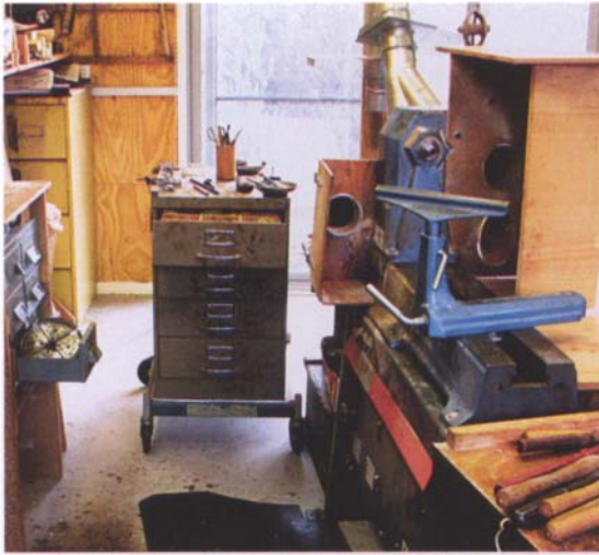
A trolley for tools and a mobile accessory cabinet are easy to roll clear for cleanup or making space for specific tasks.
