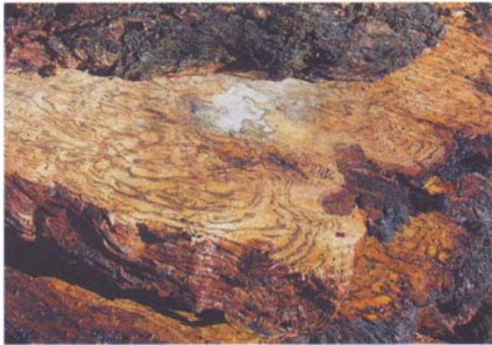
A dramatic, open-grained eucalyptus burl like this is, for safety, better worked thick than thin.
