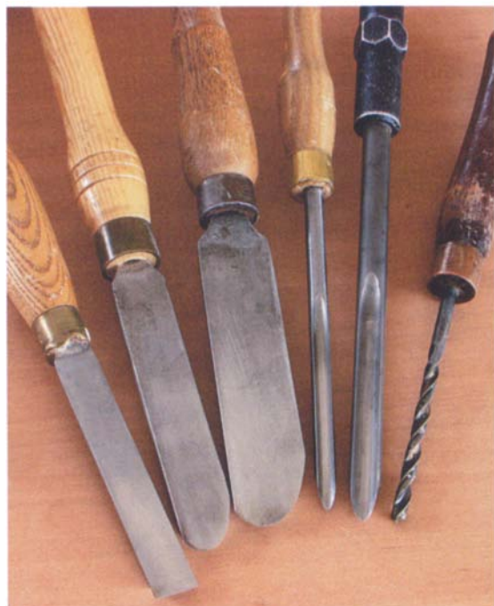
End-grain hollowing tools include ( from left ) a square-end scraper, round-nose scrapers, spindle gouges, and a depth drill.
