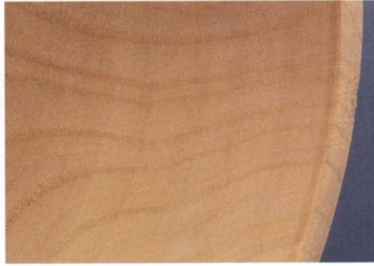
This surface could have been cut cleaner, but sanding soon removed the gouge marks on this 10-in. (250mm) ash bowl.
