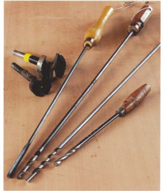
Forstner or multispur bits ( left ) will bore large-diameter holes in items such as pepper mills and hollow forms. Long drills and augers ( center ) are used for drilling out lamp bases. Many holes can be bored freehand on the lathe using a depth drill ( right ).
