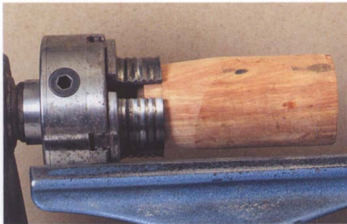
End-grain blanks are most securely held in a chuck like this Vicmarc fitted with shark jaws. The jaws should abut a shoulder.
