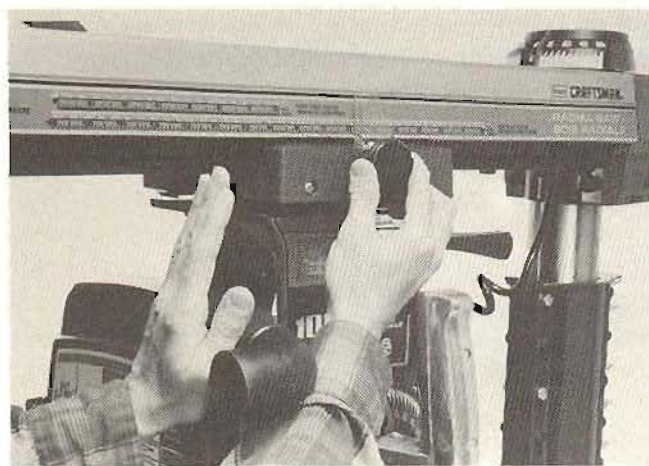
Fig 3-18 Testing rip clamp
