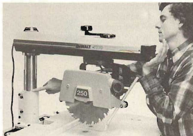
Fig 3-27 Testing column pivot
