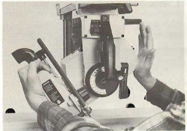
Fig 3-14 Testing bevel clamp
