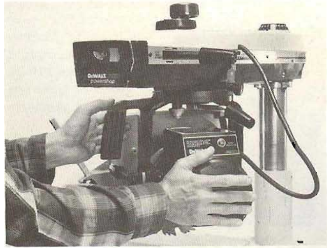
Fig 3-10 Testing the yoke clamp
