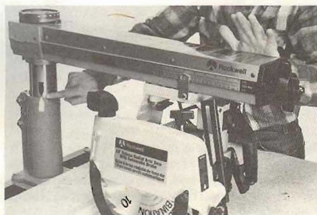
Fig 3-33 Testing column rotation
