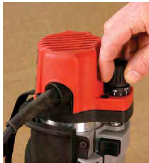
The Milwaukee's fine adjustment on its fixed base was the favorite of the routers tested.
