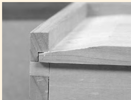
Traditional drawers used raised panels made of solid wood for the bottoms. These are easily made on a router table with a raised-panel bit, then fit into a groove in the drawer sides.
