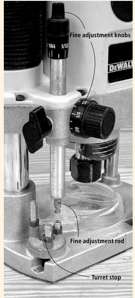
The fine-adjustment knobs make the depth as accurate as possible.
