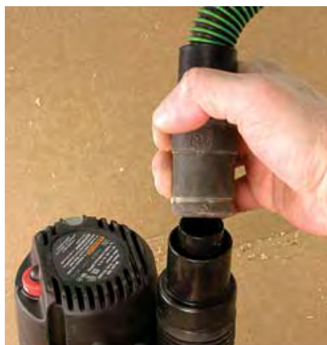
The Porter-Cable, as well as the DeWalt have the dust collection attachment at the top of the column, a more convenient location.
