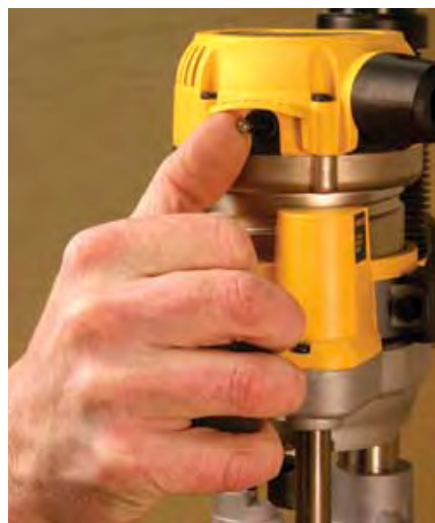
The switch on the DeWalt is in an easy-to-locate and easy-to-operate position.
