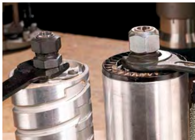
The large cast wrench of the Milwaukee (right) made for easy bit tightening. The thin stamped wrench of the Makita (left) tended to slip off the nut.
