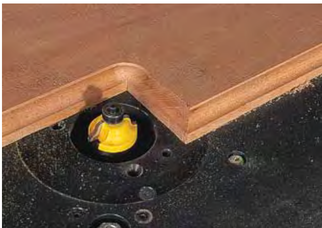
One of the big advantages of router tables is that they can sneak into tight corners a shaper cannot. The ogee profile on this piece will need to be finished up with carving, but this cut would be almost impossible on a shaper.
