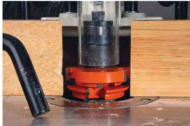
The tall spindle on a shaper allows it to be used with taller cutters, such as crown moulding cutters. Even with this large stile-and-rail cutter installed, you can see how much spindle is still available.
