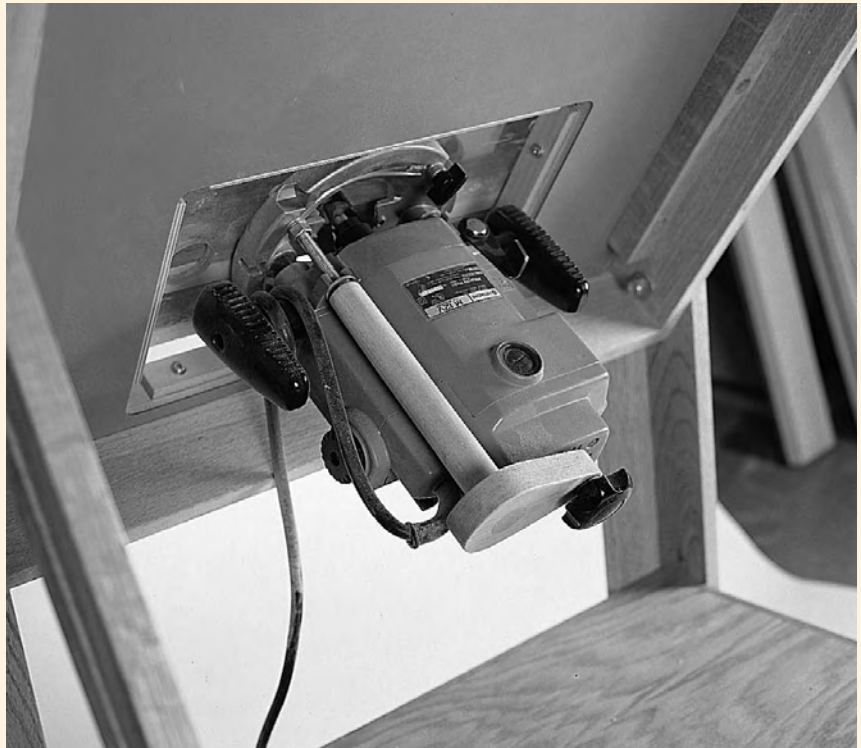
The crank fits most plunge-style routers and helps greatly when the tool is positioned upside-down in a router table, such as the tilting router table discussed earlier.
