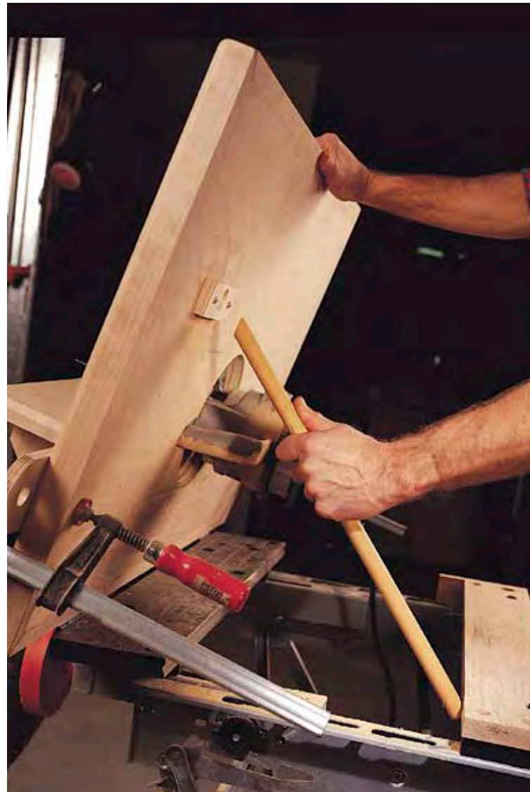
Once the tabletop is hinged to the Workmate's front board, it's easy to locate the positions for the prop stick and stick bracket. Note the shop-made replacement board for the Workmate top.
