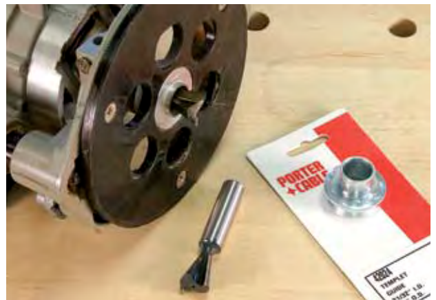
The \frac{3}{4} " outside-diameter guide bushing must be reduced in length to protrude less than \frac{1}{8} ". This modification allows the base of the router to lay flat on the workpiece.
