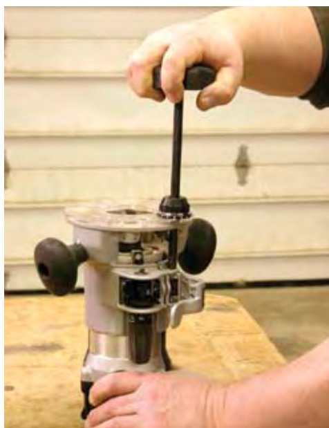
Several of the routers offered above-the-table depth adjustment, but the Porter-Cable is the only one with an above-the-table motor latch.
