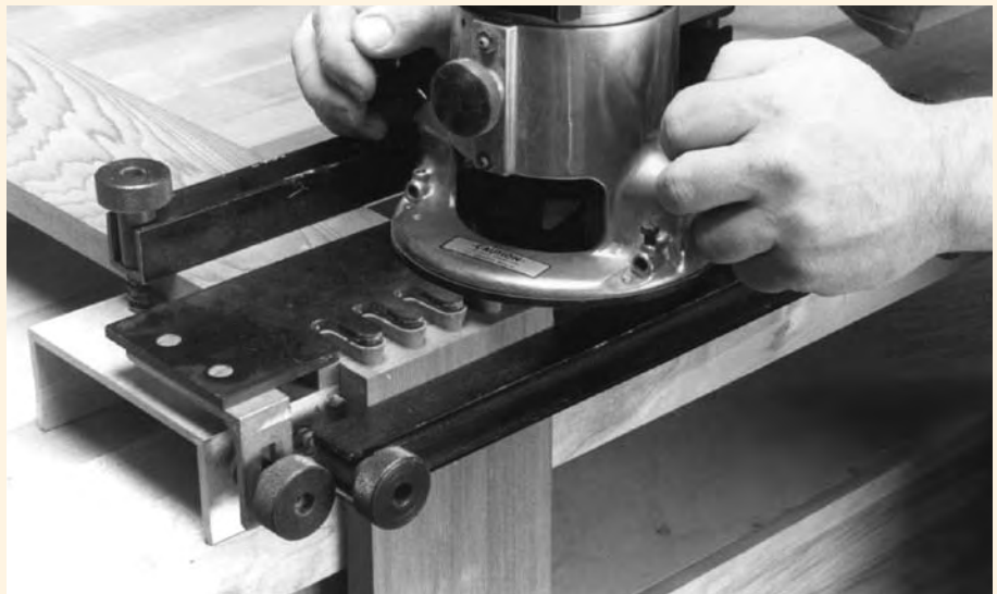
On half-blind dovetails (above), the joint is hidden from view on one side. This makes it ideal for the fronts of drawers and other applications where you don't want to see the joinery. Through dovetails (right) are visible from both sides and are often used for decoration, as well as joining.
