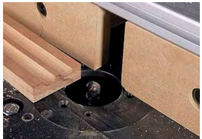
Another advantage of router tables is that you can cut directly above the bit, such as with this fluting shown here. Making this cut on a shaper requires a trickier setup.
