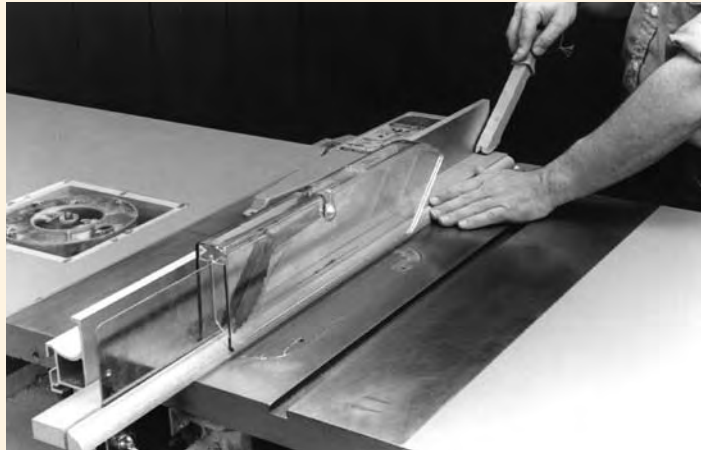
When you're ready to shape your workpiece, first cut the end grain along the ends ...
