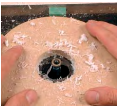
After cutting an adequately sized starter hole with a drill bit, a bearing-guided flush-cutting bit does a nice job of shaping the interior holes to match the template.
