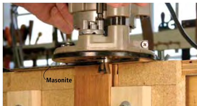
The secret to this jig is the 1/8"-thick Masonite guide piece. This matches the depth of the dado, so the only adjustment needed is to move the guide piece in or out to establish the finished width of the dovetail tenon.
