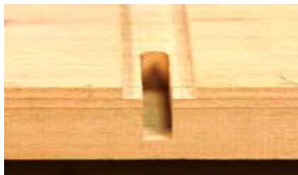
Use the modified guide bushing and a \frac{3}{8} " straight bit to prepare the socket for cutting the dovetail.
