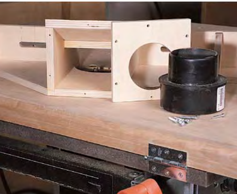
Inside view of the dust chute from the rear including the plastic 4" to 3" dust-collection hose adapter. Rout the 3" hole for the adapter with the circle-cutting jig or use a "fly cutter" in your drill press.
