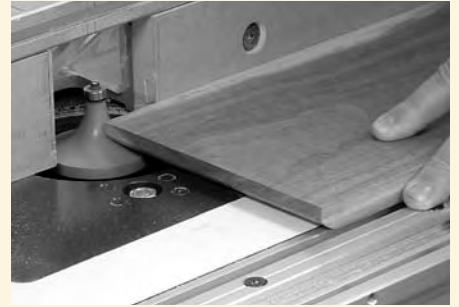
... then cut the long grain along the edges.
