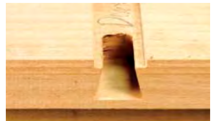
Use the same guide bushing and a \frac{3}{4} " dovetail bit to finish the dovetailed part of the joint.
