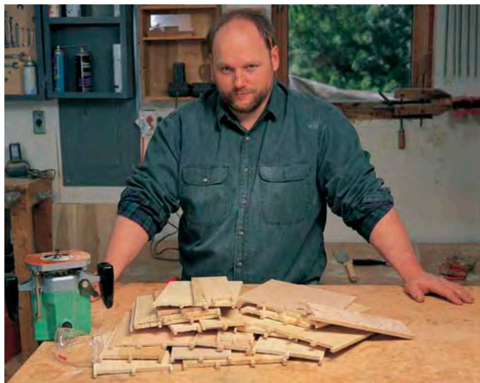
After a while you'll have enough templates to cut dovetails for almost any drawer.
