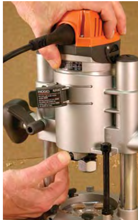
One feature can get in the way of another. To change bases on the Ridgid and Freud routers, the spindle lock must be depressed.
