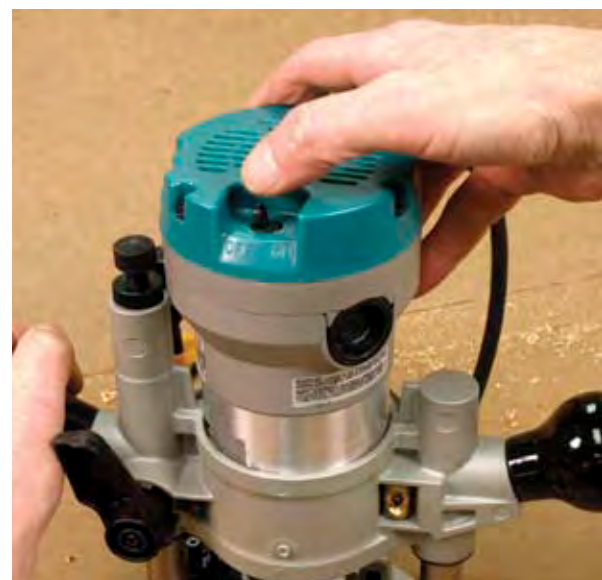
For some switches, such as on this Makita, it's necessary to remove one hand from the router to turn it on or off.
