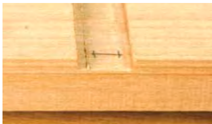
The first step is to mill all of the dados to a depth of \frac{1}{8} " with a \frac{3}{4} "-diameter straight router bit.
