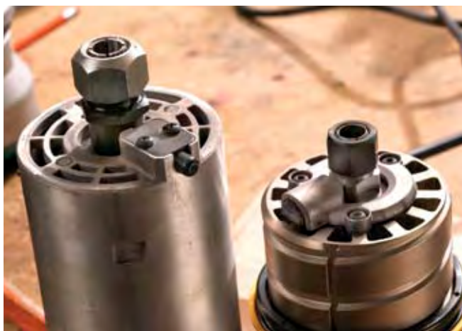
Spindle locks sound convenient, but they all had problems. The Ridgid (left) was easy to operate, but in the way when changing bases. The DeWalt was difficult to press in.
