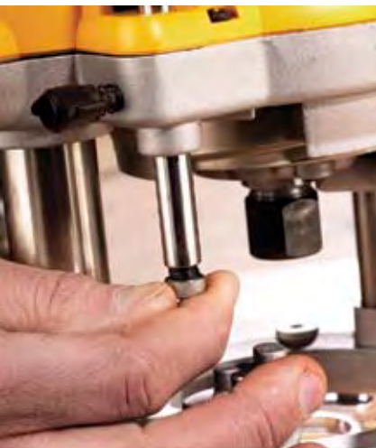
A fine-threaded nut at the end of the plunge rod makes fine-tuning depth settings simple and precise.
