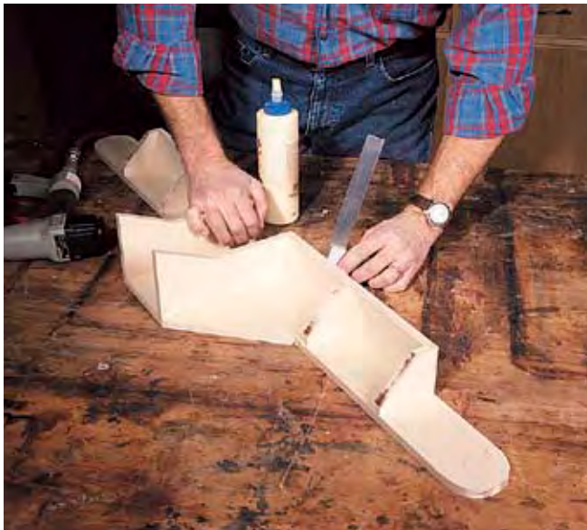
As you assemble the fence, make sure it is square along its length. Be sure and check it again after it is clamped up.
