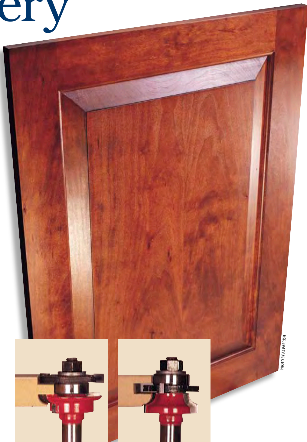
Cutting the cope on the rail's end.
