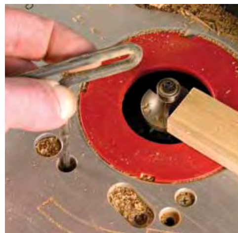
Above-the-table adjustments aren't always as easy as they seem – the hole to reach the screw can fill with debris, and you'll likely need to bend down anyway to see the edge of the bit.
