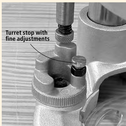
The turret stop is the most common depth stop in plunge routers.
