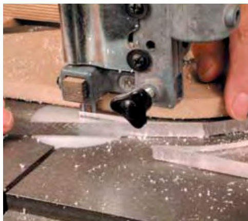
With the template carefully attached to the acrylic, use your band saw to rough-out the shape of the jig itself. Leave a little extra, but don't leave so much that the router won't be able to clean it up easily.
