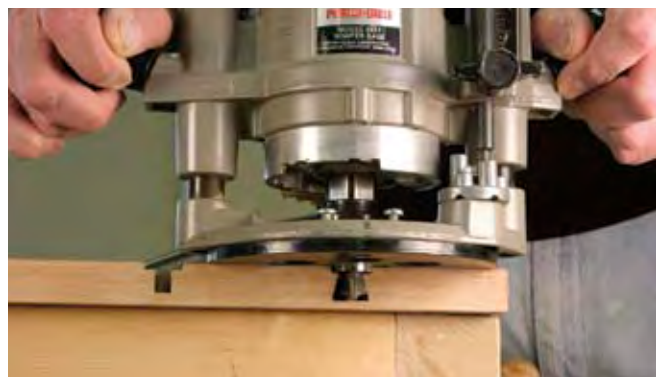
As you slide the router along the edge, the guide bushing and dovetail bit will enter the dado together.
