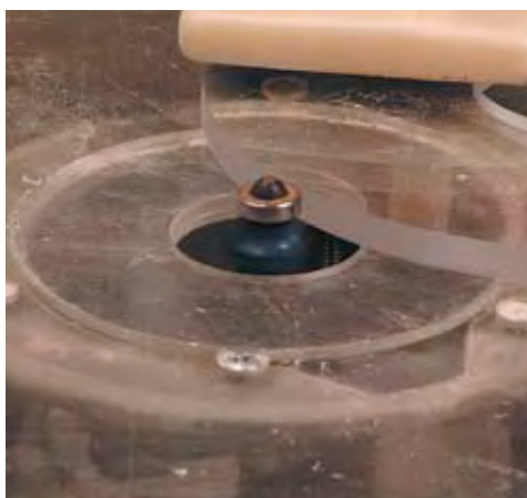
I used a bearing-guided roundover bit to soften the bottom edges of the jigs to protect the wood from scratches and to protect the slightly fragile edges on the jig itself. For the rest of the edges, sandpaper works fine.
