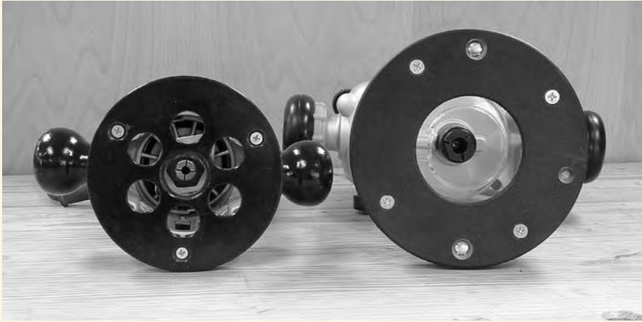
The 1½-hp router (left) has a base opening that is sized for bits appropriate to that size motor. The larger plunge router (right) has a 3-hp motor, appropriately sized for larger bits for panel raising or large profiles. This base has a larger opening to accommodate those bits.
