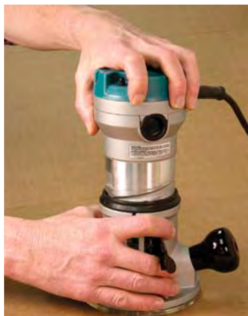
Routers without a fine-thread adjustment on the fixed base have coarse threads on the motor housing. Depth of cut is set by twisting the base in the motor housing.
