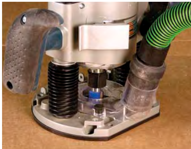
Some routers require a separate attachment for dust collection. The Bosch, shown here, can mount a hose in two different locations.
