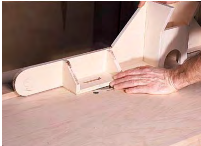
Break in your router table by milling the slots in the fence subfront that will allow the fence faces to adjust into or away from the router bit. Lay out the stop/start lines and plunge cut the slots.
