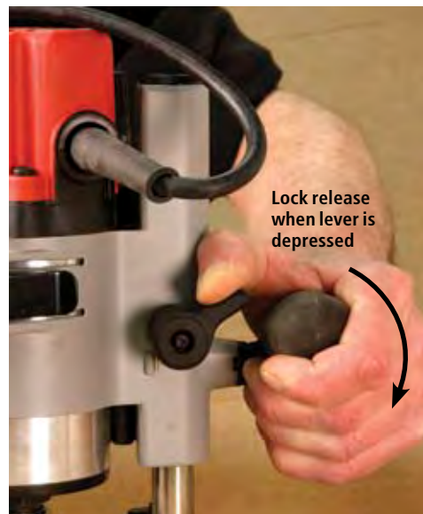
Location and direction of the plunge-release lever is also important. Some, such as the Milwaukee shown here, release when pushed down. Others lock when the lever is pushed down.
