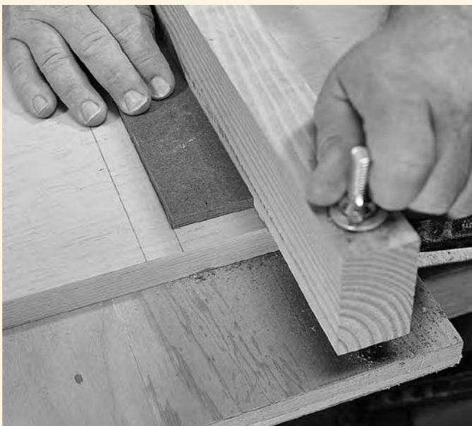
Use the positioning gauge to align the stock underneath the clamping bar. The edge of the gauge indicates the inside edge of the cut.
