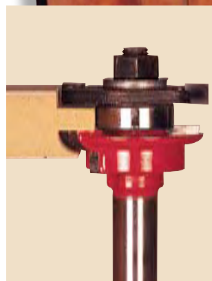
Cutting the cope on the rail's end.
