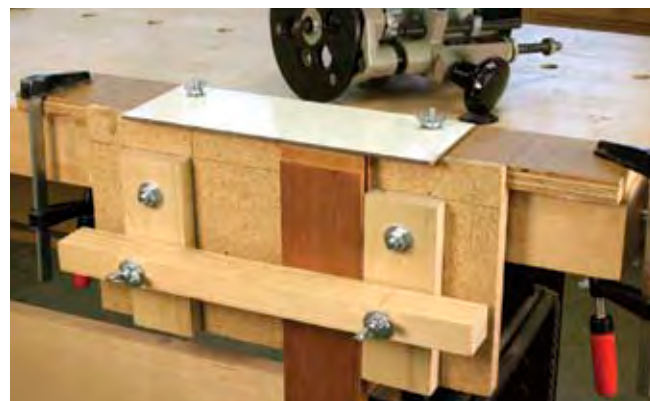
This clamping jig lets me quickly make the tenons without adjusting the router setup. The work is clamped vertically below the Masonite guide piece.
