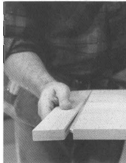
12-15 The corners of the tongue need to be trimmed to fit the groove milled in the breadboard edge. When a test-fit shows a tight joint, I glue and clamp the edges to the panel.
