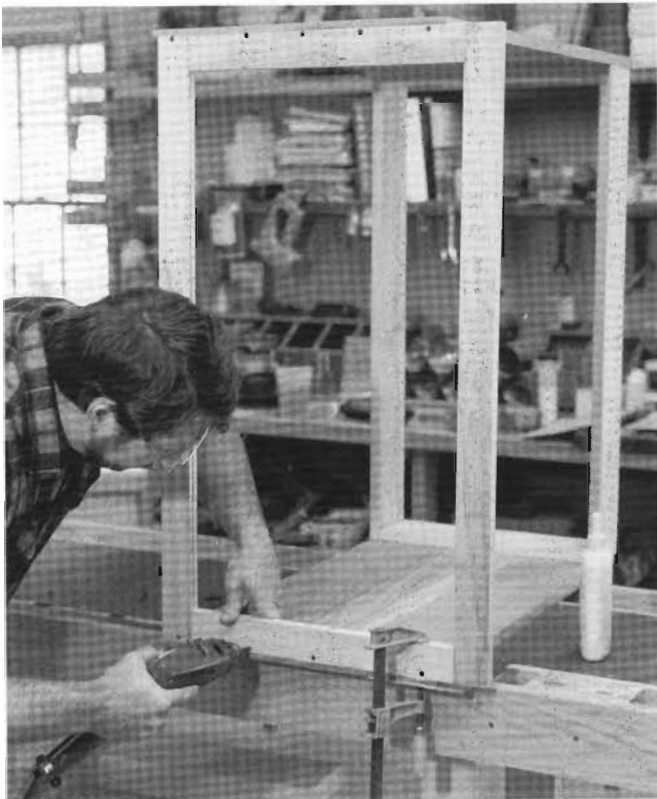
6-2 Glue and screw the top and bottom frames to one side, then the other. The top frame should extend 3 in. beyond the sides' front edges.
