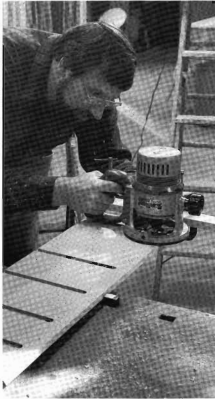
12-9 A wood board, clamped to the desk top, guides the router as I mill stopped dados for the desk compartment dividers.
