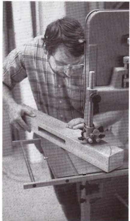
Bandsaw-For curves or straight cuts in extra-thick stock, the bandsaw is best.
