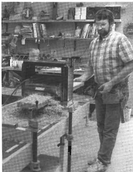
7-1 I use a thickness planer to transform roughsawn cherry boards into smooth, uniformly thick stock.
