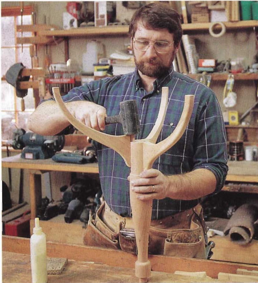
10-9 After spreading glue on the leg dovetails, I coax them into their column grooves with a shot-filled mallet. The fit should be snug, with no need of clamps to keep the joints tight.
