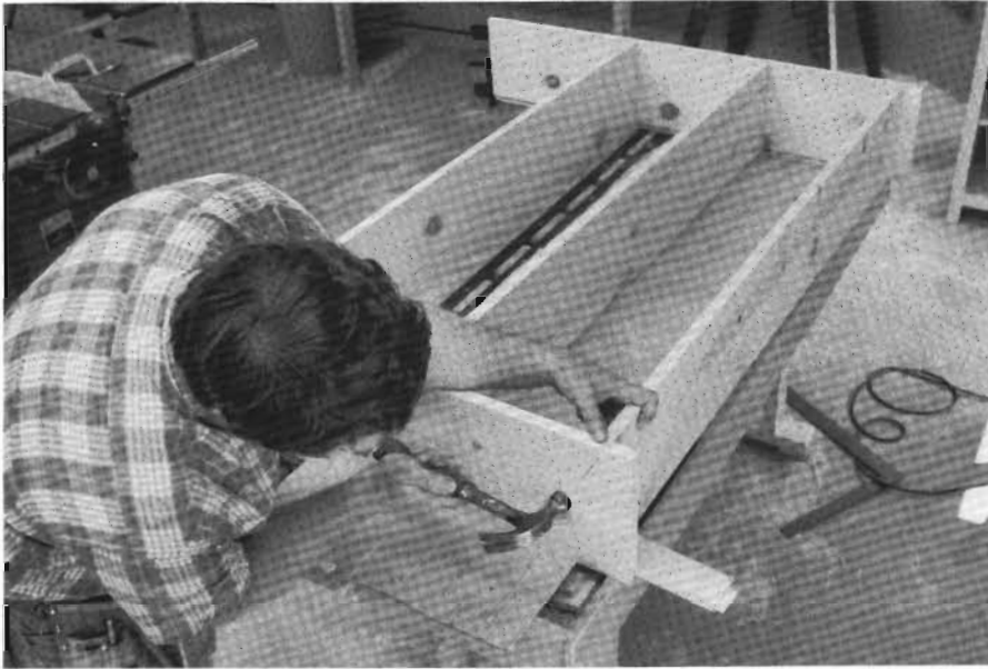
11-12 Assemble the upper cabinet by gluing and nailing shelves into dados milled in the sides.
