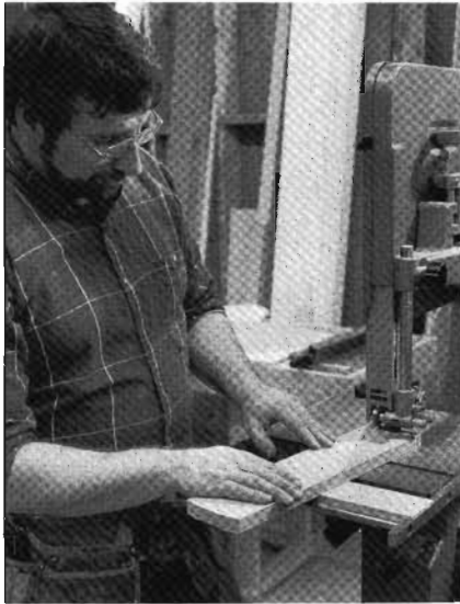
10-10 A simple jig enables me to cut the curved ends of the cleat as well as the round top. First I wedge a block of wood between the guide arms of the bandsaw. Then I drive a screw through the block and into what will become the cleat's center point. The screw acts as a pivot point for cutting the curves.
