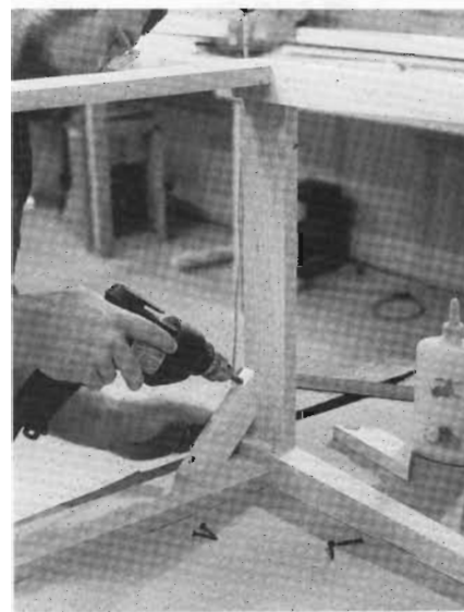
12-6 Strengthen the base by installing pine corner braces just inside the legs. Fasten the braces to the rails with glue and screws.
