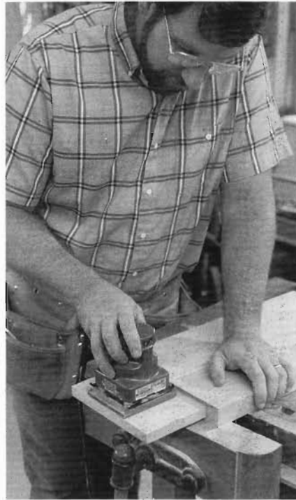
7-10 With an orbital sander and medium-grit paper, I smooth out the tenon cheeks and sides to get a better fit in the mortise.
