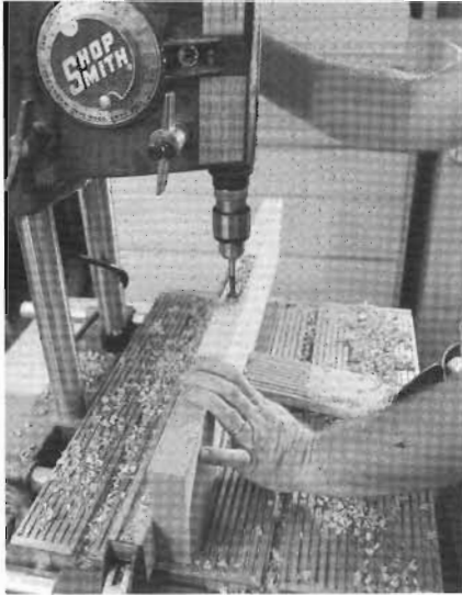
7-6 Use a 3/4-in. Forstner bit to drill out the mortise in each trestle top. A featherboard, clamped to the drill press table, keeps the stock braced firmly against the fence.
