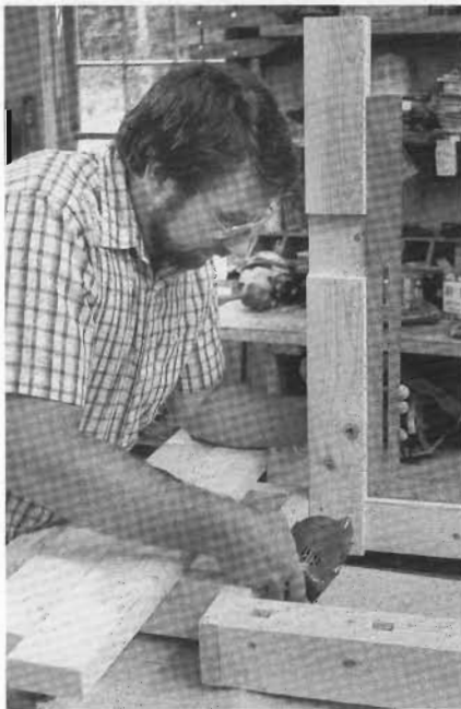
2-5 I hold each leg against the framing square while screwing it to the top frame of the bench.
