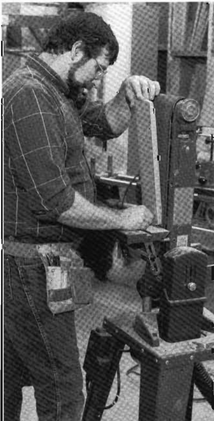
10-11 Using the stationary belt sander, I taper the ends of the cleat.
