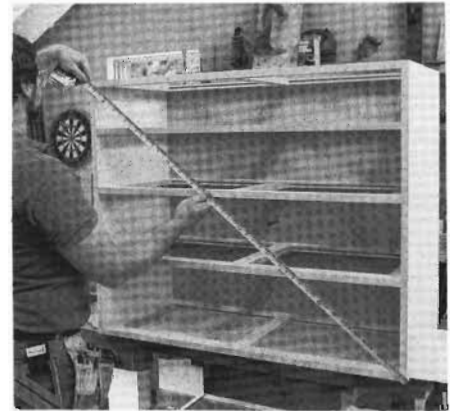
9-7 Nail the back to the top frame only, then check diagonal measurements at the front of the chest to make sure it's square. If necessary, rack the chest slightly until diagonals match. Then finish nailing the back to sides and frame members.
