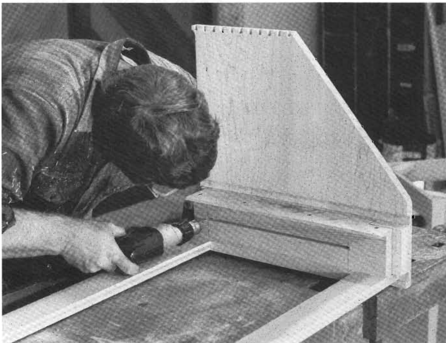
12-8 Install each support by first pushing it into its fully closed position. Then drive a 1 1/4-in. drywall screw through the divider and into the support at the very back of the divider's slot.
