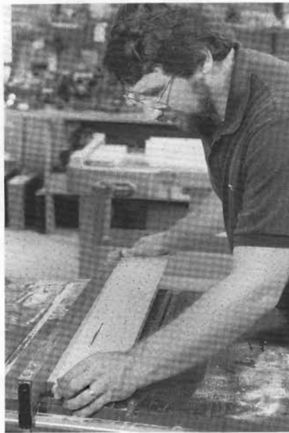
3-7 Carefully lower the rail down over the blade to cut out the bottom edge of the brace. Set the rip fence 1 5/8 in. away from the blade.
