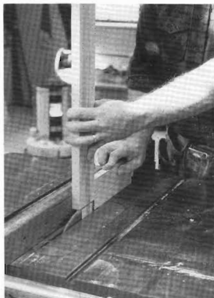
6-16 To cut the haunch in each tenon, move the gauge block 3/8 in. closer to the cutter and raise the cutter 1/2 in. above the table. Hold the rail on edge against the miter gauge as you move the tenon through the cutter.
