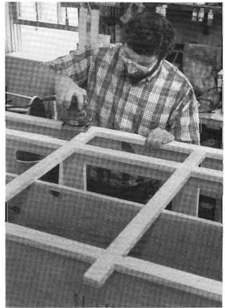
11-7 After gluing and nailing the face frame to the hutch, I go over it with the orbital sander, using medium-grit sandpaper.
