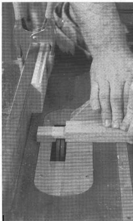
1-10 To mill the tenons, I cut the shoulders first. Starting on one side, I “nibble” away the waste by making several passes over the cutter. Use the same technique on the other side of the tenon.
