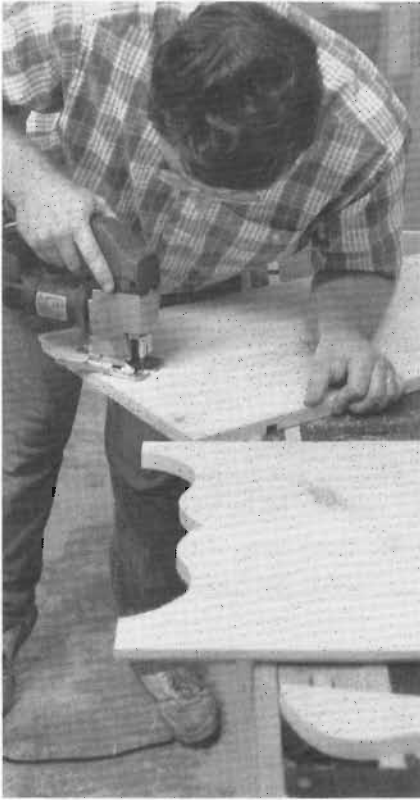
11-2 After tracing a pointed curve pattern onto both sides, I use a portable jigsaw to cut out the legs.
