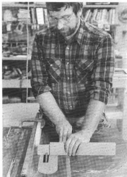
6-15 A wood gauge block, clamped to the rip fence, is positioned to align each rail for its shoulder cut. After making the shoulder cut, make repeated passes with the rail held against the miter gauge to complete each tenon cheek.
