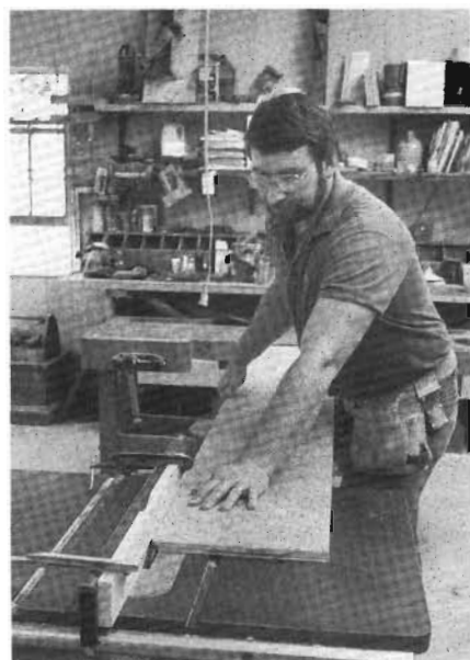
8-3 The sides have to be rabbeted to receive the back. Position the auxiliary fence partway over the cutter, so that only 3/8 in. of cutting width shows. Run the back edge of each side against the fence to mill the rabbet.
