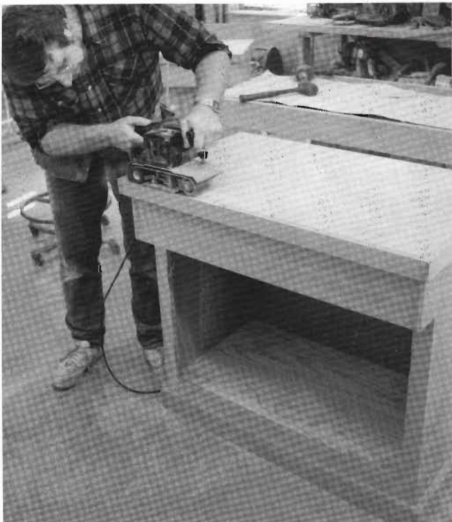
6-9 For best results when laminating, both surfaces to be joined must be smooth. I use a belt sander to smooth the oak trim pieces flush with the particleboard surface.
