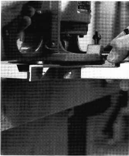
12-16 To mill the angled rabbet along the front's side and top edges, I use a 22-degree laminate-trim bit with its bearing removed and its lower shank filed off. I mill the rabbet in several passes, adjusting both the router fence and the bit depth after each pass.
