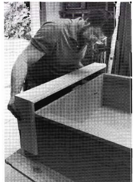
8-7 With corner joints glued and reinforced with blocks, the base slides in place against sides and bottom.
