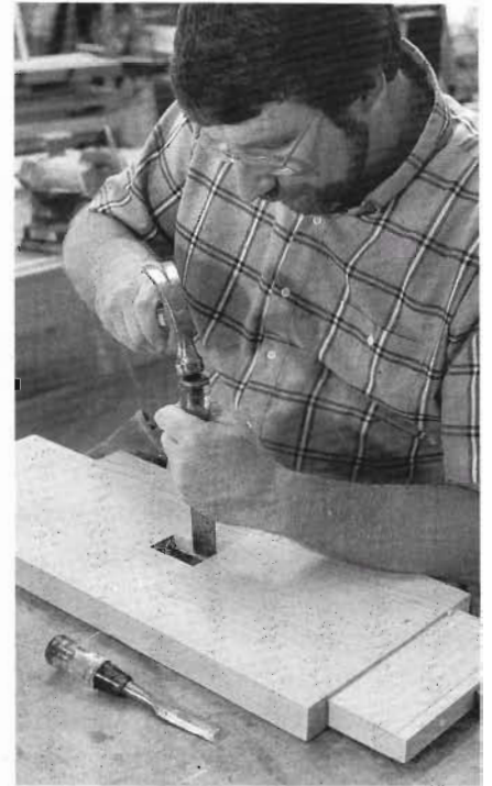
7-11 After drilling out the mortise in each trestle center piece, chisel it square from both sides.
