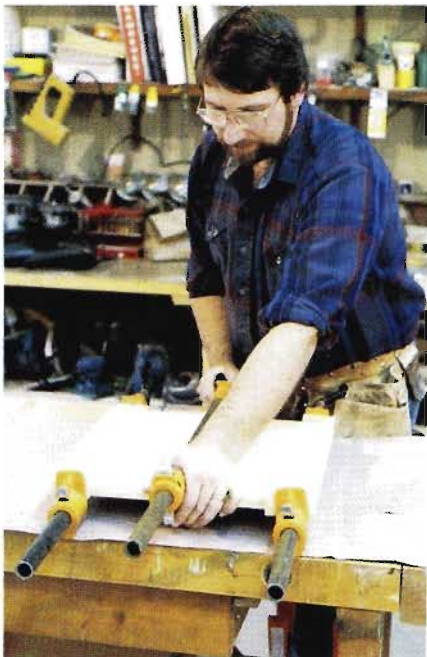
5-1 Use three pipe clamps to glue up the top, two underneath and one on top. Tighten the lower clamps first, using glue squeeze-out to gauge the evenness of clamping pressure.
