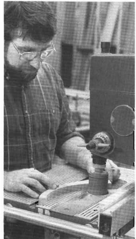
10-4 A drum sander, chucked in the drill press, does a good job of smoothing the edges of each leg.
