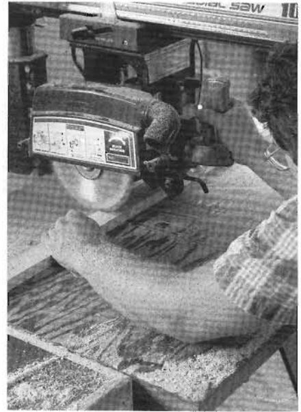
11-6 I cut all the lap joints using the dado head on the radial arm saw.
