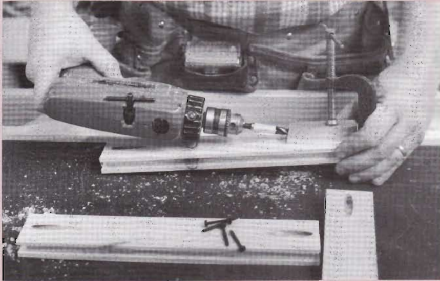
11-9 I use the pocket hole jig to drill the rails of the hutch doors, so that they can be glued and screwed to the stiles. The frame members have already been grooved to accept their panels.
