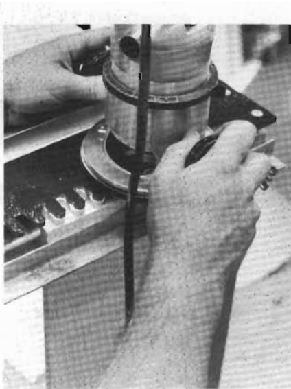
9-8 The base has dovetailed corners that are made using a router, a 3/8-in. dovetail bit and a dovetail jig.
