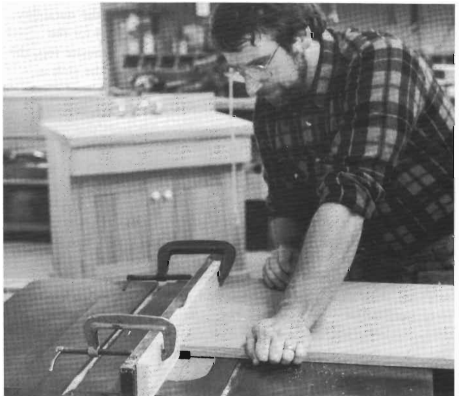
6-1 Rabbet the top edge of each vanity side using a wood auxiliary fence positioned against the dado cutter. Cutter height is 3/8 in. and width is 3/4 in.
