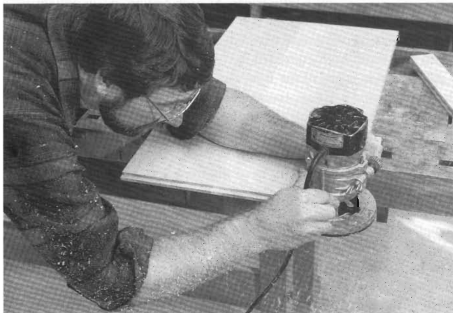
12-14 I mill a tongue along the end-grain edges of the front, using a router and 3/8-in. rabbeting bit. Adjust bit depth so that after 2 passes, a 1/4-in.-thick tongue remains.
