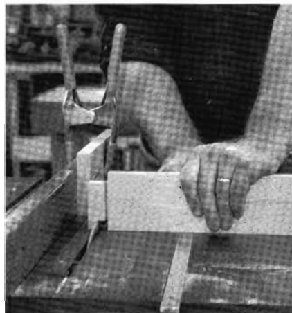
12-3 A wood gauge block (clamped to the rip fence) and the miter gauge align the shoulder cuts for each tenon. Successive passes through the blade remove the waste at the top and bottom of the tenon.
