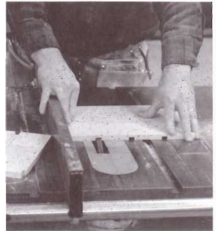
12-10 Dados for the horizontal dividers are cut on the table saw, with the rip fence used as a guide.
