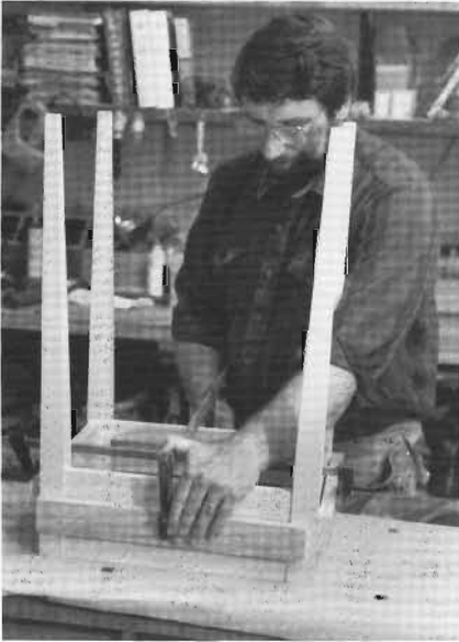
5-10 Dry-fit the rails and legs, and trim mortises or tenons as necessary for a good fit. Then glue and clamp the frame together. Test the rails and legs for squareness. If necessary, install a temporary brace to hold the frame square until the glue cures.
