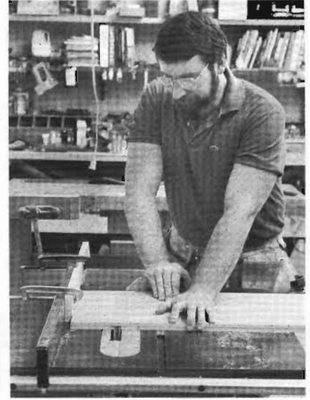
8-2 Dado the sides for the bottom shelf using the miter gauge. Position the auxiliary fence on your side of the cutter, and 4 1/4 in. to the right of it.
