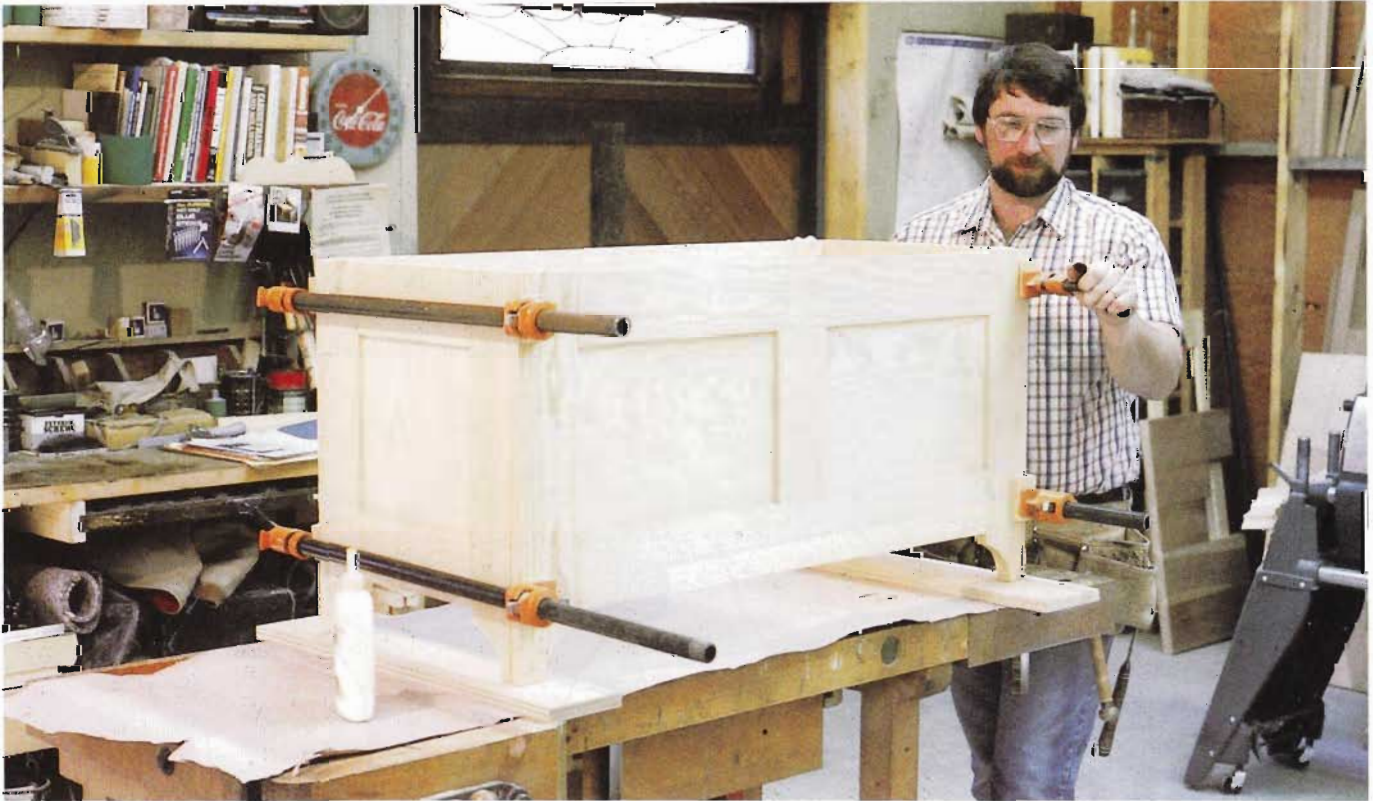
4-14 Glue up each side separately, then assemble the chest by gluing and clamping the tongue-and-groove joints at the corners. Use four clamps, positioned across the side rails. If necessary, brace the chest square until the glue cures.
