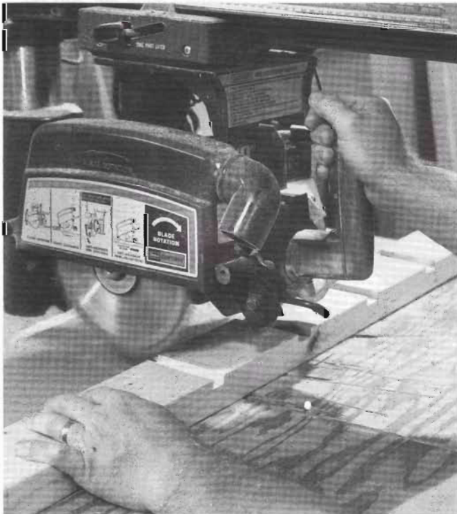
2-2 Dadoes for the bench dog assembly are milled 1 in. wide and 3/8 in. deep, with the radial arm saw adjusted to cut at an 86-degree angle.
