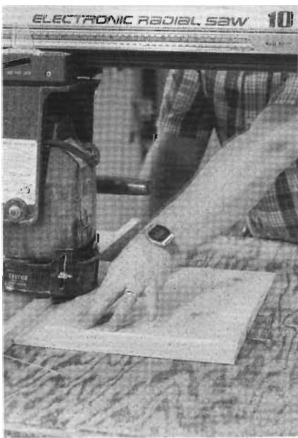
11-8 Raised panels for the doors are milled on the radial arm saw, using a molding head and panel cutters.
