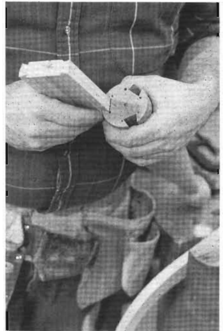
10-8 To avoid the risk of ruining a good leg, it's smart to make your first dovetail in scrap stock to test the set-up of the router table and your joint-making technique.
