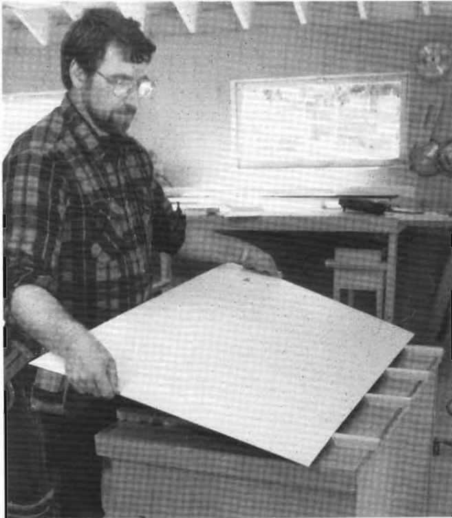
6-11 With thin wood strips positioned across the top, align the laminate and then pull out one strip at a time. Remove the center strips first and force the laminate down firmly against the top.
