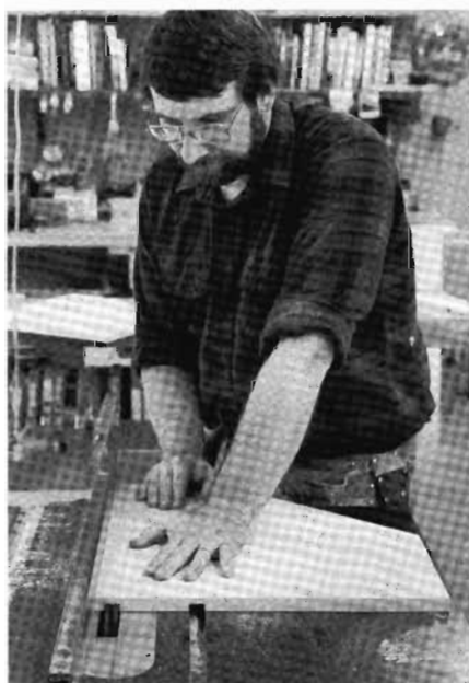
12-7 Use the rip fence as a guide when milling dados in the desk sides. Raise the cutter \frac{3}{8} in. above the table, and adjust its width to \frac{3}{4} in.
