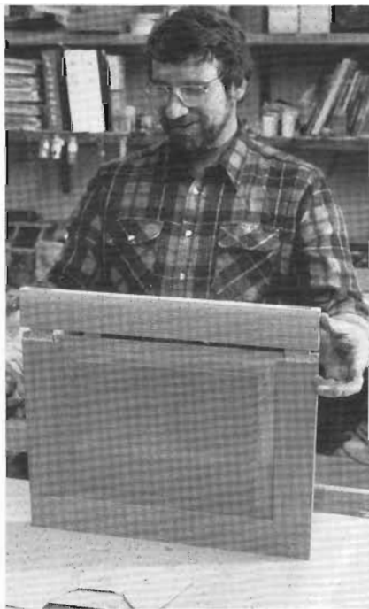
6-18 Slide the panel into its groove after assembling 3 sides of the frame; then glue the final stile in place.
