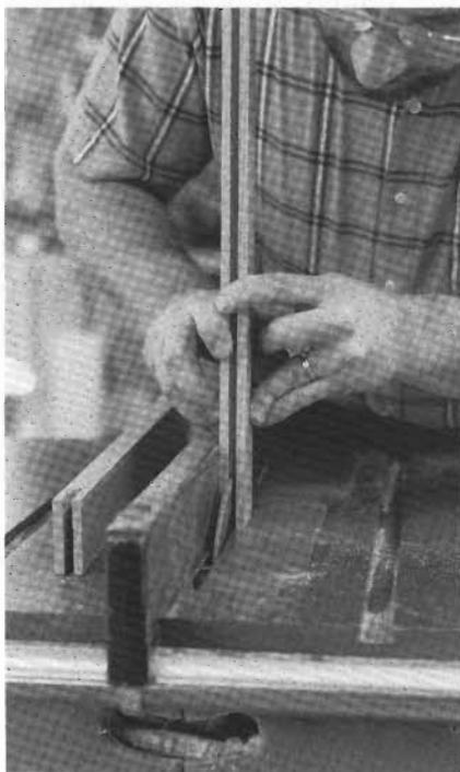
1-9 Mill the mortises by running each stile on its end through the blade, guiding each face of the stock against the rip fence. To make these cuts, you'll need to brace the stock firmly, and work carefully .
