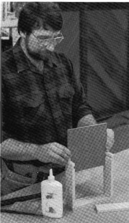
12-12 Each small drawer for inside the desk has its sides dovetailed into its front. After gluing sides and front together, I slide in the bottom before gluing and nailing the back in place.
