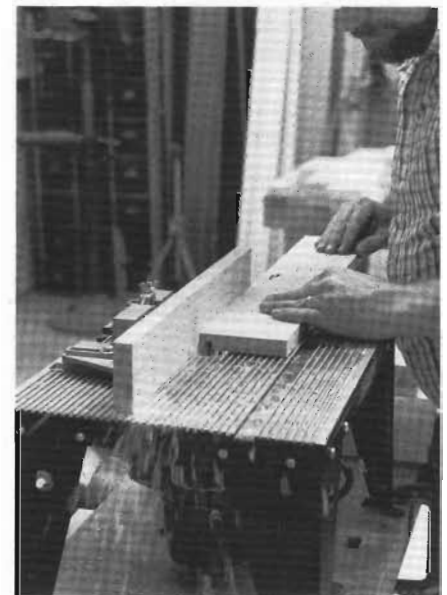
4-3 Groove the front and back stiles on the router table, using a \frac{3}{8} -in. straight bit. Bit height is just over \frac{3}{8} in., and the fence should be set \frac{3}{16} in. away from the bit. Keep the bit and fence set up this way until you've milled all the grooves and all the mortises.
