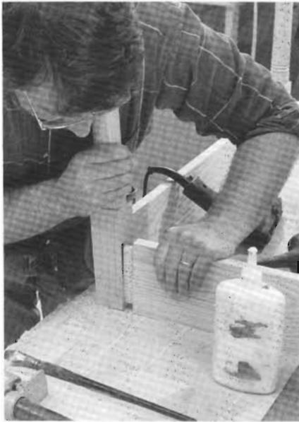
3-9 With a coat of glue applied, the rail tenon gets fitted into its mortise.
