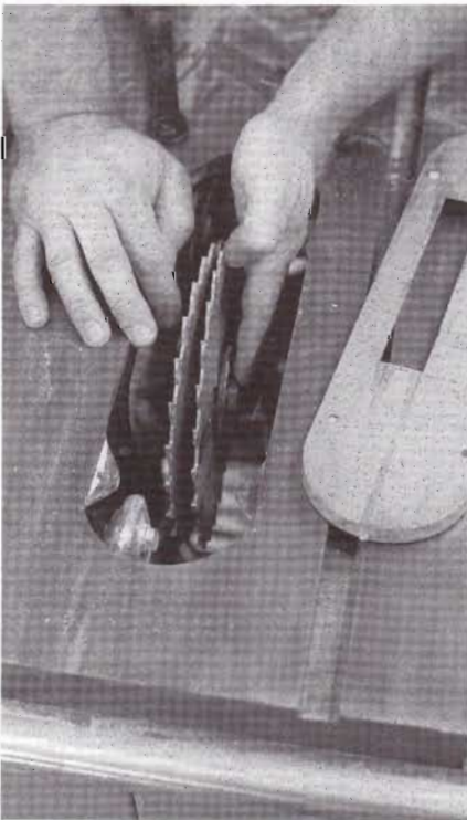
Dado head—This adjustable, twin-bladed dado head mounts on the arbor of the table saw.
