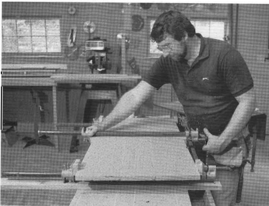
3-12 The table top is glued up from 3 ash boards. Pipe clamps alternate over and under the stock to help keep clamping pressure even.
