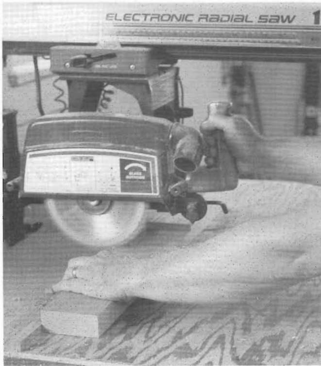
7-2 Mill the broad dado in each foot piece by making multiple passes with the dado head. Adjust the cutter for maximum width of cut. Depth of cut should be 1/2 in.
