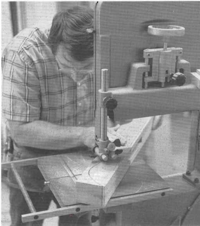
7-4 Cut out the curved feet on the bandsaw. To cut curves in hardwood this thick, you'll need a sharp, 1/4-in. blade.
