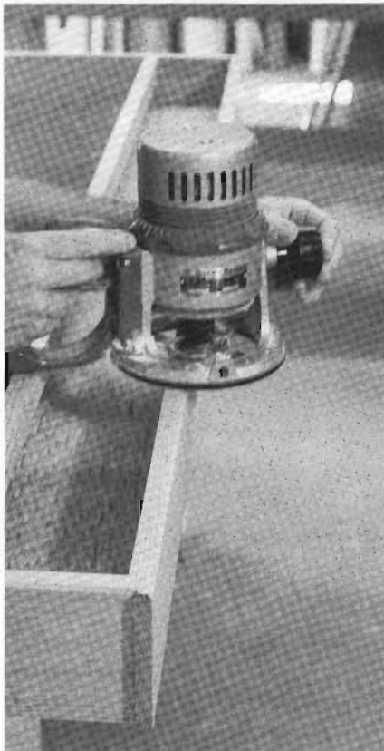
Router—With a router and a good selection of router bits, many different edge treatments are possible. Here I'm chamfering the top edge of the oak board that forms the back of the workbench.
