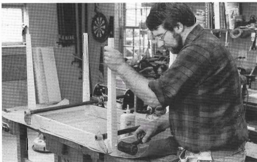
12-5 After gluing and clamping the rails to the legs, I drill 2 holes through each joint and peg the tenons in their mortises with a pair of 1/4-in. dowels. Coat the dowels with glue before driving them, and let them protrude above the surface so that they can be sanded flush after the glue dries.
