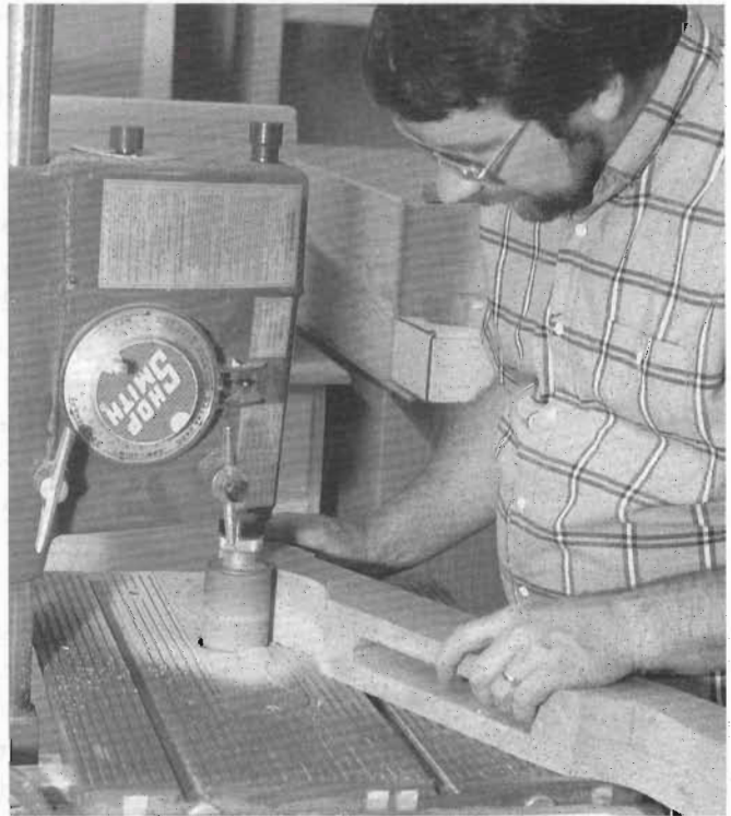
7-5 A drum sander, chucked in a drill press, does a good job of removing saw marks and irregularities after curved cuts are made.
