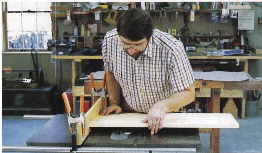
9-4 Stopped dados are cut in two steps. First, the sides are dadoed on the table saw, using the rip fence as a guide. Because the dado must stop shy of the front edge, the side has to be lowered over the cutter. Dado width is 3/4 in.; depth of cut is 3/8 in.
