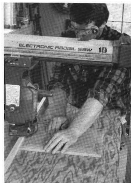
6-17 After cutting the 3/4-in.-thick oak panels to size, I raise the edges on the radial arm saw, using a molding head and panel cutters. Mill the edges in stages, lowering the cutters until edge thickness is 3/8 in.
