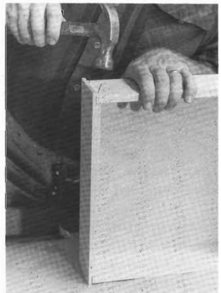
5-12 Glue the front to the sides and nail through the sides into the shoulders of the rabbets, using 1 \frac{1}{4} -in. brads.
