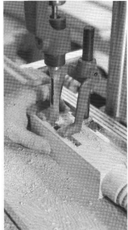
3-2 A hollow-chisel mortising bit makes quick work of milling mortises in the legs. A fence keeps the leg aligned while repeated plunge-cuts are made with the bit.
