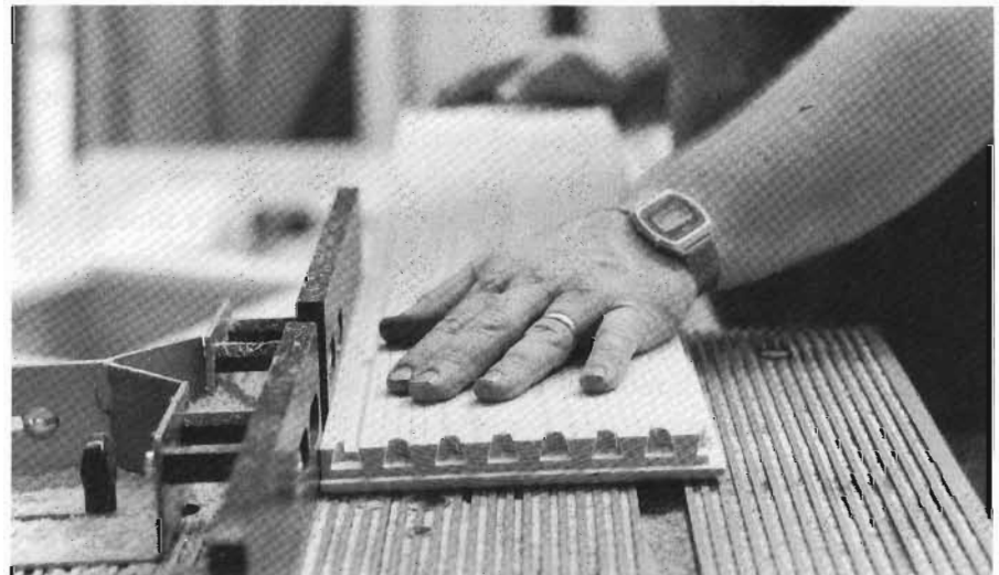
9-16 The drawer fronts have been rabbeted along top and side edges, and dovetailed to receive sides. The final step before assembly is to round over the front edges. Use a 1/4-in. roundover bit, set up in the router table. After adjusting bit height and fence position, mill the short edges of each front first, then the long edges.
