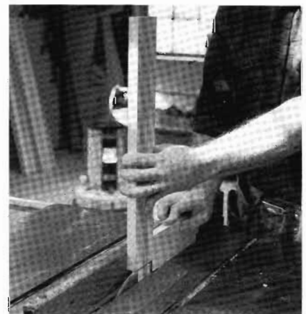
12-4 To complete the tenon, make a pair of cheek cuts with the rail held on end. Use the rip fence to guide first one face of the rail, then the other, through the blade. For safety, push the stock with a scrap piece of wood.
