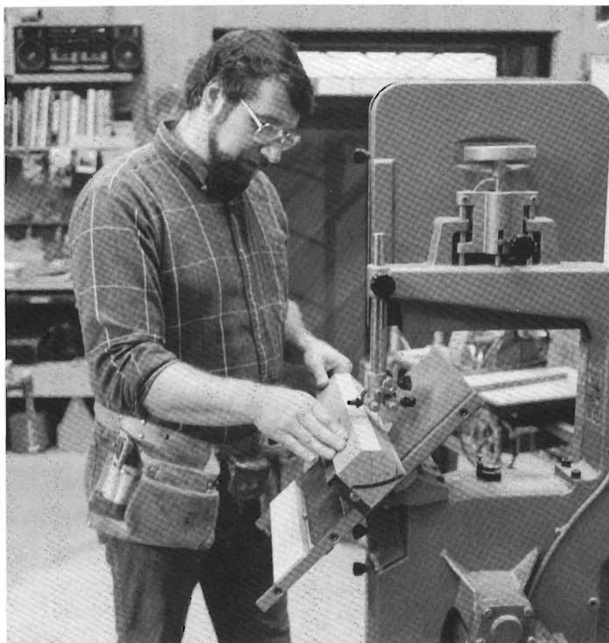
10-1 I use the bandsaw to trim off the corners of the cherry blank for the turned column. Sawing out these 4 triangular sections will save time on the lathe.
