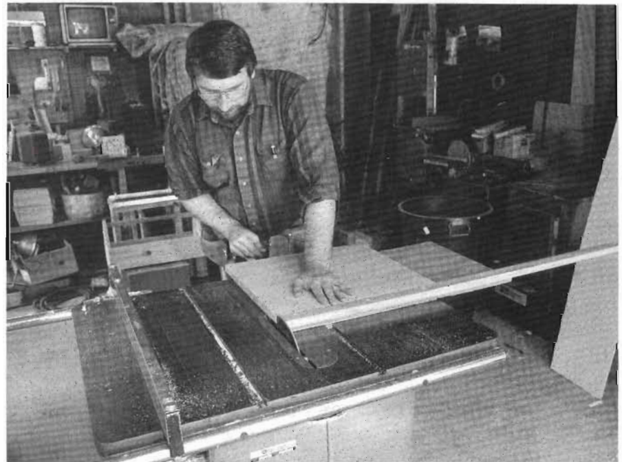
Panel cutter—This is a useful jig for squaring up large panels on the table saw.
