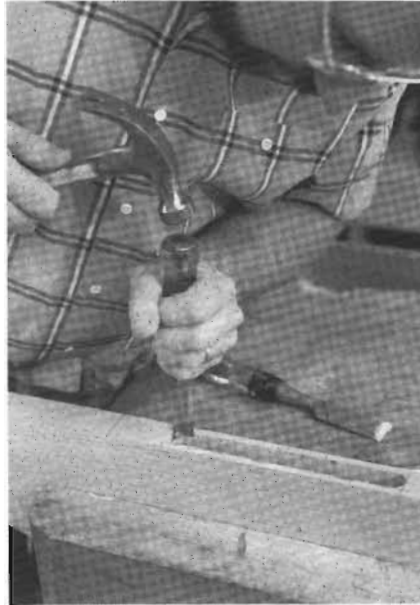
7-7 With a sharp chisel, square up the edges of the mortises and smooth the inside of the joint.
