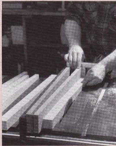
5-4 Make the tapered cut by carefully moving the jig and the workpiece together through the saw blade. The straight side of the jig rides against the rip fence; the adjustable side holds the workpiece.
