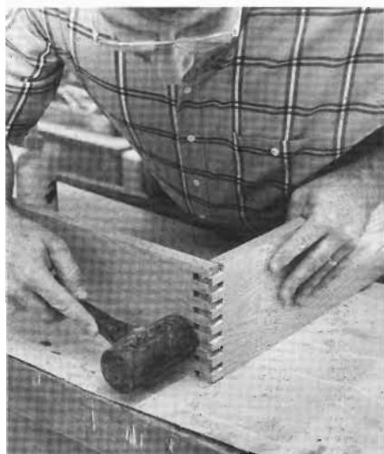
1-6 After spreading glue on the fingers of the joint, tap both pieces together with a shot-filled mallet.
