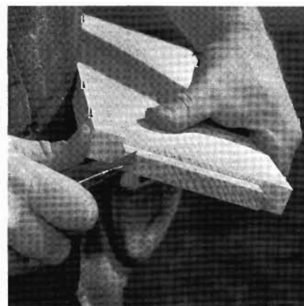
5-9 With a sharp utility knife, trim a rough curve into the top and bottom of each tenon. This should give the tenon a snug fit in its mortise, which is curved top and bottom from the router bit used to cut it.
