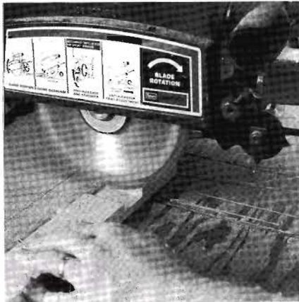
8-5 Lap joints in the face frame's stiles and rail can be cut on the radial arm saw, using a dado cutter. Set the dado for maximum width of cut and 3/8-in. depth of cut. Then make repeated passes to complete each joint.
