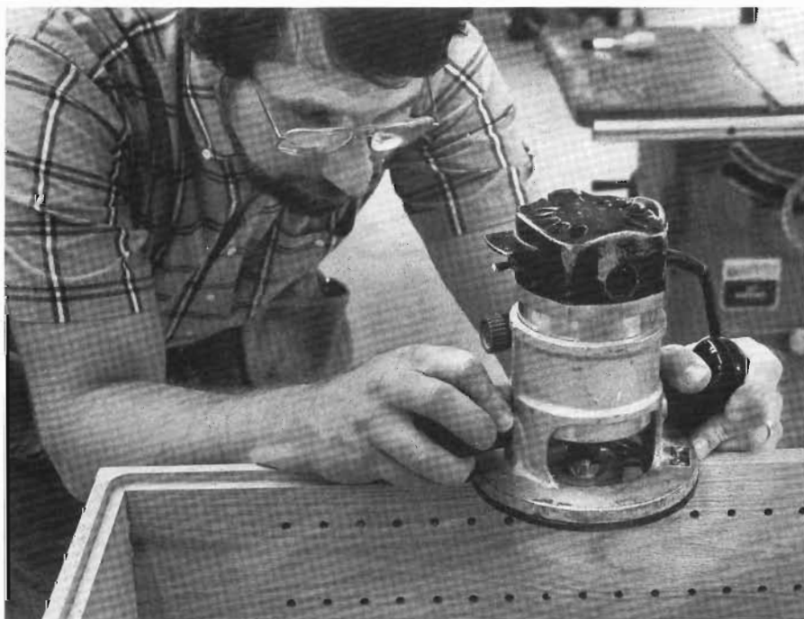
1-7 With a 3/8-in. rabbeting bit in the router, I rabbet the back edge of the box to receive the plywood back. The curved corners should be chiseled square before cutting and installing the back.
