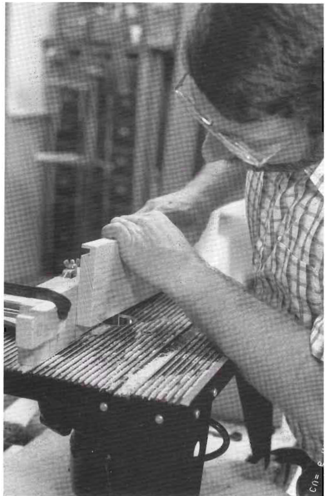
4-5 To cut the lower mortises, stiles must be firmly lowered down over the bit. The cut begins at the lower end of the mortise, and ends 3 in. later, when the bottom edge of the stile butts against a stop block clamped to the rip fence.
