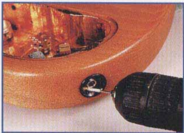
16 Installing the output jack plate
