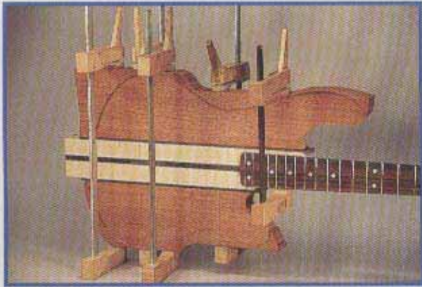
36 Gluing second body wing
