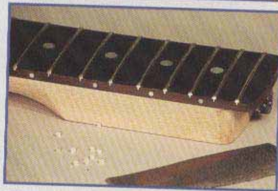
32 Side inlays in place
