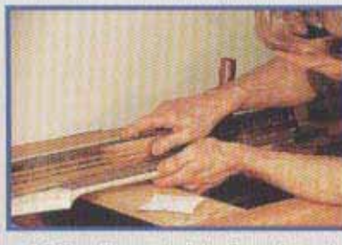
18 Sanding arch into fingerboard with full-length sanding block
