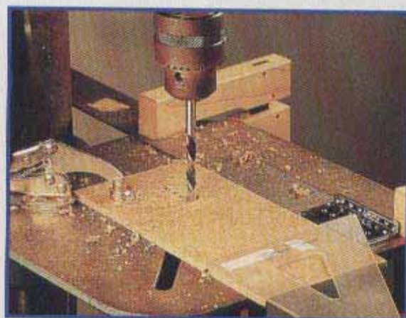
32 Making a jig for aligning ferrule holes
