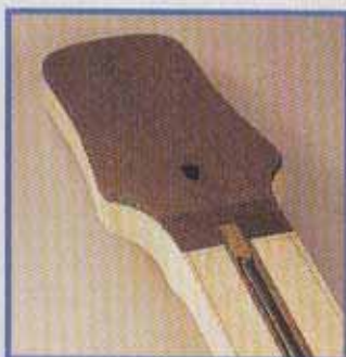
17 Headstock faceplate trimmed to neck surface
