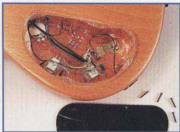
19 Pickup leads connected
