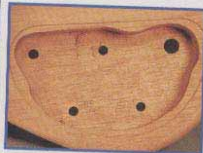
26 Electronics cavity interior (right)
