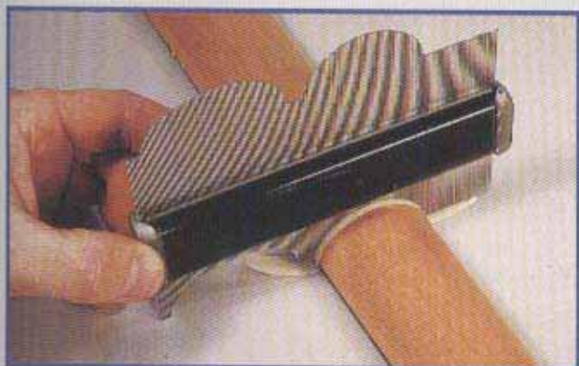
4 A feeler gauge can make a cross section of a neck (mask the neck to avoid scratches). Trace the shape from the gauge onto paper or cardboard, and cut this out to use as a template.
