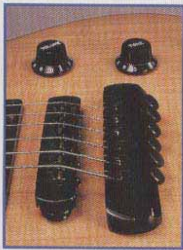
13 Variation of Tune-o-matic bridge. Stop tailpiece is equipped with fine tuners, and the bridge saddles are small rollers, allowing adjustment of the string spacing for use with a wide range of pickups. Roller saddles have a slightly detrimental affect on tone.
