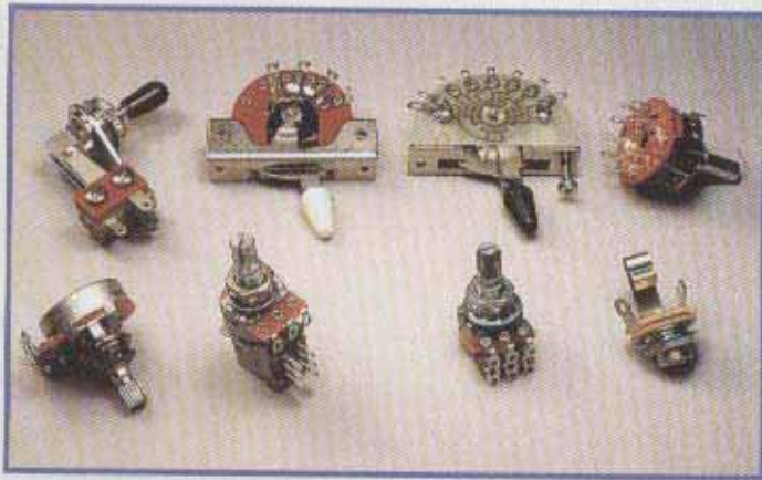
10 Electronics components Top, L to R Three-position switch, 3-pickup SG style Standard Stratocaster 5-position switch Specialty 5-position Rotary switch Bottom, L to R Potentiometer Potentiometer with DPDT push-pull switch Blend potentiometer Output jack
