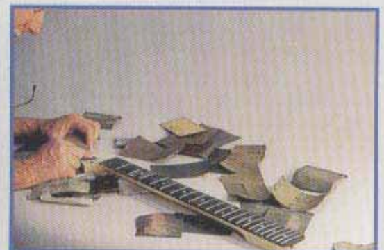
2 Sanding around edges with sandpaper stretched between fingers
