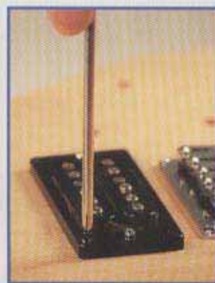
10 (right) Attaching pickups in body
