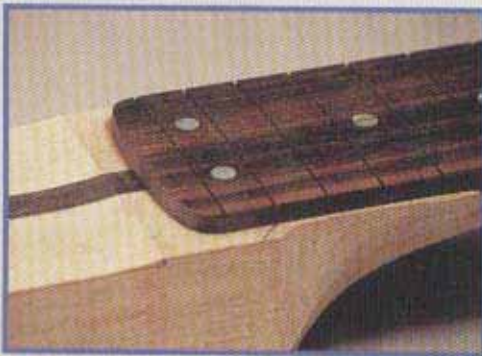
27 Fingerboard rounded at body before gluing
