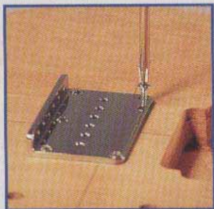
28 Screwing the bridge to the body
