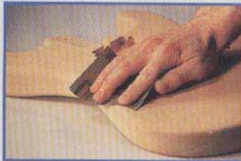
2 Sanding around edges with sandpaper stretched between fingers
