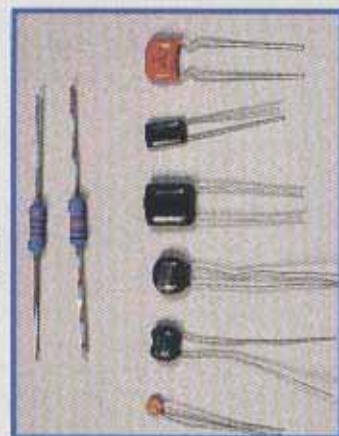
11 Resistors (left), Capacitors (right)
