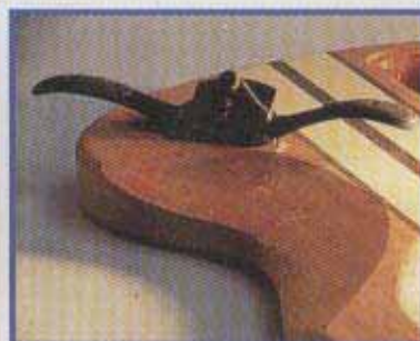
49 Carving body contour with a spokeshave
