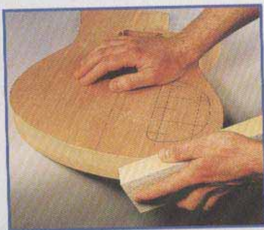
16 Sanding the sides to final shape
