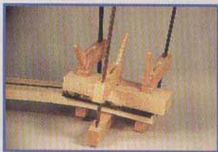
15 (above) Gluing headstock faceplate
