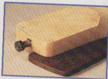
11 End of neck is sanded before fingerboard is attached
