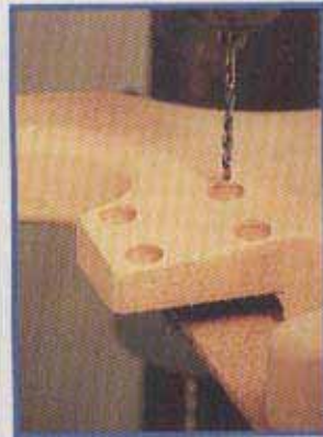
40 Drilling neck screw holes
