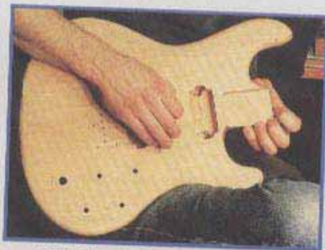
49 Testing the contours in playing position
