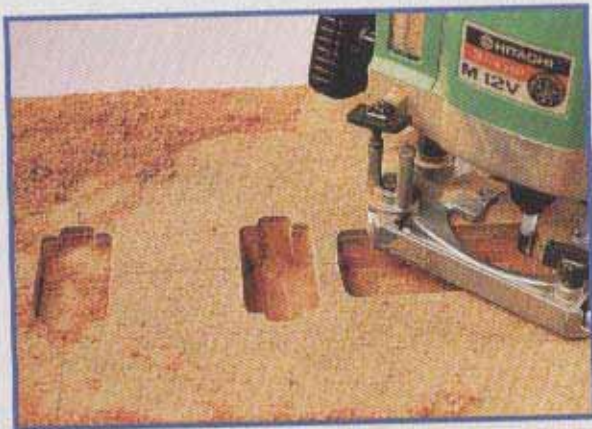
13 Routing the cavities
