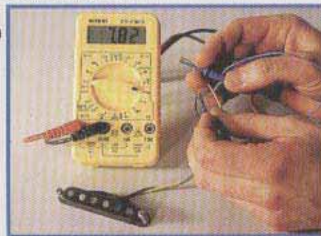
6 Telecaster neck pickup, with 7.82 kilohms coil resistance
