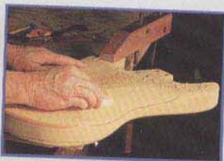
47 Sanding the back contour smooth with an eraser as a sanding block. Flex the eraser slightly for concave curves.
