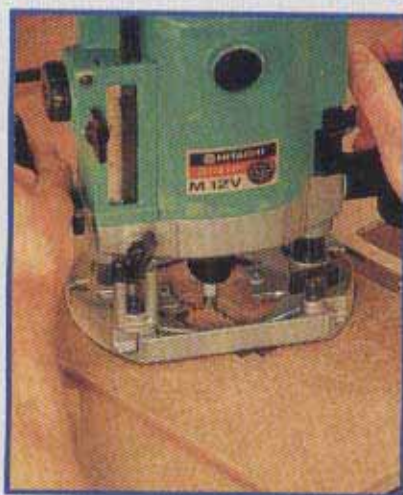
9 (lower left) Preparing to rout the second pickup hole in the Master Template
