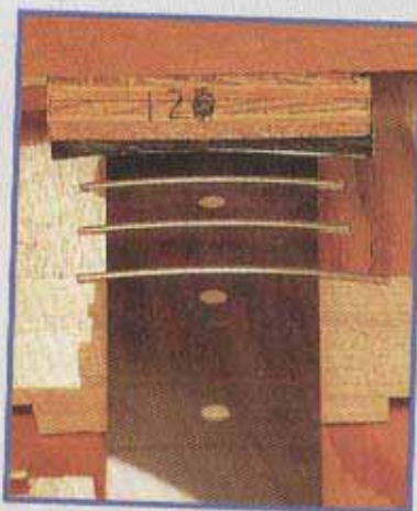
23 Fret press. This one is made with milled phenolic blocks. Closer side presses fret, far side (with felt) rides on fingerboard
