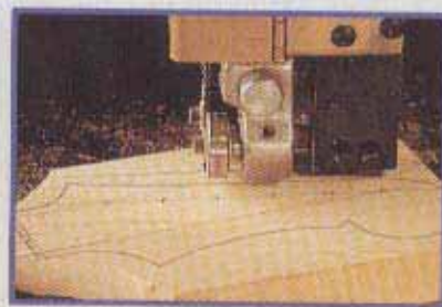
19 Cutting straight side for tuner drilling jig
