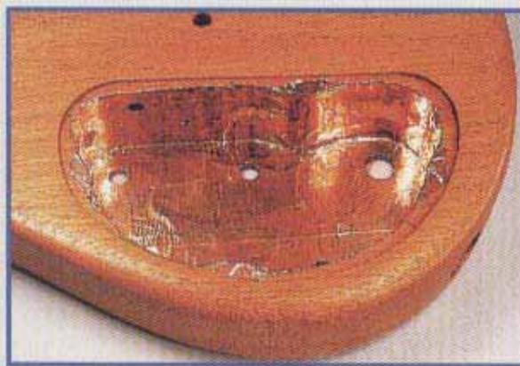
14 Copper shielding tape in electronics cavity
