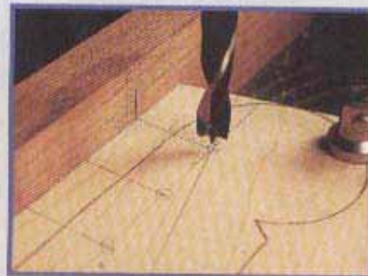
21 Aligning headstock to marked fence
