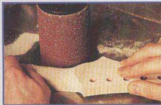
29 Shaping around volute with oscillating spindle sander
