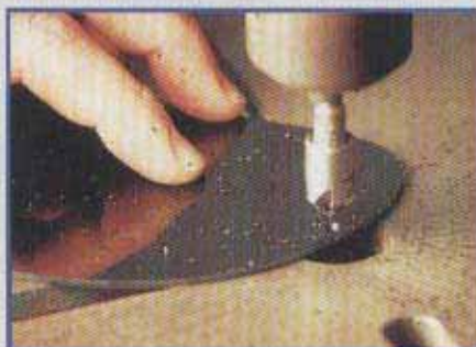
14 (middle right) Screw positions marked for drilling
