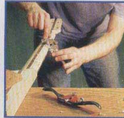
28 Fingerboard alignment tacks
