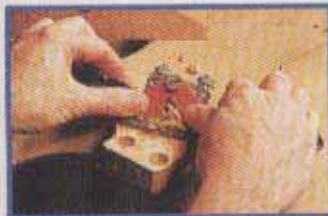
43, 44 Carving the heel chamfer
