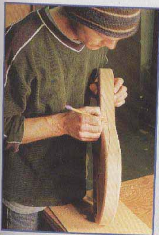
45 Marking the back contour
