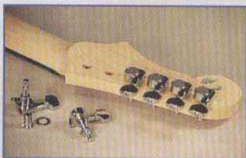
5 Aligning tuners in holes
