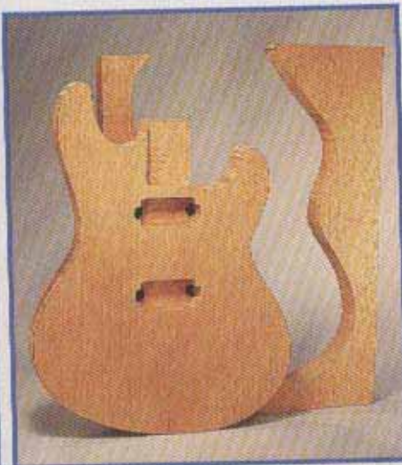
15 The body completely cut out
