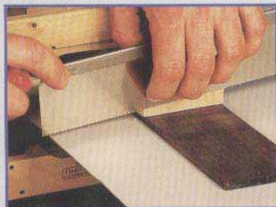
4 Sawing fret slots with fence
