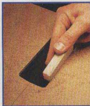
6 Sanding the neck pocket to its final shape using small sanding block to keep lines straight
