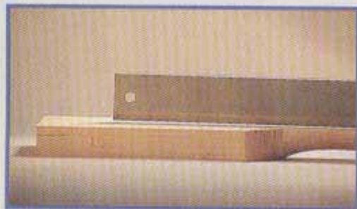
7 (right) Neck piece was flat before carving, bowed after
