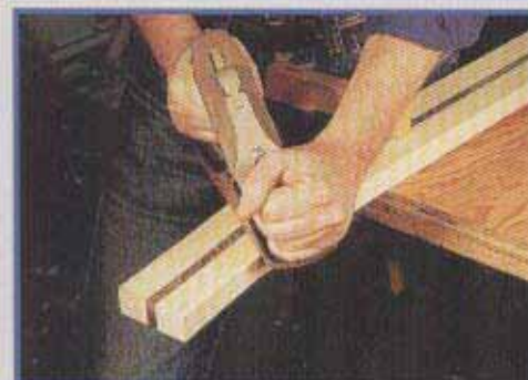
11 (left) Locating truss rod position
