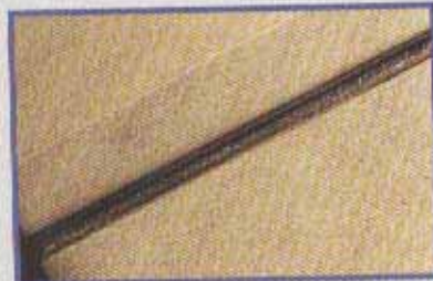
30 (below right) Recrowning fret with fret file
