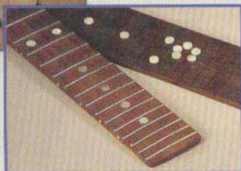
6 Inlay positions on fingerboard
