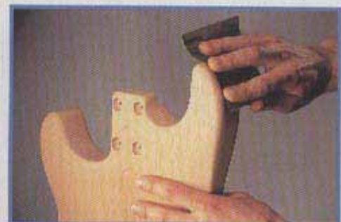
3 Sanding curves in upper horn
