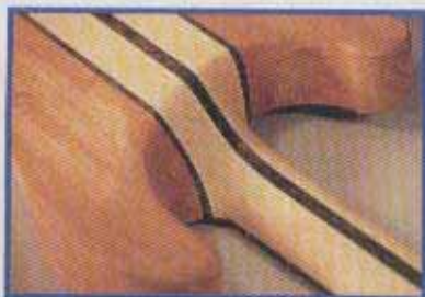
50 Sanded heel and body contour
