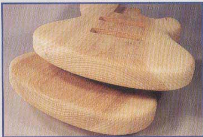
1 One-piece bodies from same board with opposite grain orientation
