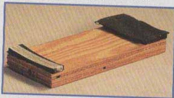
23 Fret press. This one is made with milled phenolic blocks. Closer side presses fret, far side (with felt) rides on fingerboard
