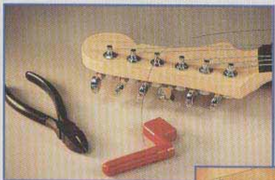
7 Stringing for nut slotting
