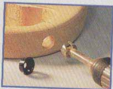
50 Output jack hole and Forstner bit
