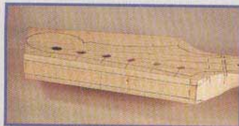
21 Aligning headstock to marked fence
