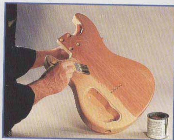
7 Applying first sealer coat
