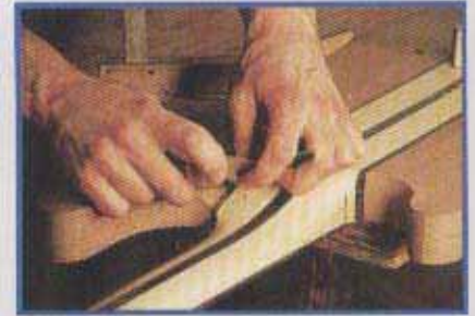
39 Carving heel into body wings
