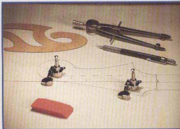
26 Laying out the headstock
