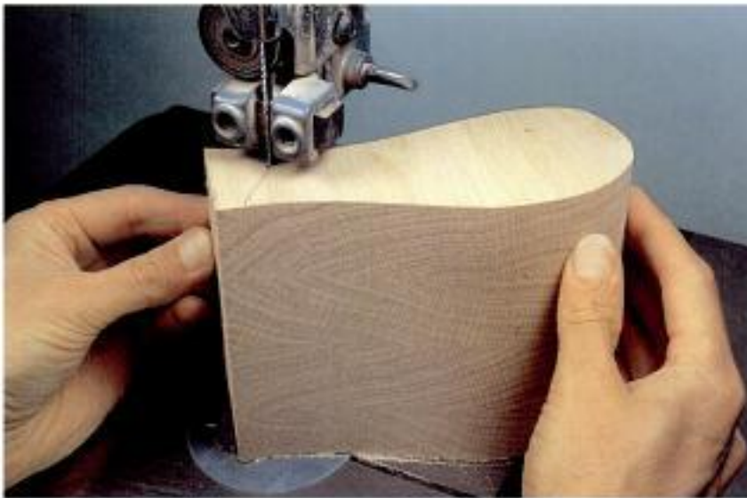
Photo 3-7 Before you begin cutting apart the drawer blocks, and while your guard is still at the proper height, cut the waste off any drawers whose pattern requires it.
