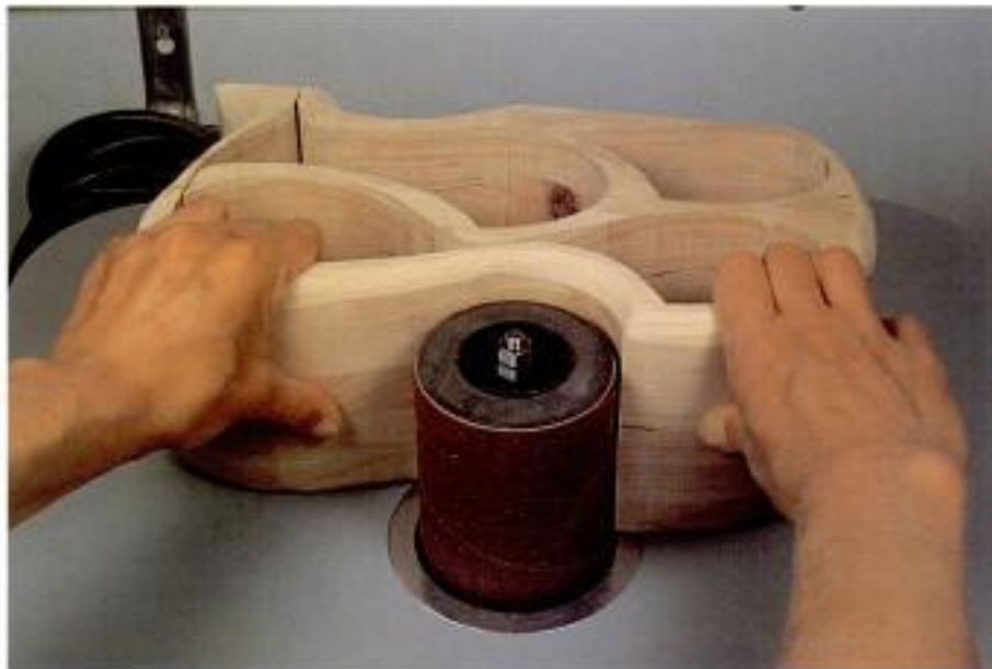
Photo 4-4 Another option is to sand the inner curves on the oscillating drum sander.
