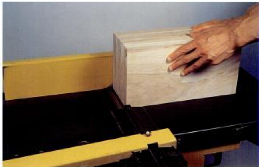
Photo 2-14 Jointing is the easiest way to square one side of the block.
