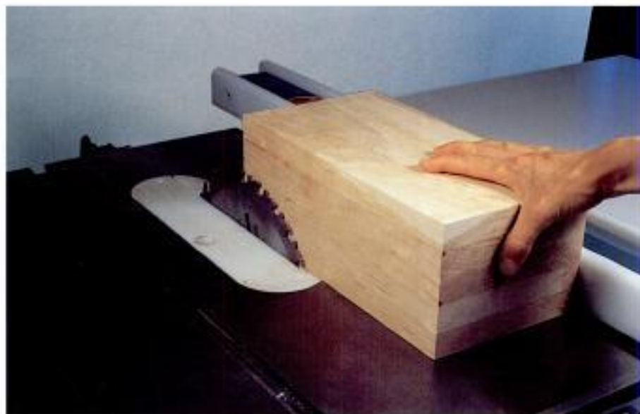
Photo 2-15 If you use the table saw for squaring, be sure not to rip more than a blade's width off the block.
