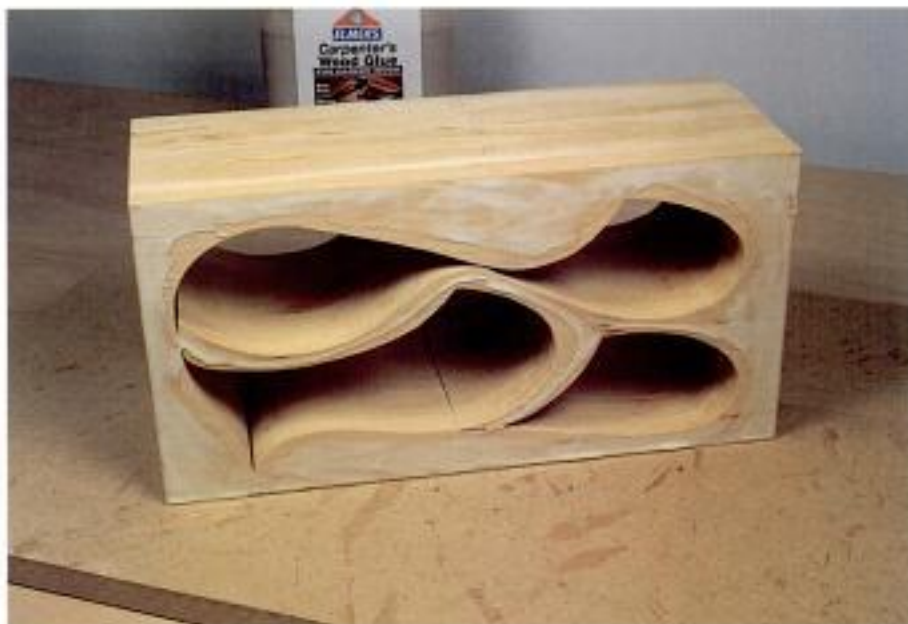
Photo 3-14 Avoid spreading too much glue right to the edges of the drawer cavities. Otherwise, you'll have to chip the dried glue off the insides of the cavities.
