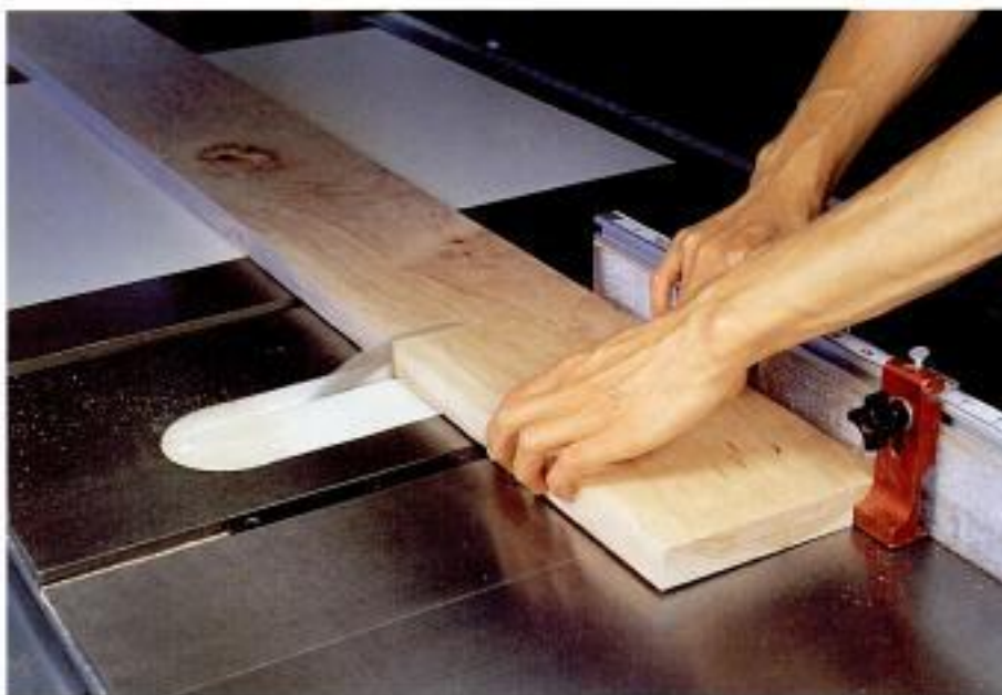
Photo 2-9 Keep the pieces in order as you crosscut the board into five even sections.
