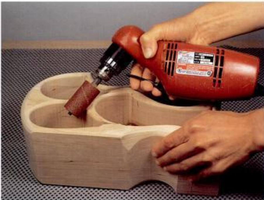
Photo 4-13 As an option, or if you don't have a router, you can roughly round over the openings with a coarse sanding drum in your portable drill. 80-grit on the palm sander will quickly smooth it out.
