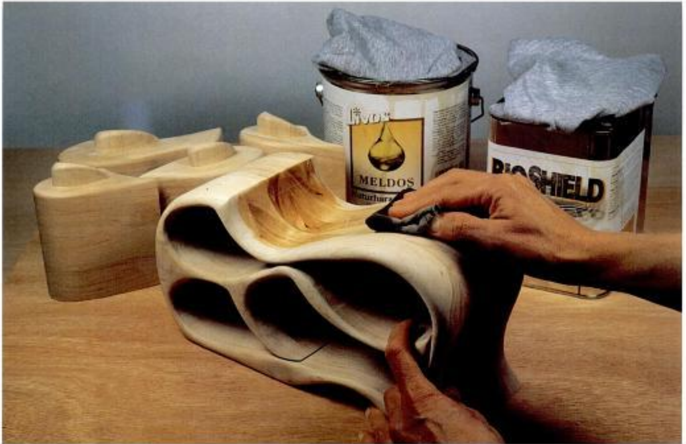
Photo 5-1 For best results, give the sealer coat an extra day to dry.
