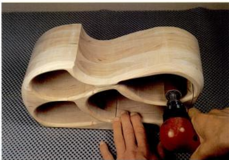
Photo 4-15 If you didn't use the oscillating drum sander previously, sand the drawer cavities with your drums and portable drill.
