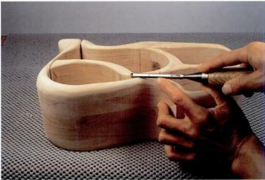
Photo 4-19 A sharp chisel makes easy work of rounding over in the saw kerfs.
