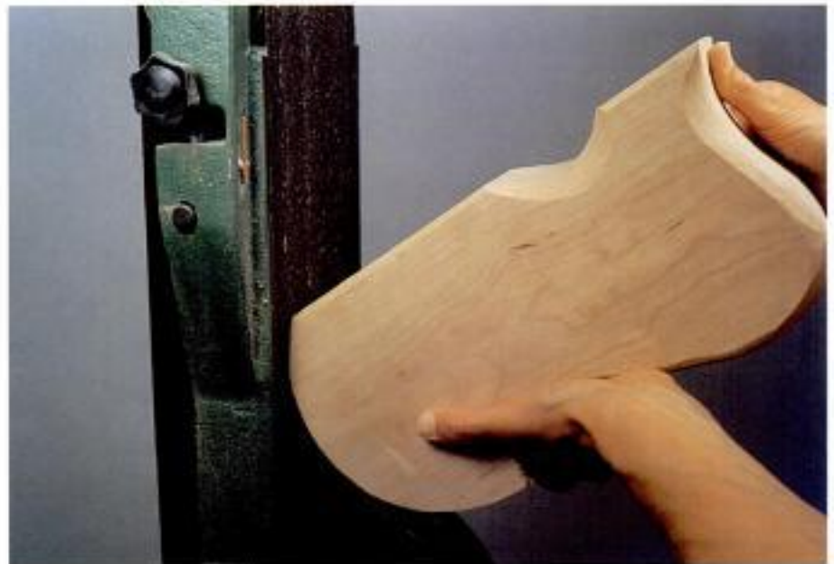
Photo 4-11 Hold the box or drawers tightly as you sand out the cross-grained lines. Use an upward motion against the face of the 120-grit belt. Repeat this process using the 180-grit belt to lessen your palm sanding later.
