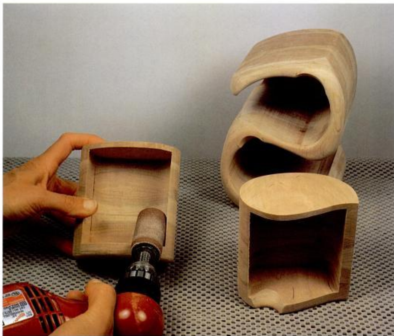
Photo 1-3 An angle drill is the easiest on your wrist for freehand shaping techniques.
