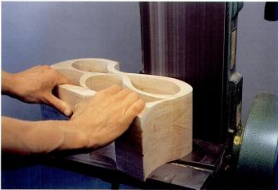
Photo 4-2 The outer curves of the box can be quickly smoothed with a 60- or 80-grit belt.
