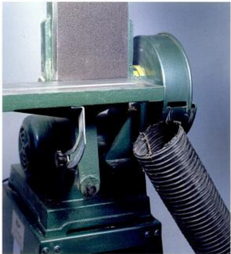
Photo 4-1 Shaping with a belt sander creates great clouds of dust. You can cut down on the dust by simply hooking your dust collector hose beside or beneath the table while using the sander in the vertical position.
