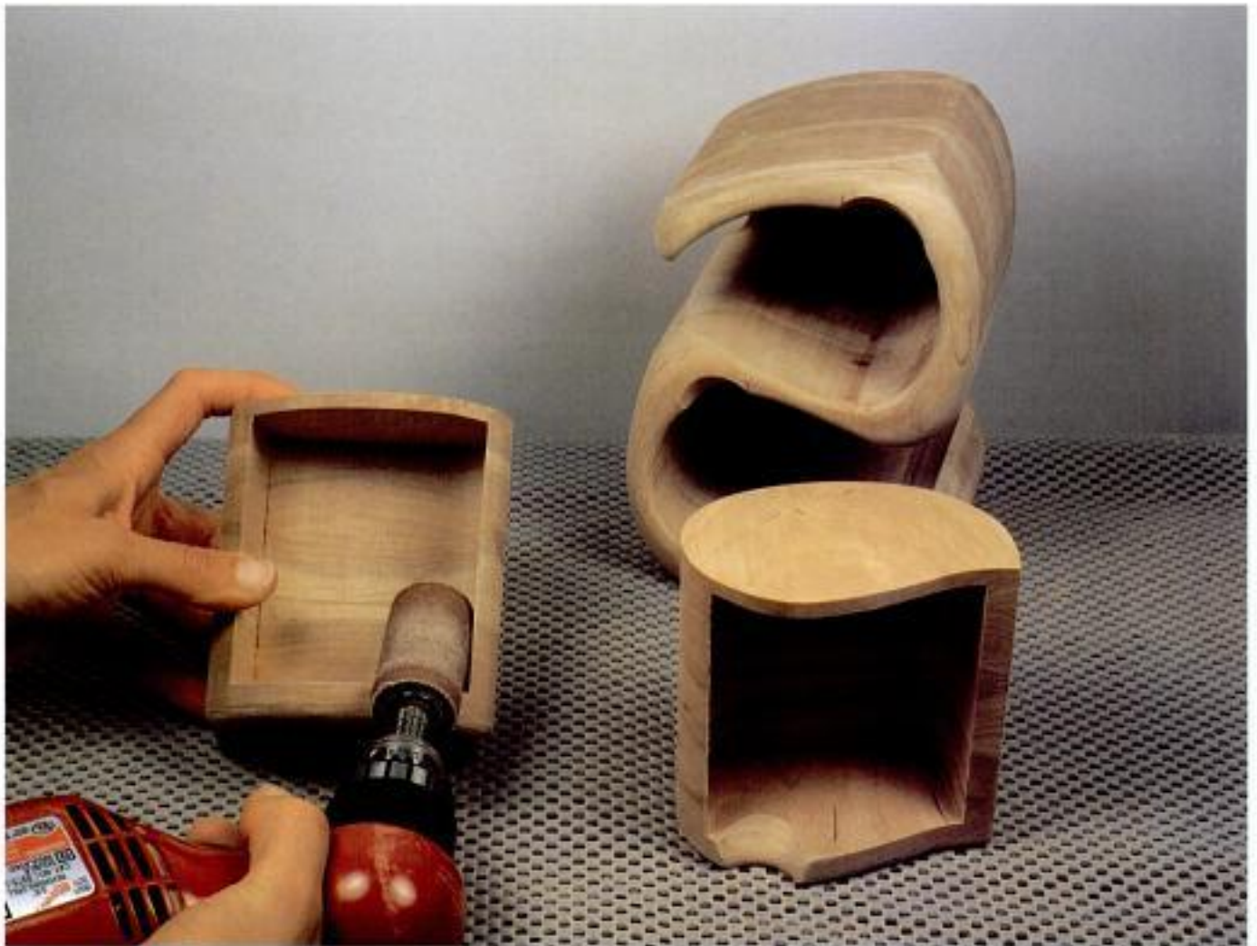
Photo 4-24 The finger slots can also be cut using the drums on your portable drill. If you roughed the slots on the oscillator, you will still have to refine the slot shape with the portable drill since it allows you more control and range of motion.
