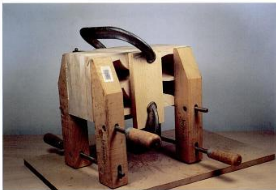
Photo 3-15 When clamping the thin back to the body, use a couple scrap blocks to ensure even contact with all box edges.
