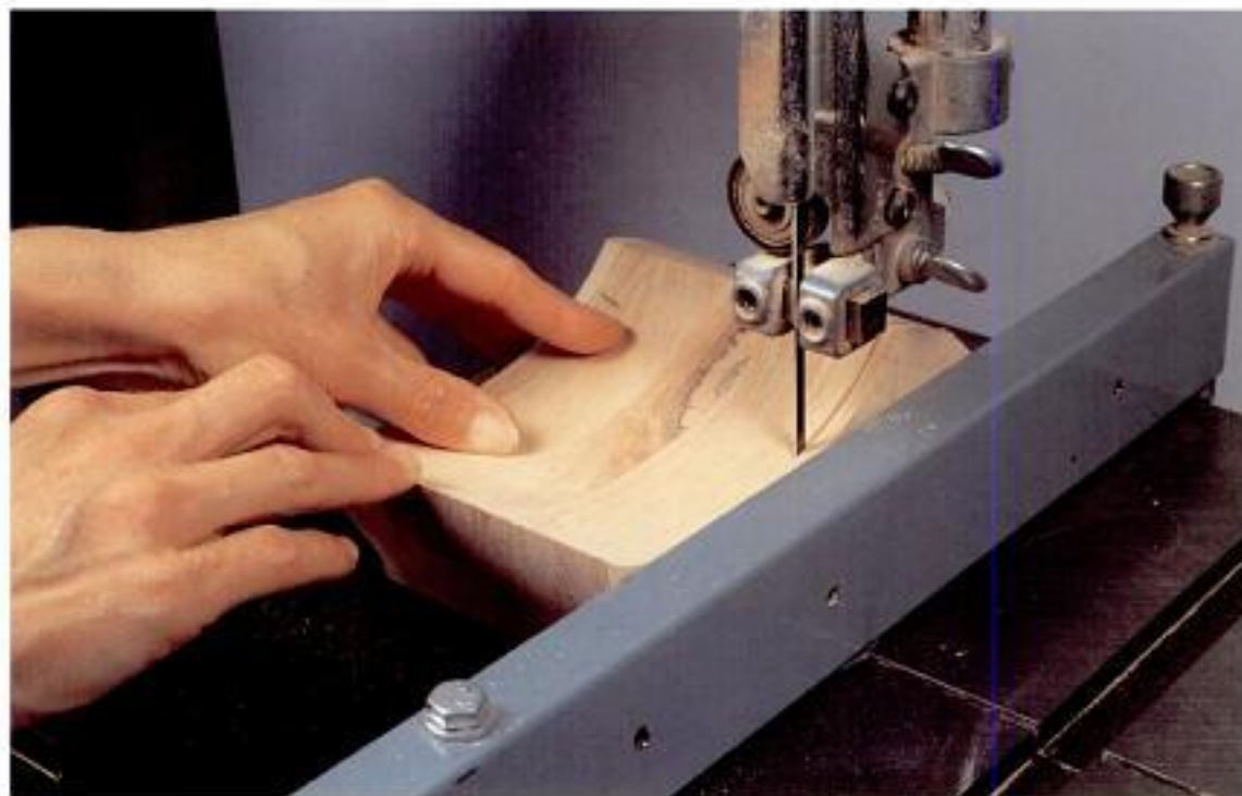
Photo 3-9 Rip \frac{1}{8} " (6mm) off the backs of the drawer blocks. When finished with all the blocks, reset the fence to \frac{1}{8} " (1.3cm) and rip the drawer fronts off.
