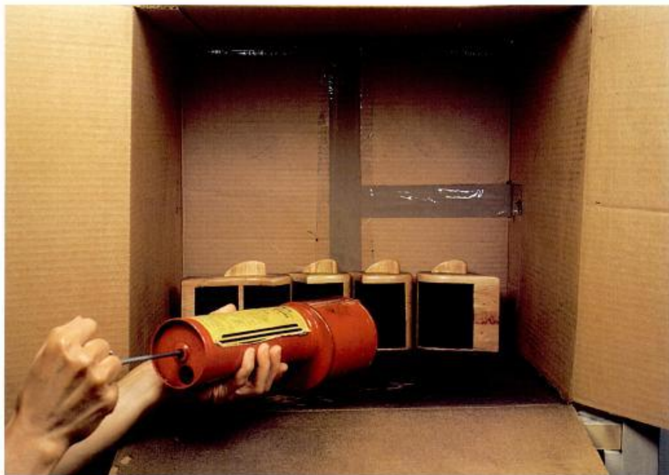
Photo 5-4 A large box can serve as a spray booth when applying flocking to the drawers.
