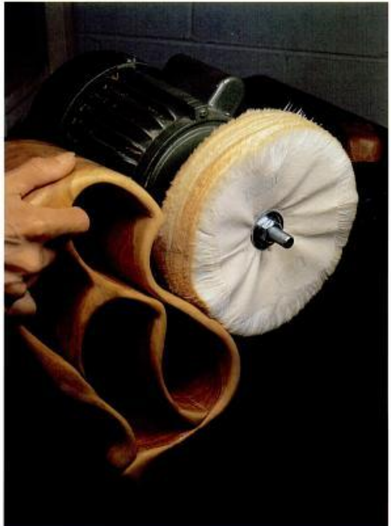
Photo 5-3 A buffing wheel with a fine abrasive can add extra burnish to an oil finish quickly and easily.
