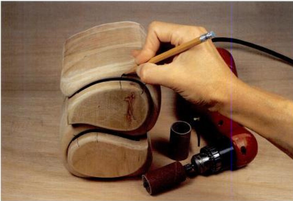
Photo 4-22 When you mark the finger-slot positions for the Cobra and Box designs, make sure you won't be cutting into the side of the drawer.
