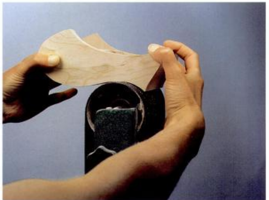
Photo 4-8 Sand the drawers carefully and thoroughly, but don't remove too much wood.
