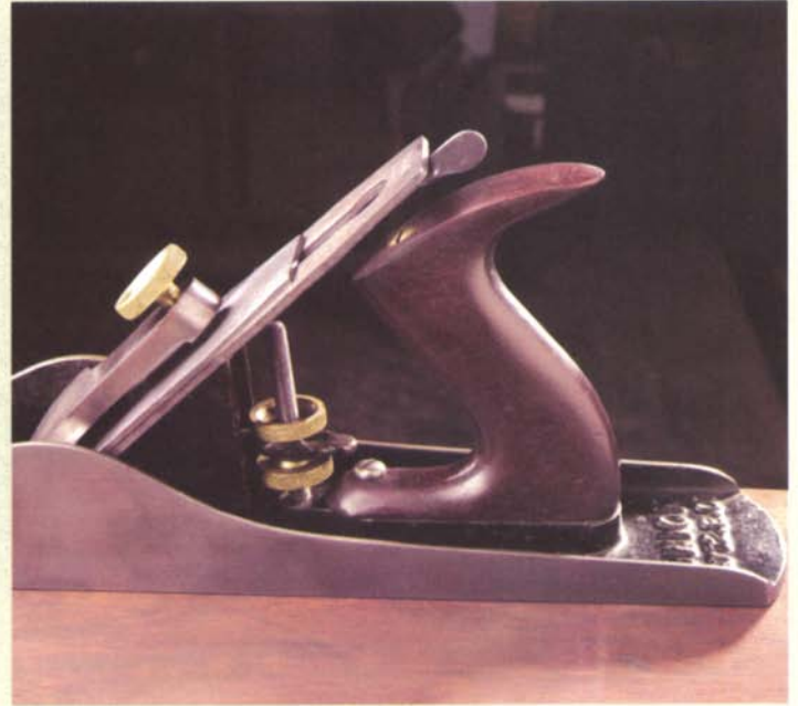
Union Tool's vertical post adjuster is somewhat slower to adjust than a Bailey plane adjuster, but it is extremely positive.
