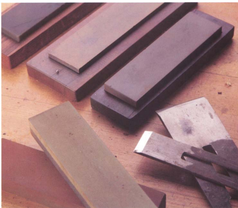
Effective sharpening demands using a variety of stones, such as (clockwise from top) a hard black Arkansas finishing stone, a medium and fine India, and two-sided water stones. A box keeps each stone protected and holds the stone in place while sharpening.
