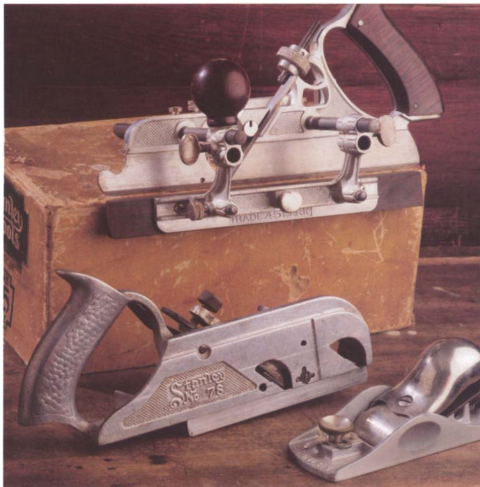
Stanley experimented with aluminum for only a few years, making planes of this material quite unusual and uncommon. Shown here are a Stanley #45, #78, and block plane.
