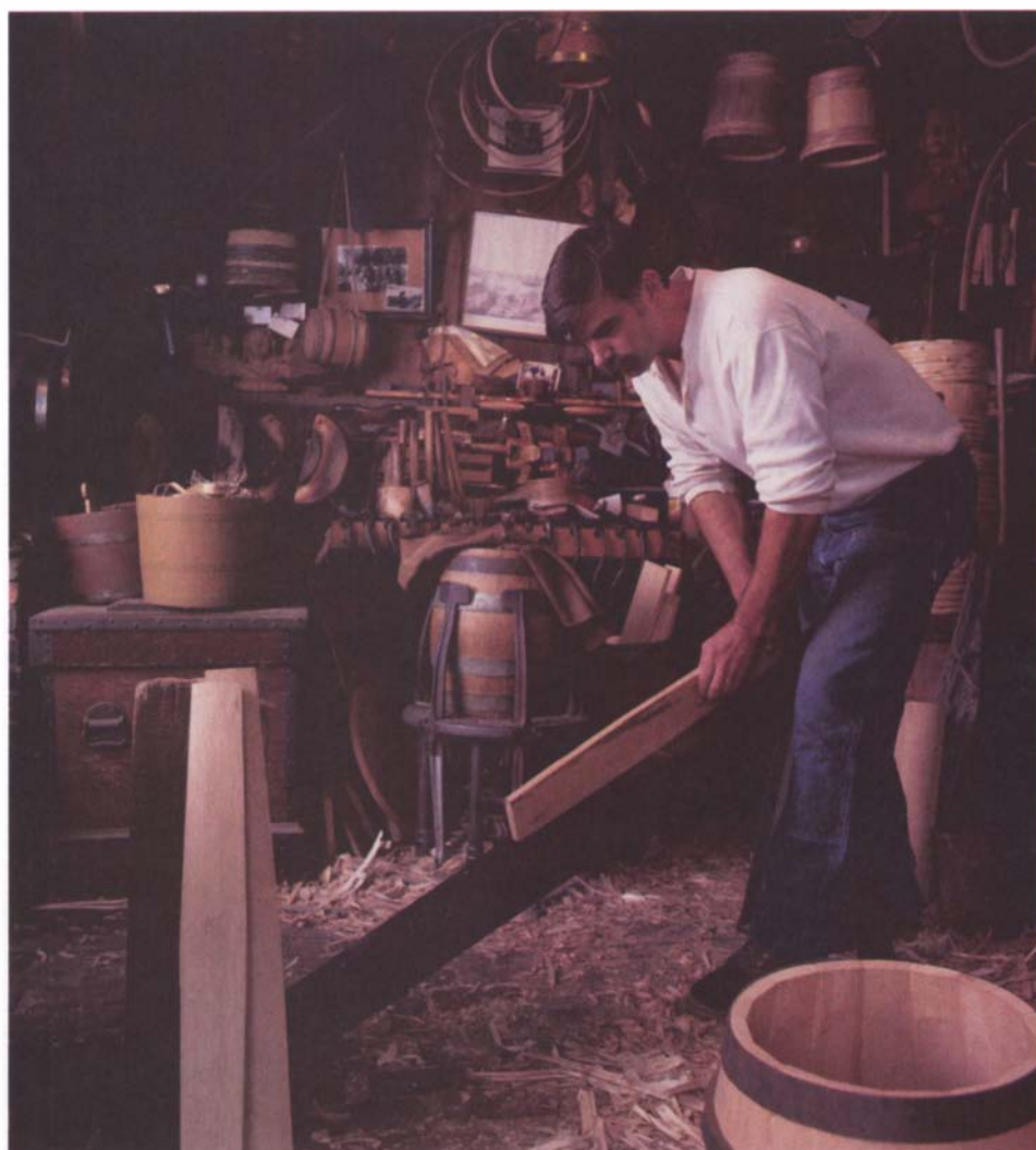
Ron Raiselis, the cooper at Strawberry Banke Museum in Portsmouth, New Hampshire, shapes white-oak barrel staves on a long and heavy cast-iron jointer plane. This is the way coopers have always done it, trusting their hand and eye to get the taper and bevel right.
