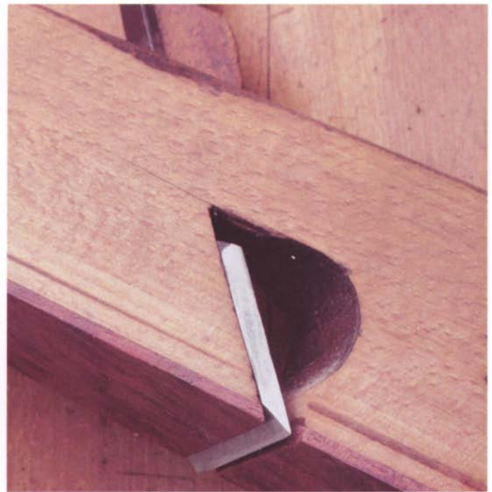
To tune a skewed rabbet iron, the back of the iron along the shoulder edge should be beveled at least as much as the skew angle.
