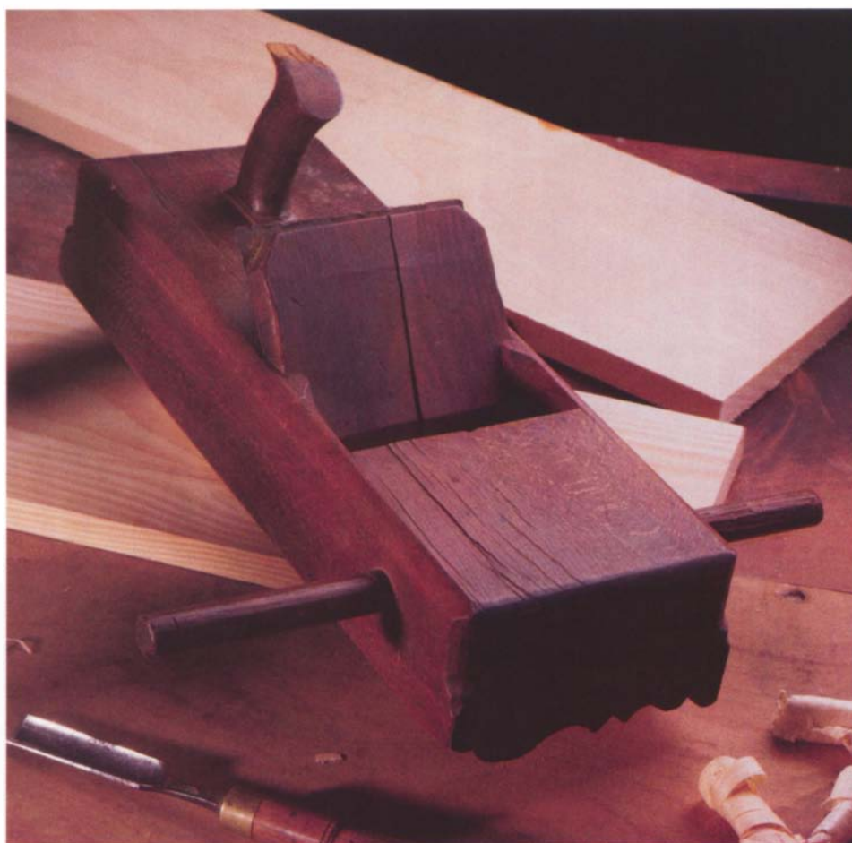
A cornice plane, with its unusually wide iron and wedge and front handles, can cut a crown molding. The alternative is to use a series of narrower planes.
