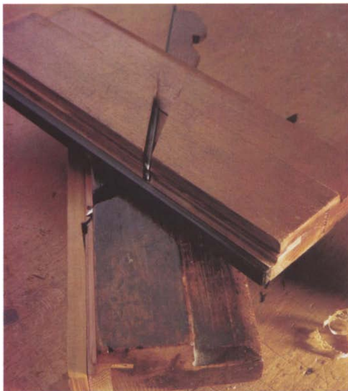
New life for two old side bead planes. The bottom one has a new sole, boxing, and fence; the top one new boxing, fence, and a profile shaped with a scratch stock. A frugal woodworker of a century ago would have readily shaped an old plane to fit his needs.
