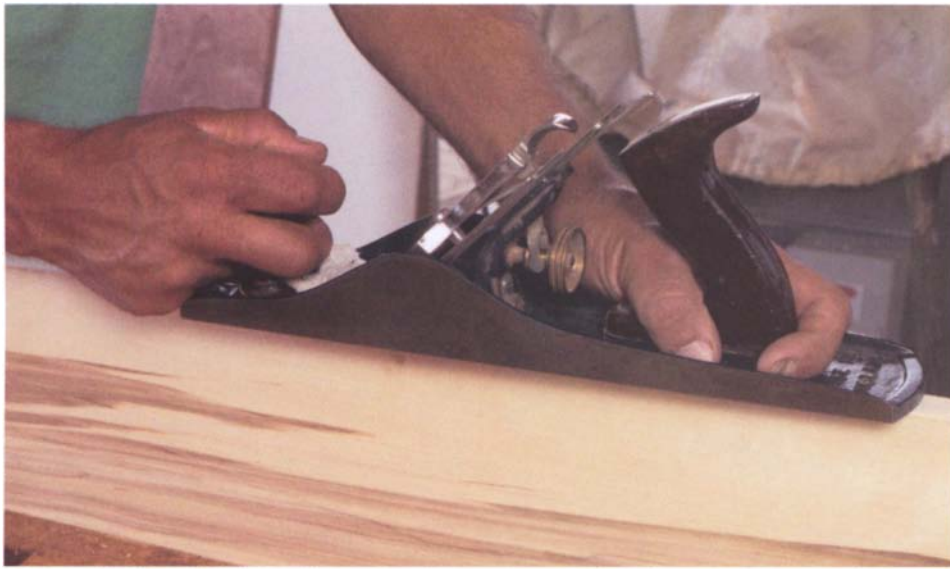
Turning the jointer around and planing backwards takes out any crown at the starting end of the board.
