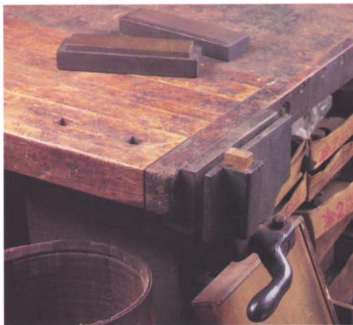
A side vise with a pop-up bench dog can serve as a versatile end vise.
