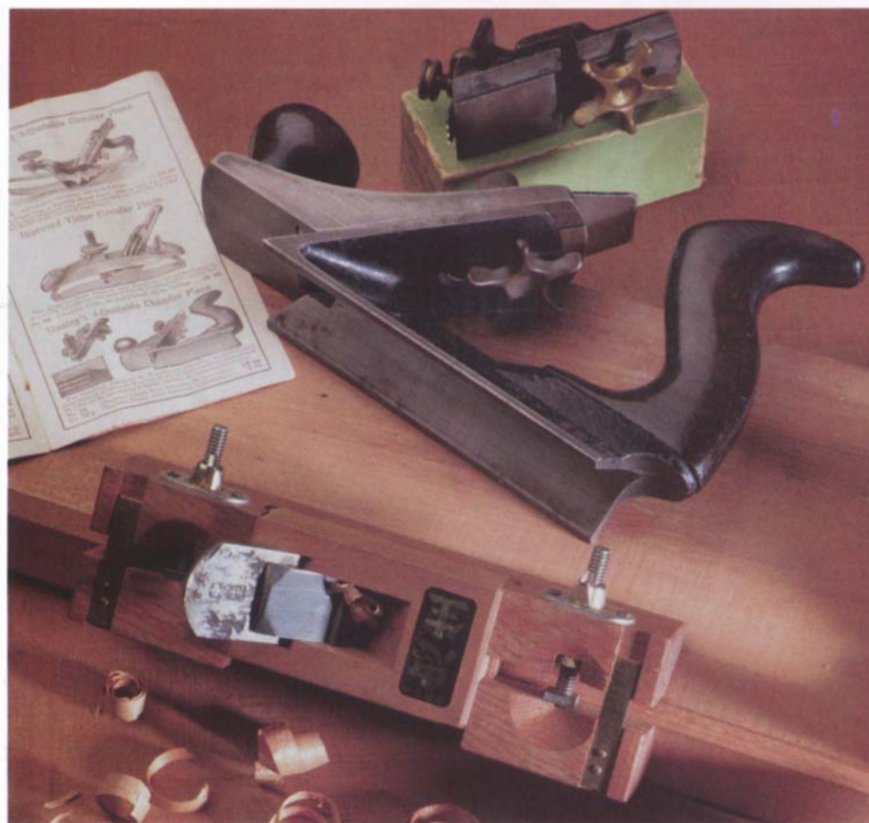
Chamfer planes have a sole in the shape of a deep right-angled “V” to guide the plane along a square edge. In the background is a Stanley #72, behind it a separate front piece that holds scratch cutters for detailing wide chamfers. The Japanese chamfer plane in the foreground has an adjustable-width sole and a sliding carriage for the iron.
