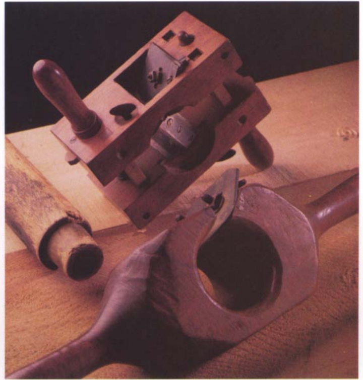
Rounder planes work on the same principle as a lathe, shaving a piece of wood round as it is fed up through the middle. The large rounder in the foreground cuts only one diameter; the more complex “witchet” at rear is adjustable and will cut tapers and tenons.
