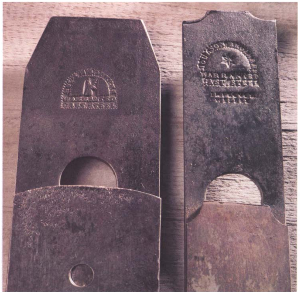
Stamping plane irons with the maker's mark was an early form of advertising. "Warranted Cast Steel," stamped on these two irons, was known for its superior quality and its ability to hold a keen edge.
