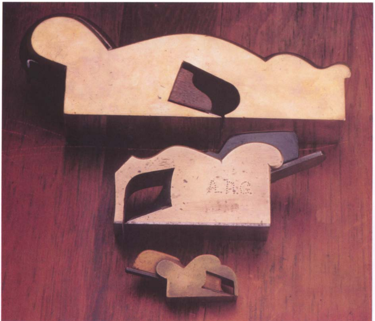
The traditional British shoulder plane at top has gunmetal sides and mahogany infill, combining beauty and adequate mass to work exceptionally well. The two smaller bullnose planes are solid metal and have shapely wedges.
