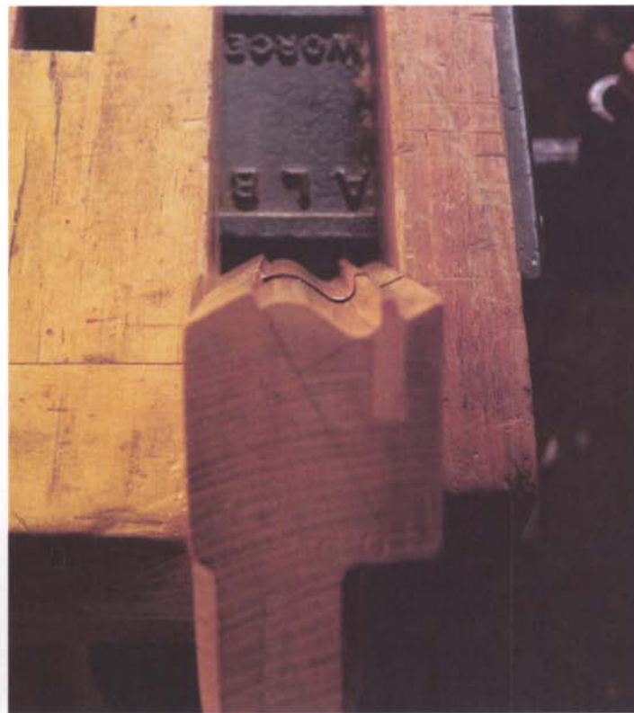
In a well-tuned plane, the iron should exactly parallel the shape of the sole (sighting down from the toe).
