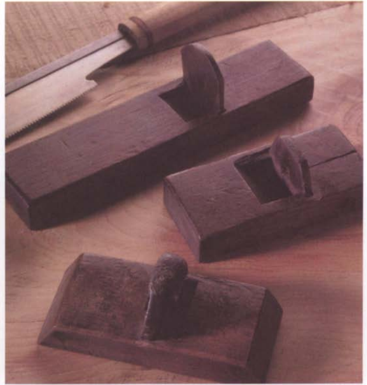
Oriental scraping planes have thick irons wedged into low hardwood bodies. The two smaller planes are used to flatten the soles of longer bench planes.
