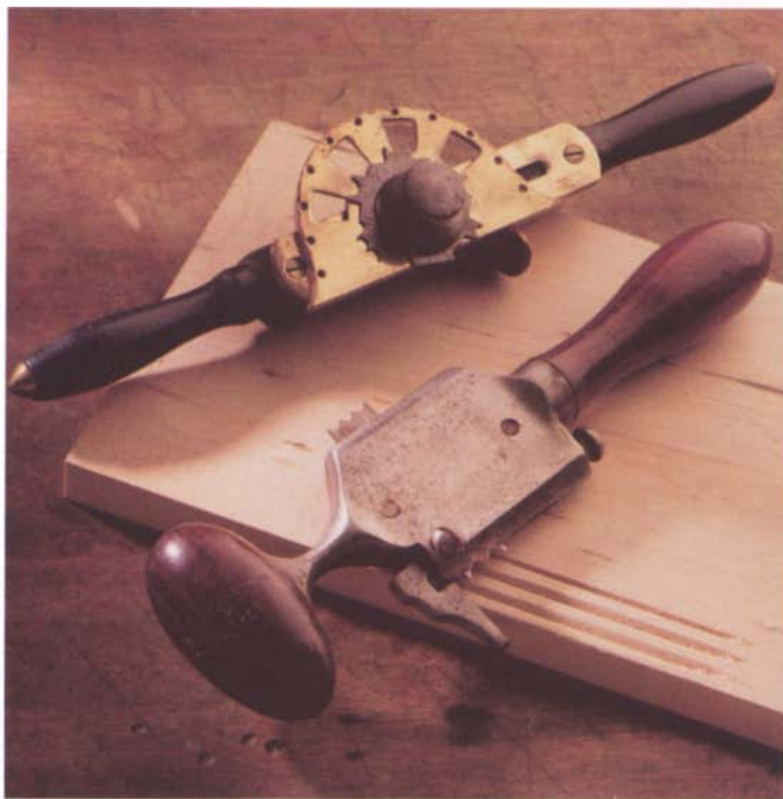
Two types of Windsor beaders. The one at rear has a cutter wheel with different cutter profiles filed into the circumference; the one in the front takes individual cutters. Both have adjustable fences.
