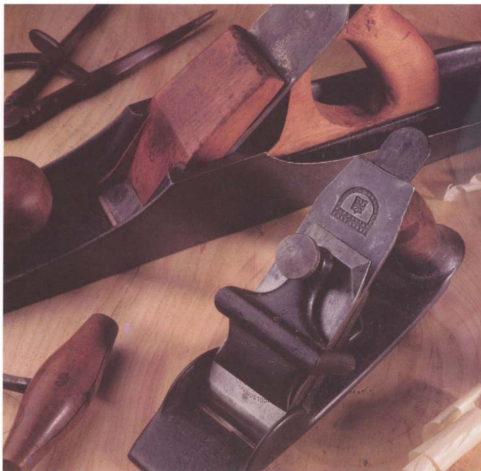
The first patented cast-iron plane, Hazard Knowles' plane of 1827 (at rear), had a frog cast integrally with the body. Another early cast-iron plane, a Birdsell Holly smoothing plane of 1852 (foreground), had a frog added to the plane and connected with the tote for better support.
