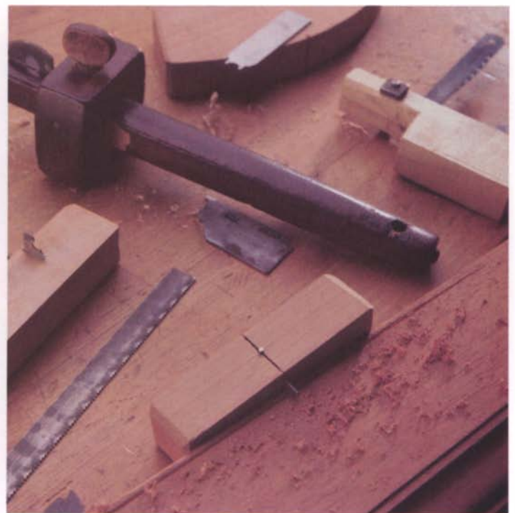
Homemade scratch stocks for cutting details such as a small bead can be as simple as a shaped piece of hacksaw driven into a saw kerf in a wooden block. An old marking gauge also works well.
