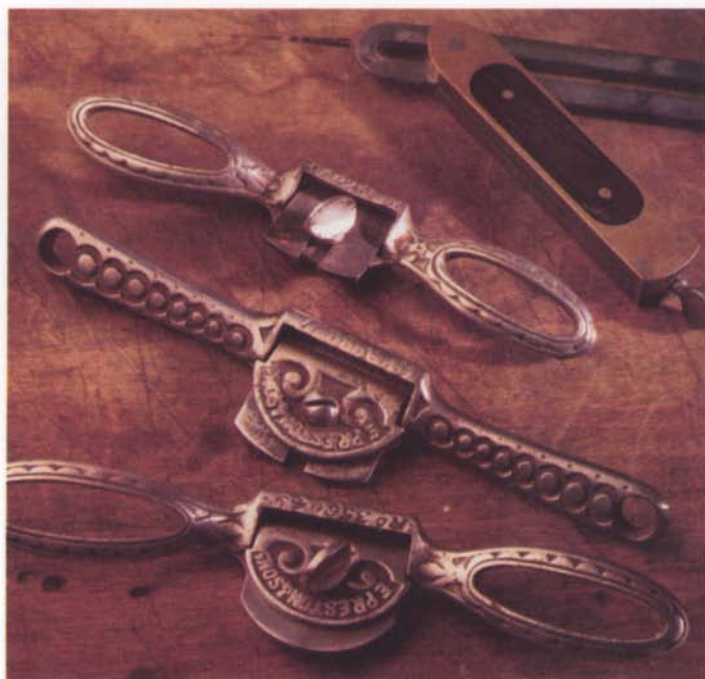
These three spokeshaves are typical of the designs by English maker E. Preston, with ornate castings and comfortable and decorative handles, and made to tight manufacturing tolerances.
