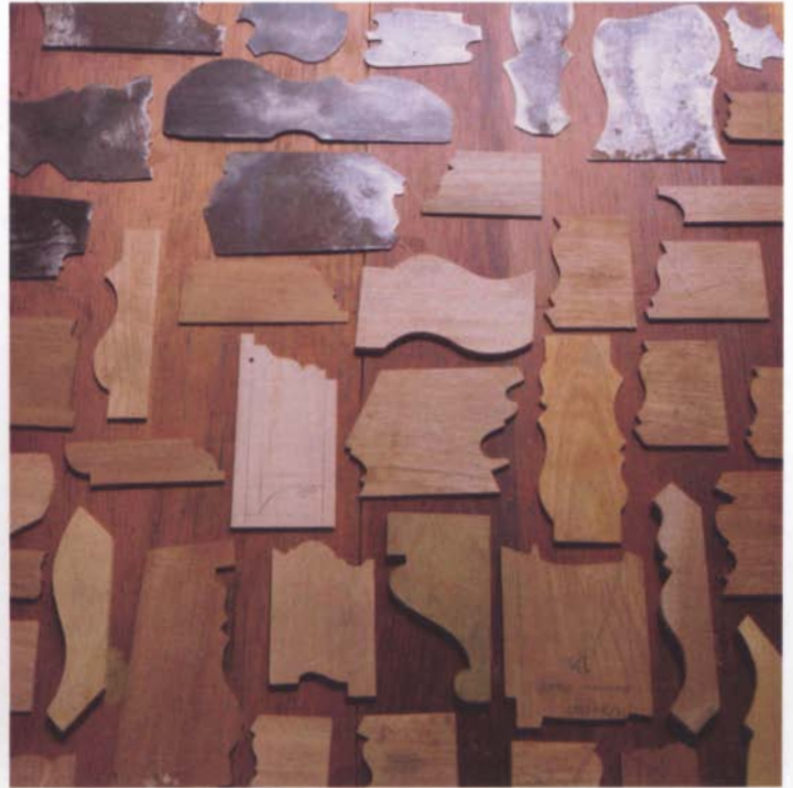
The various wooden templates shown in the foreground speed layout, while the metal scrapers at rear are used to fine-tune the sole profile after it has been shaped with other molding planes.
