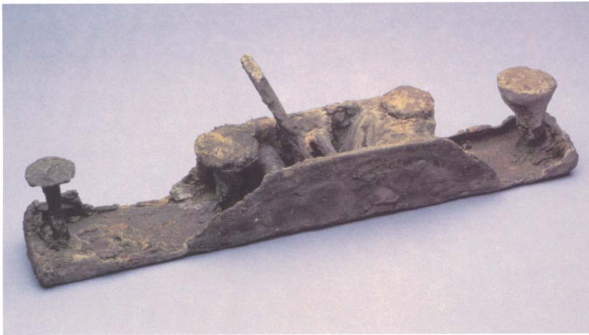
Early planes, such as this Roman carpenter's plane dating from the late 4th century, united a steel sole (and often sides) with a wooden body (which has not survived on this plane). (Photo copyright Reading Museum, Reading, England. All rights reserved.)
