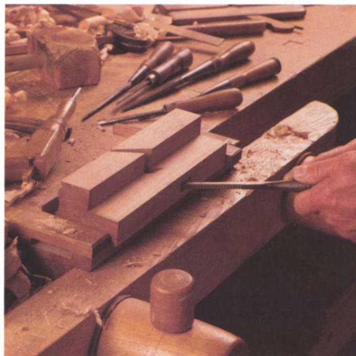
After defining the wedge mortise and then boring through to the throat, Ted uses floats and chisels to enlarge the mortise and true the bed.
