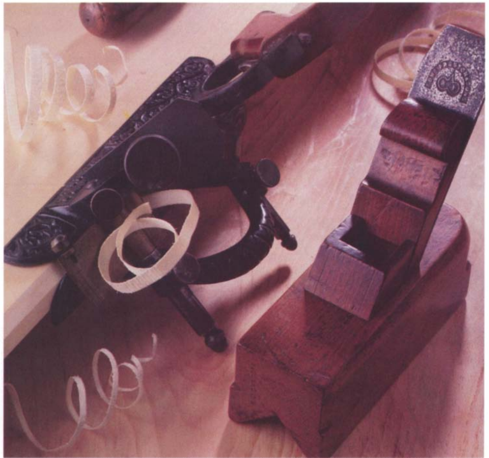
In the stop chamfer plane by Joseph Lee (1883) at left, half the sole slides open or closes to adjust the width of the chamfer. In the E. Preston chamfer plane at right, the whole center section of sole, iron, wedge, and throat moves to cut wide or narrow chamfers.
