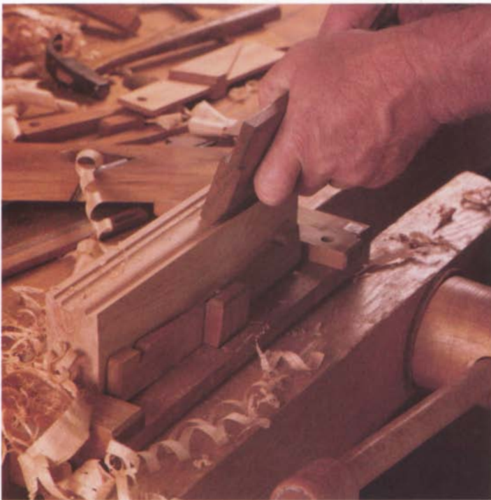
Ted shapes the sole profile to the layout lines with hollows and rounds.
