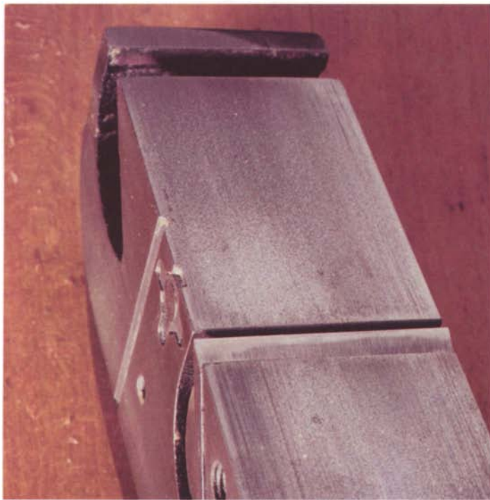
To tune a rabbet plane, here a #78 fillister, adjust the iron so that it is parallel with the sole and just proud of the side.
