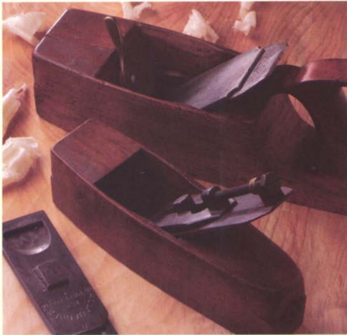
Early adjusters for wooden planes look awkward to modern eyes. Shown here are Gladwin's 1858 patent smoothing plane (at rear), which has a brass lever cam that locks and unlocks the double iron, and Worrall's patent block plane, which adjusts with a screw at the heel of the plane.
