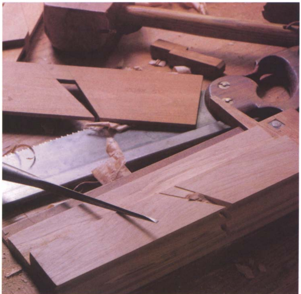
The mouth and throat of the plane are cut with a fine backsaw and then chopped out with a chisel. The pitchboard in the background is for laying out the throat opening.
