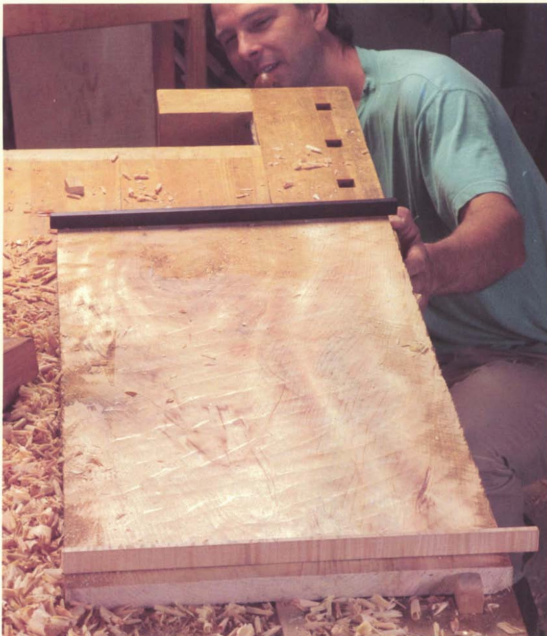
Sighting across the top edges of a pair of winding sticks reveals any twist or winding in a roughly flattened panel.
