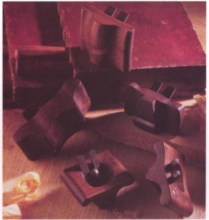
Short-sole molding planes shape the curved sections of the handrail. No matter how many shapes stairmakers owned, for some stairs they had to make special planes.
