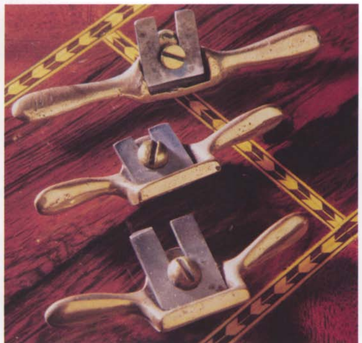
Tiny patternmaker's or modelmaker's spokeshaves cast in brass are useful for fine work. With three different sole shapes—flat, concave, and convex—this set can cut a variety of shapes.
