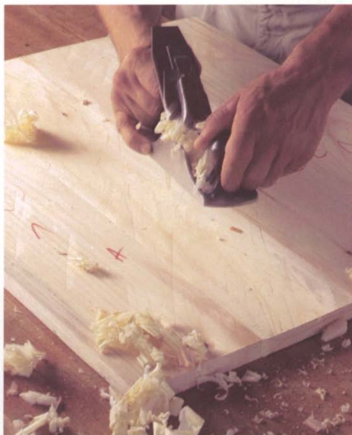
Surface a glued-up panel by flattening out the transitions between pieces. Plane on the diagonal just as with a wide board.
