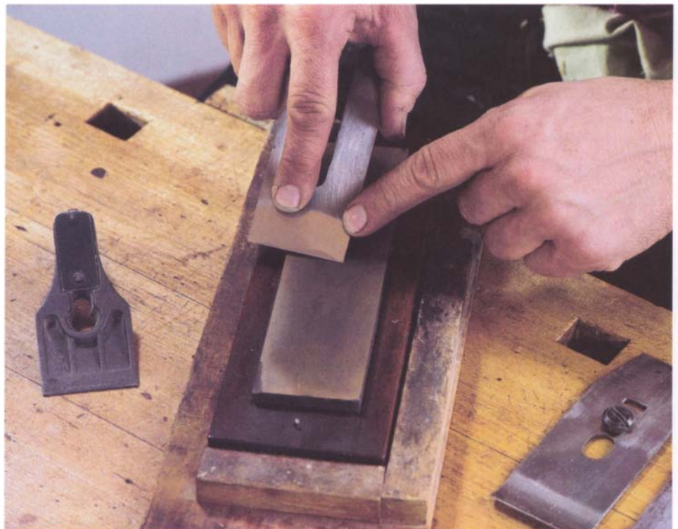
Shape the iron profile gently convex or relieve the corners on a benchstone after grinding the iron. Start with a coarse stone and use light pressure to prevent gouging the stone.
