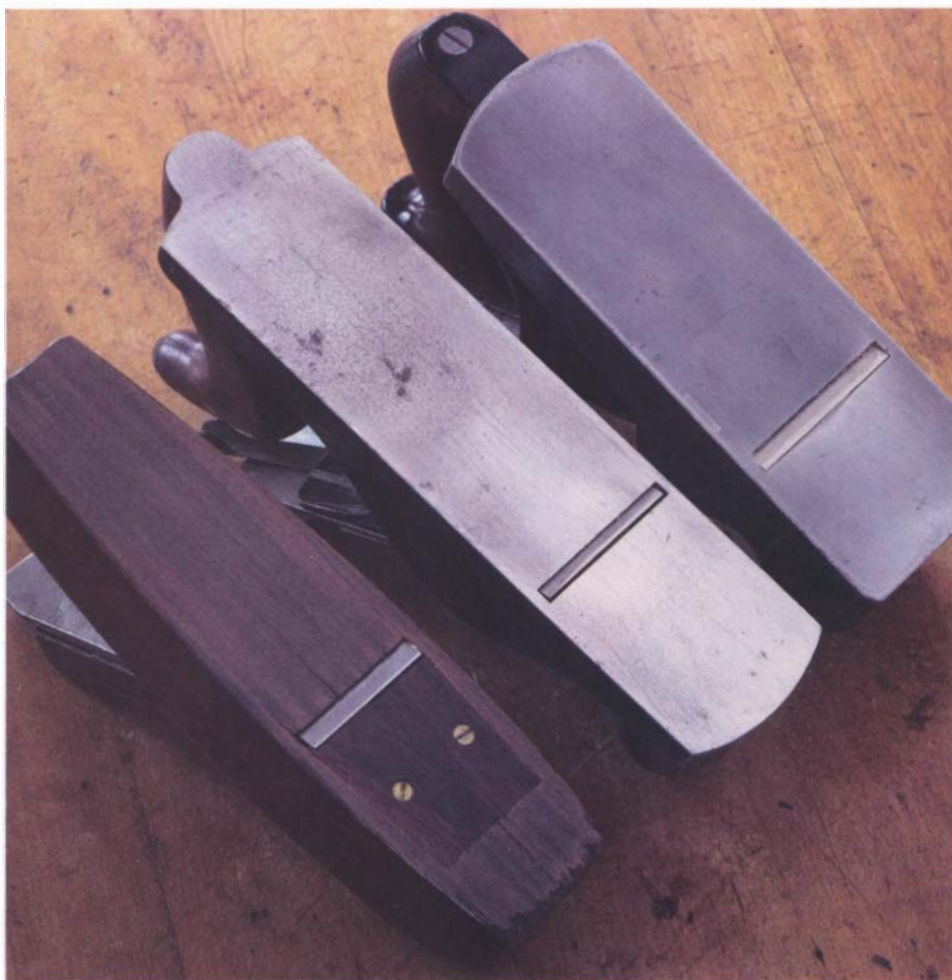
These three planes tuned for smoothing have flat soles and throats to suit the work. The lignum-vitae smoother with an added throat plate (left) and the #4 (center) have medium throats for preliminary smoothing and general bench work. The Norris at right has a very narrow throat for the finest smoothing cuts.
