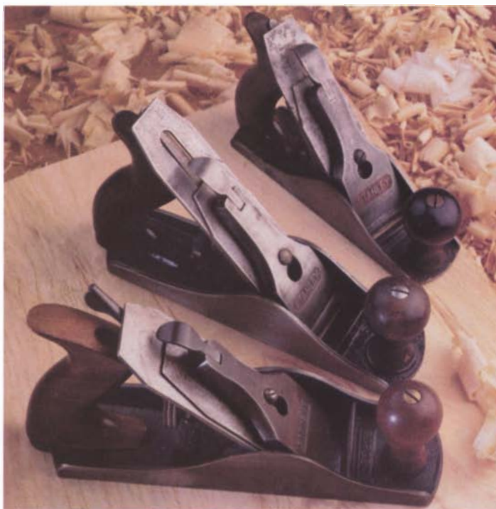
Common bench planes such as the #2, #3, and #4 shown here (from rear) have identical adjusters, rear handles, lever caps, and body shaping.
