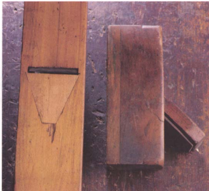
Flatten the sole of a wooden plane against a long jointer held upside-down in a vise.
