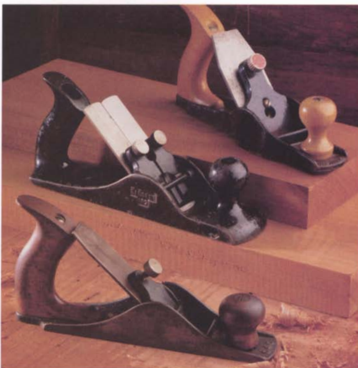
Scrub planes are the hardest-working bench planes. Shown here (from rear) are a Stanley #340 furring plane with minimal sole for "cleaning" rough boards; a Sargent #162 with two irons and cast-iron handles for a sure grip; and Ohio Tool's #040, which is nearly identical to a Stanley #40.
