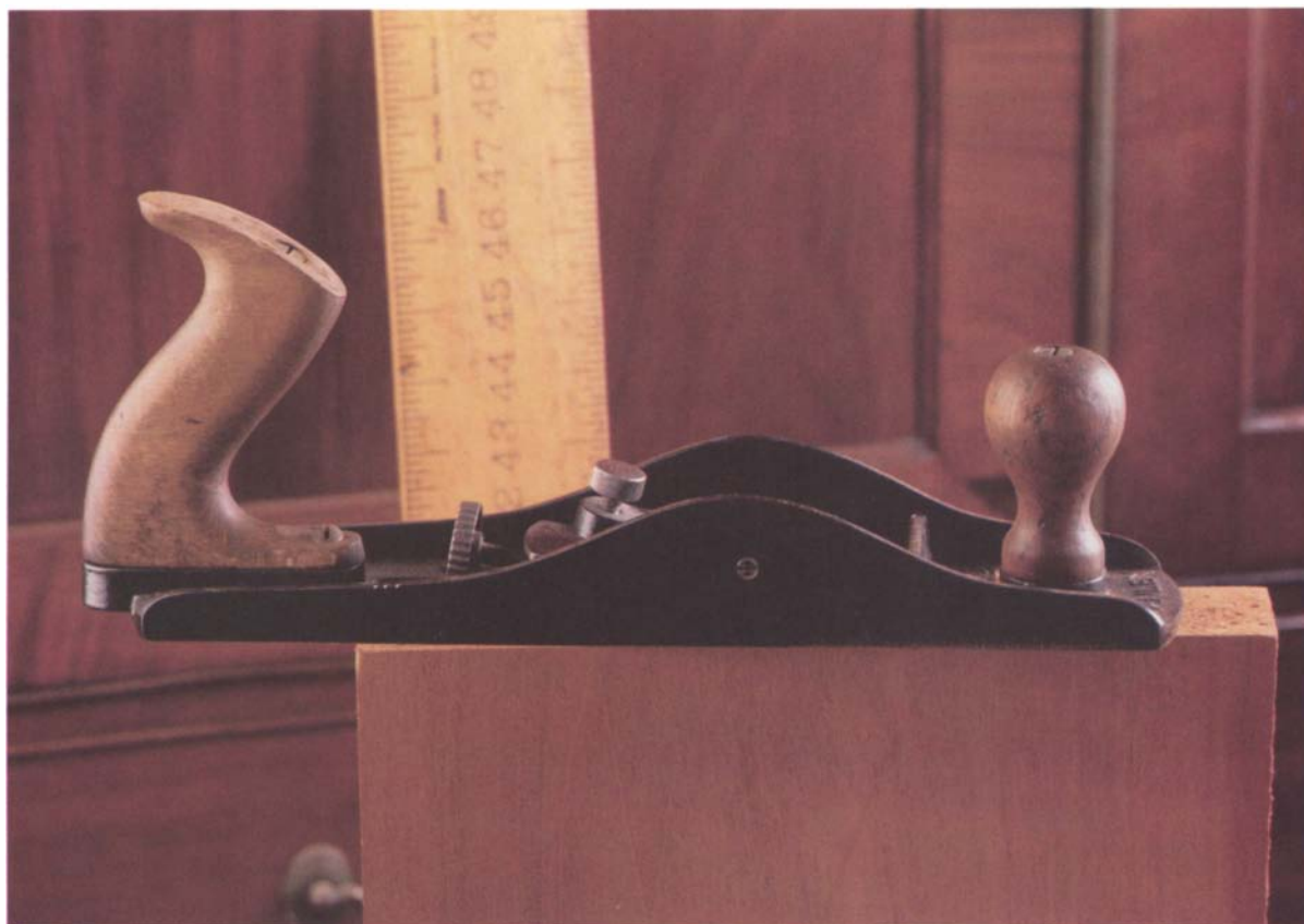
The Stanley #64 low-angle jack plane shown at left was designed for truing butcher blocks. The #62, a similar plane for furniture makers, is slightly shorter with an adjustable throat and rose-wood handles.
