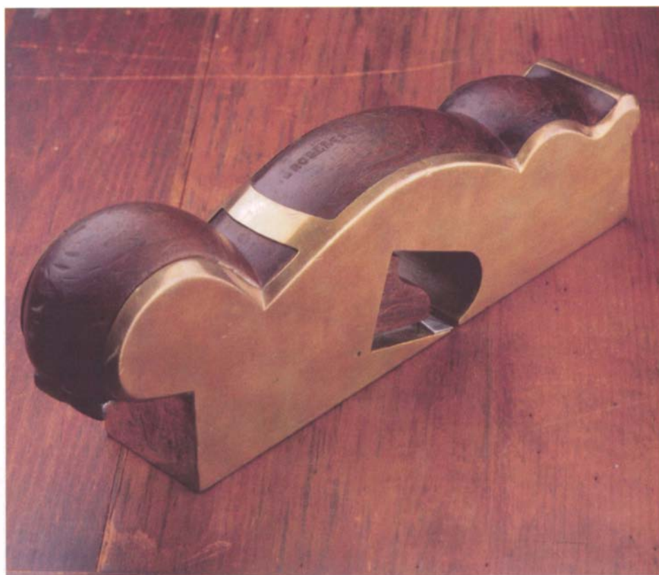
This beautiful English shoulder plane has a gunmetal body infilled with mahogany, which adds mass to the plane for superior performance.
