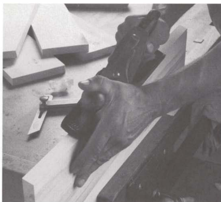
You can joint a bevel freehand by using your outstretched hand to steady and orient the plane.
