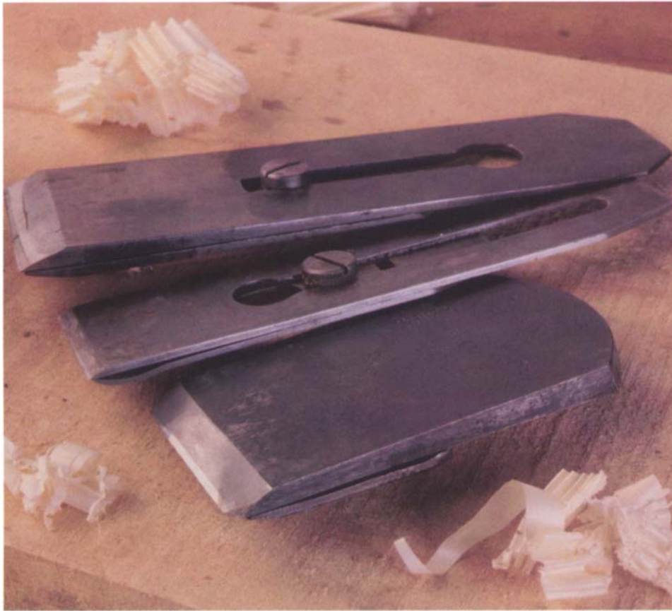
A Japanese laminated iron and cap iron (bottom) is considerably more massive than the standard Stanley thin iron (center) and the thicker iron typical of old wooden bench planes (top).
