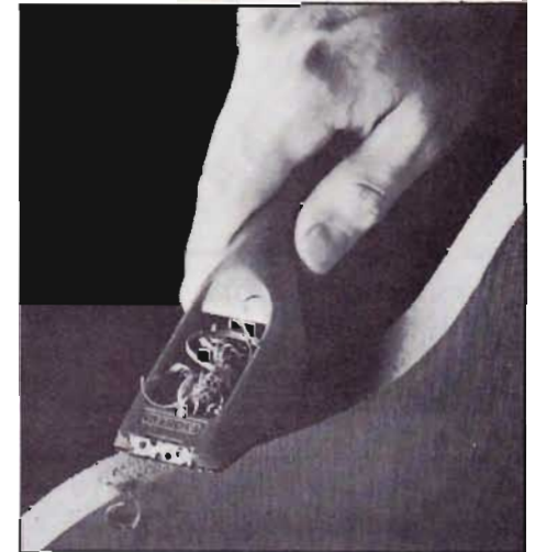
SHAVERS cut on the pull stroke and are designed for one-hand operation. When needed, it is all right to apply pressure on the toe with your free hand.
