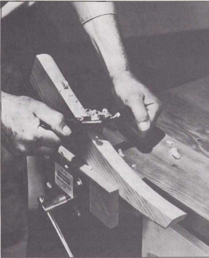
Grip the SPOKESHAVE with both hands and exert force both downward and in the direction of the pass. Hold the tool at a different angle for each pass when you are forming a contour.
