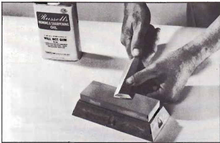
True the flat face of the blade on the fine side of the stone. Keep the blade flat and move it in a small circle.
