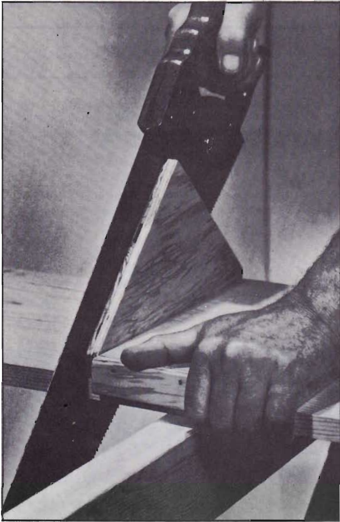
In constructing this guide, be sure the nails on the side facing the saw blade are sunk below the surface of the wood.
