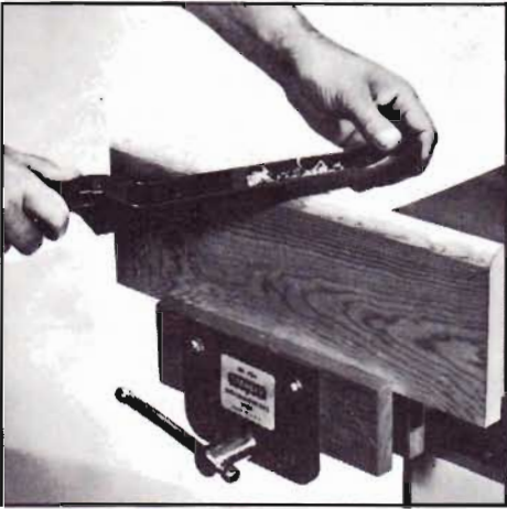
SURFORM® TOOLS cut like a horde of tiny planes, each cutting edge shaving and clearing its own path. Replacement blades are available for most designs. Work at an angle to remove stock quickly, then gradually bring the tool in line for finishing.
