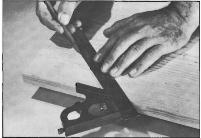
Combination squares can be used to mark lines at a 45-degree angle or to check 45-degree cuts.
