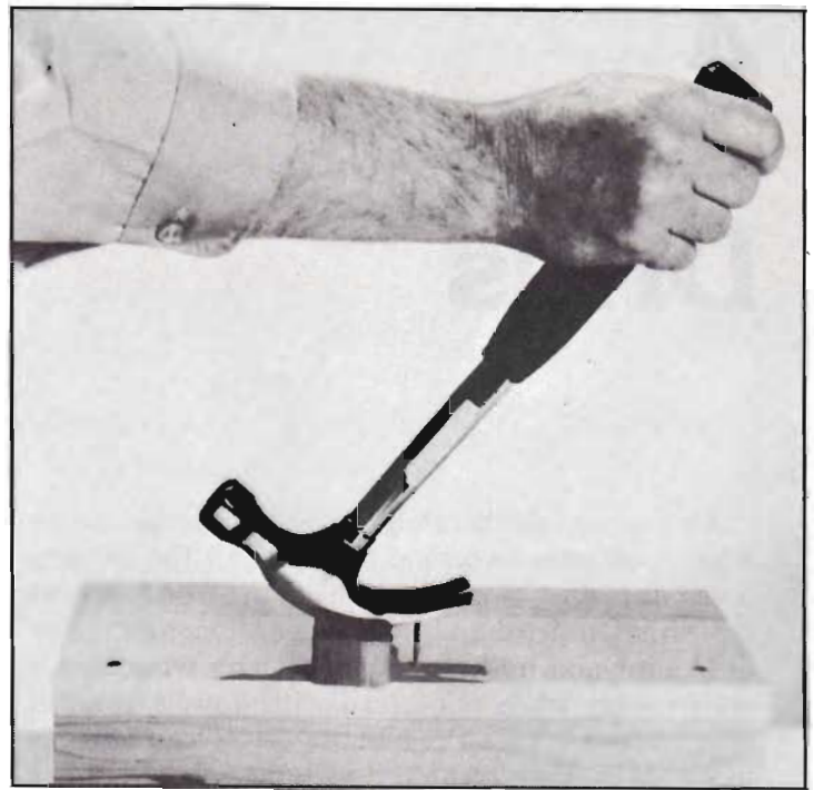
A block of scrap wood placed under the hammerhead increases leverage tremendously. The nail is removed easily and the hammer is protected from undue stress.
