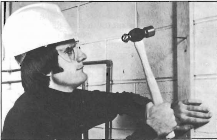
Use a heavy ball-peen hammer for driving special hardened nails into masonry. Note the hard hat and the safety goggles. Hand Tools Institute Photo.
