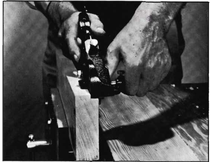
Set your RABBET PLANE to the proper depth and width for an L-shaped cut. Be sure to make all passes with the fence snug against the side of the work.
