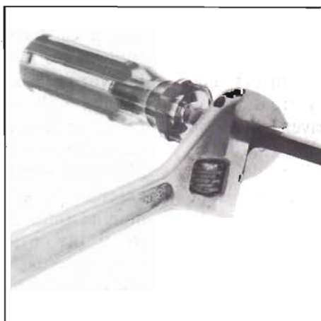
A wrench may be used on a square-shank screwdriver to apply more force to the screw. Care should be taken not to apply too much force or the screw might break.
