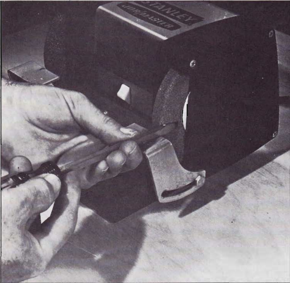
Use a BENCH GRINDER with care. Wheel guard on this machine was removed for the photograph. Always work with the guards in place, and always wear safety goggles.
