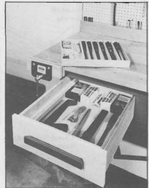
Left drawer holds chisels, shaping tools and miscellaneous tools like tapes and knives. The partitioned sliding tray keeps chisels apart.
