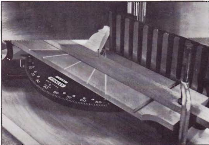
Compound-angle cuts are easy, even on coved molding, if you brace the work. The cut is then made as if it were a simple 45-degree miter.
