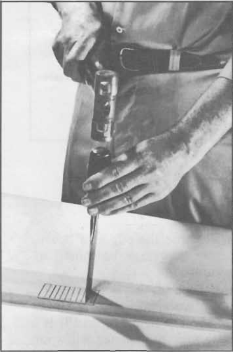
Another way to make a MORTISE is to make a series of perpendicular cuts and then clean out the waste. Many people find this method more accurate. Pencil line on edge shows the mortise depth.
