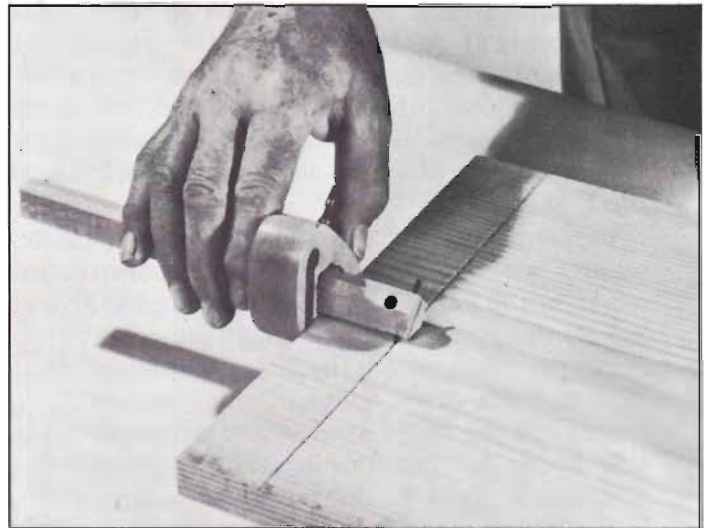
Work gently with the gauge riding on one of the flat faces of the beam. The point projects just enough to mark the work. A piece of lead can be used in place of the metal point.
