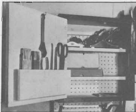
Left cabinet holds planes. Small blocks are installed on the shelves to elevate the planes and protect their cutting edges.
