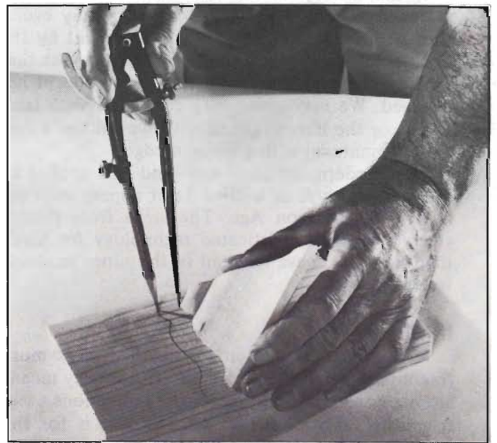
DIVIDERS or a COMPASS can be used to duplicate an irregular line. Keep the tool almost perpendicular and make sure both points are moving evenly.
