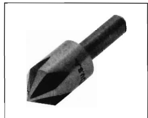
COUNTERSINK BITS , sometimes called rose head bits, are used to widen screwholes so the heads of flat-head screws will fit flush with, or slightly below the surface of the work. Properly tempered, they may be used with soft metals such as aluminum or brass.
