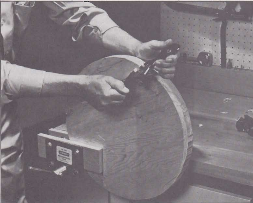
Like a block plane, a spokeshave will do a good job of chamfering or rounding edges of circular pieces. On jobs like this you can not always work with the grain, but try to as much as you can.
