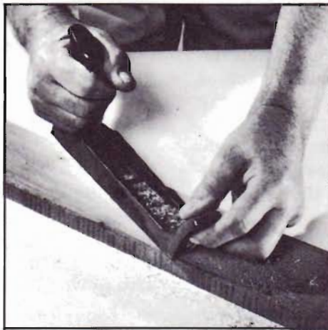
PLANE TYPE formers have handles like conventional planes. Start with oblique strokes. Keep the pressure even from heel to toe. Don't try to dig in.
