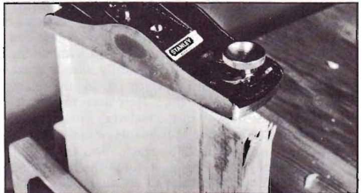
Splintering may occur at the end of end-grain cuts, even if you decrease the depth of your cut. Prevent it with the methods shown on the next page.
