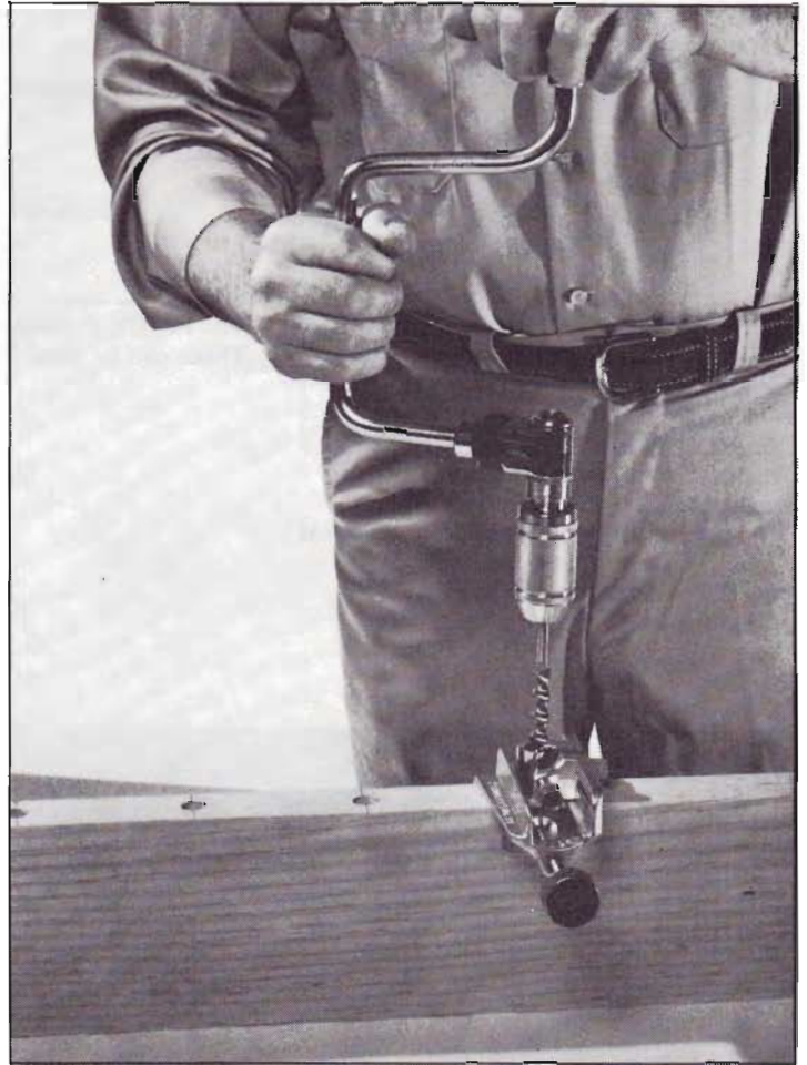
Typical doweling jigs include sleeves for various size bits and a stop to control hole depth. The jig is adjusted to center the hole in the stock, then clamped in place. The jig also guarantees the hole will be perpendicular.
