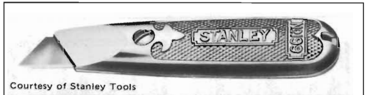
UTILITY KNIFE with fixed blade. Removing the screws allows you to change blades and provides access to spare blades stored in the handle.
