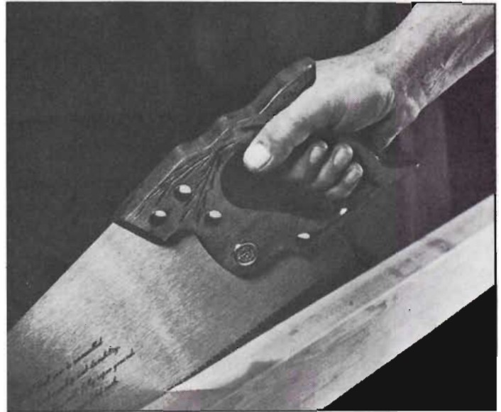
Shake hands with the handle of the saw. Be firm but don't put a strain in your hand and wrist.
