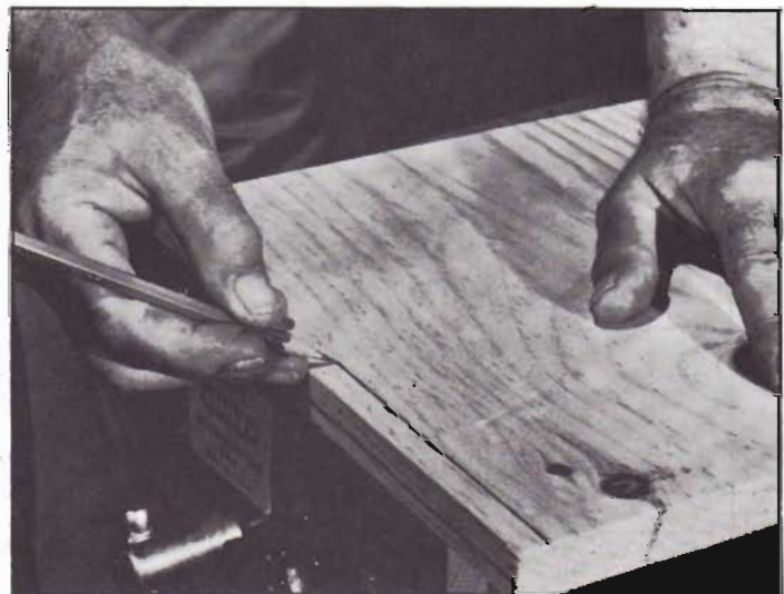
Your fingers can serve as a marking gauge when drawing lines parallel to an edge. Use one finger to ride the edge of the stock and mark by pulling the pencil.
