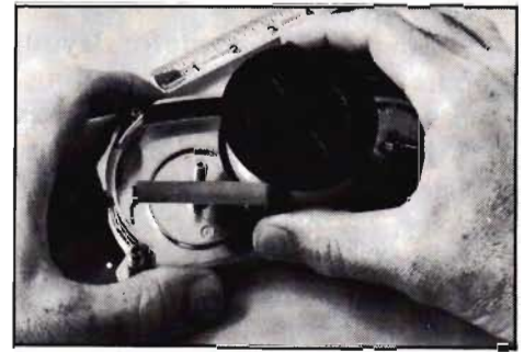
Be sure the tape you buy is replaceable. This model has a drop-in cartridge with a new blade and spring.
