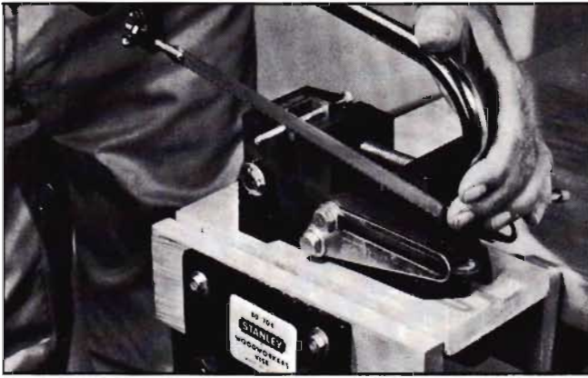
An ANGLE or DRILL-PRESS VISE is a handy accessory for gripping metal parts you wish to cut with a hacksaw. Note how this one is bolted to a board that can be gripped in a bench vise.
