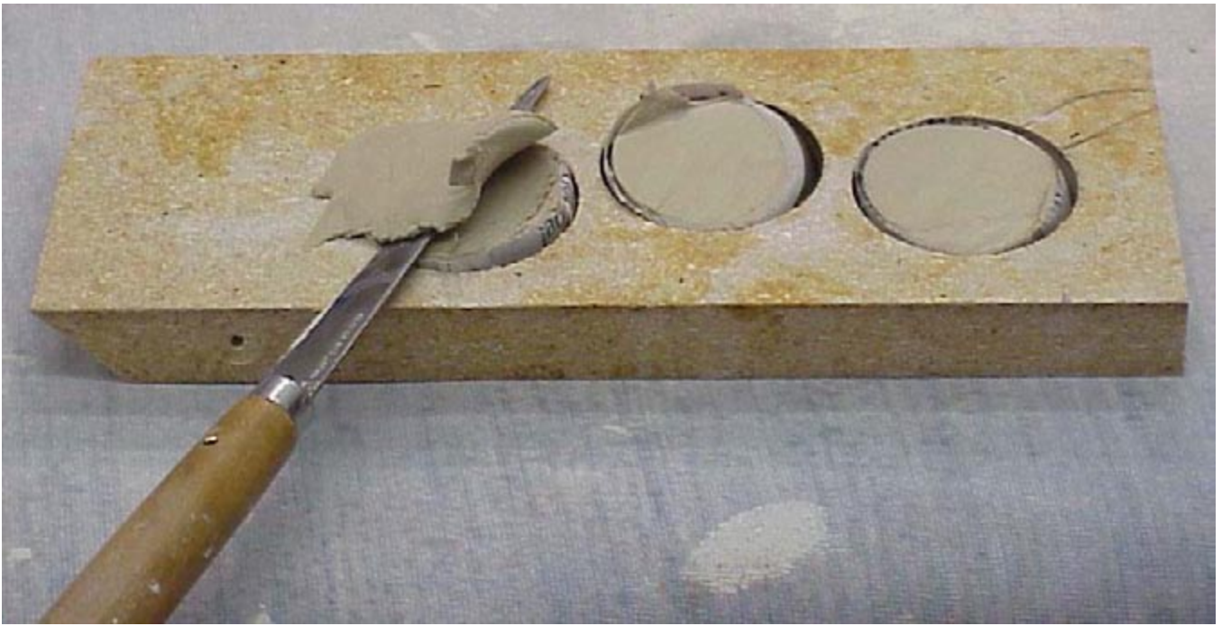
Mold Board and fettling knife - trimming the clay-filled holes flat
