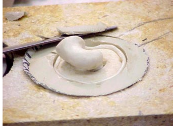
Model pressed into the clay, trimming with the fettling knife
